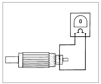
Figure 5-13. Armature Open Test
