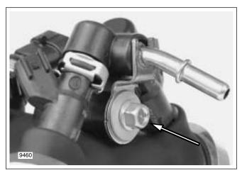
Figure 9-27. Fuel Supply Tube Clamp Hex Screw
