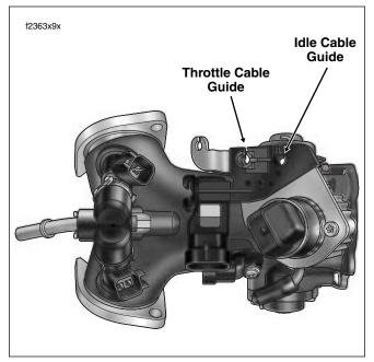
Figure 2-111. Throttle Cable Assembly - Induction Module Side
