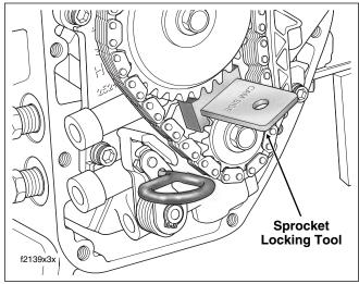
Figure 3-52. Lock Crank and Primary Cam Sprockets
