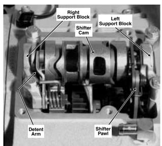
Figure 7-8. Install Shifter Forks/Shifter Cam
