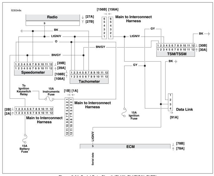
Figure 5-64. Serial Data Circuit (FLHX, FLHT/C/U, FLTR)
