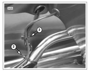
Figure 8-196. Capture CB Antenna Cable (FLHTCU)
