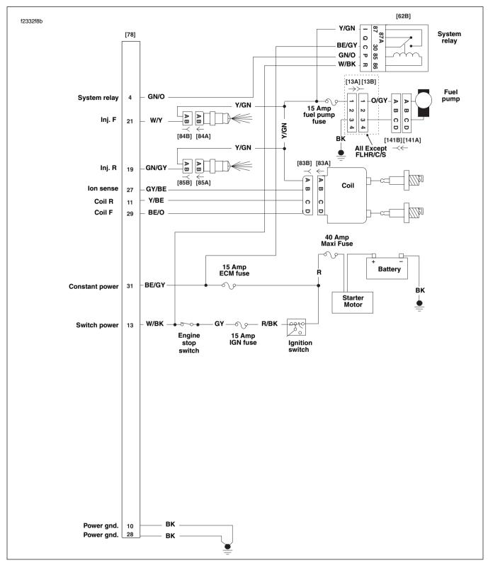
Figure 5-41. Ignition Coil Circuit
