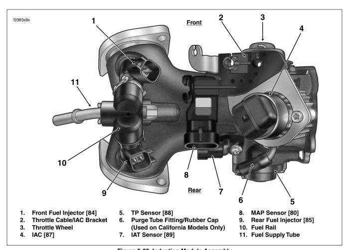
Figure 9-23. Induction Module Assembly
