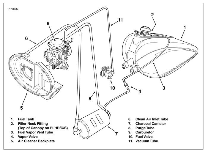
Figure 4-21. California Evaporative Emissions Control System (Carbureted Models)
