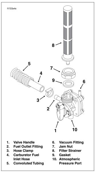
Figure 1-23. Vacuum Operated Fuel Valve
