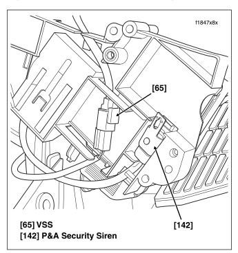
Figure 8-161. Electrical Bracket (Inboard Side)
