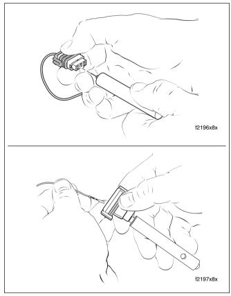
Figure 8-28. Insert Tool and Remove Terminal
