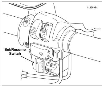
Figure 7-2. Right Handlebar Switch Assembly (FLTR, FLHTCU)
