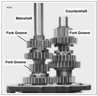
Figure 7-9. Shifter Fork Groove Locations
