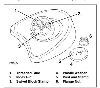
Figure 2-128. Left Side Mirror Assembly (FLHX)
