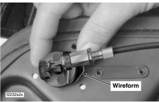
Figure 2-140. Remove Button Assembly
