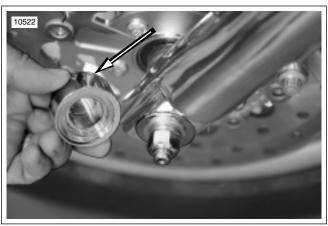
Figure 2-7. Front Axle Cover Set Screw
