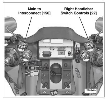
Figure 7-8. Outer Fairing Removed (FLTR)
