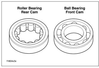
Figure 3-110. Cam Bearings
