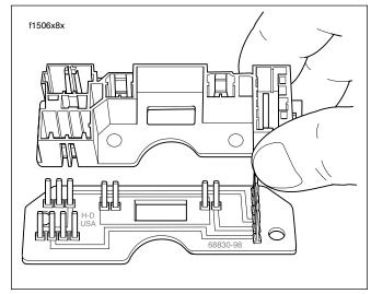
Figure 8-43. Place Pin Housing Over Circuit Board
