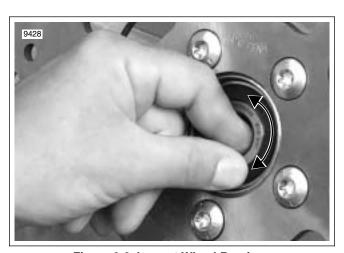
Figure 2-2. Inspect Wheel Bearings
