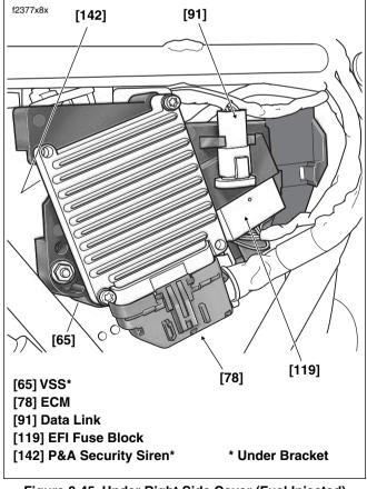
Figure 8-45. Under Right Side Cover (Fuel Injected)
