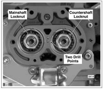
Figure D-7. Install Mainshaft/Countershaft Locknuts
