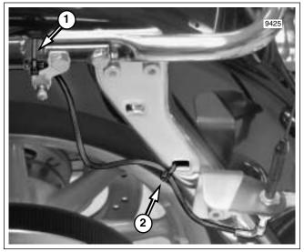
Figure 8-185. Capture Radio Antenna Cable (FLTR)
