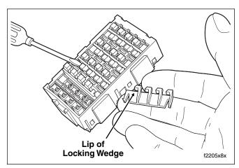
Figure B-21. Remove Secondary Locks From Fuse Block
