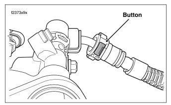
Figure 9-25. Remove Fuel Supply Line From Supply Tube
