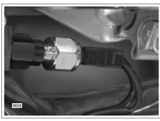
Figure 8-114. Rear Stoplight Switch
