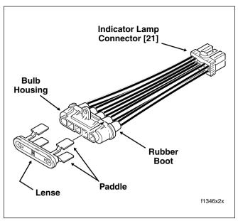
Figure 2-19. Indicator Lamp Assembly (FLHX, FLHT/C/U, FLTR)
