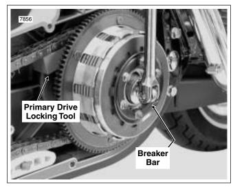
Figure 6-20. Place Primary Drive Locking Tool and Loosen Clutch Hub Mainshaft Nut
