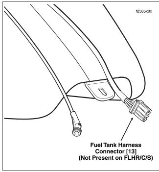
Figure B-47. Rear of Fuel Tank (Under Seat)
