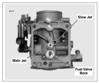
Figure 4-10. Carburetor Housing
