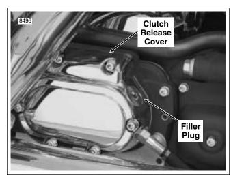
Figure 7-16. Transmission Case (Right Side)
