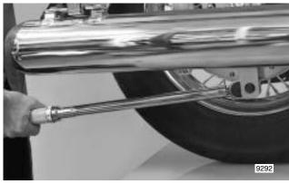
Figure 2-102. Install Tool Perpendicular to Torque Wrench
