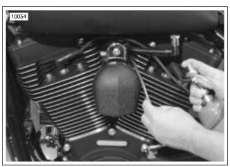
Figure 5-15. Checking for Leaks
