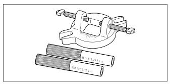
Part No. HD-95952-33B Connecting Rod Clamping Tool
