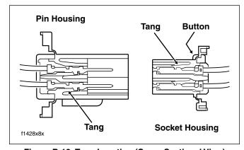
Figure B-12. Tang Location (Cross Sectional View)
