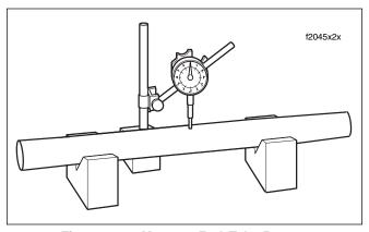
Figure 2-76. Measure Fork Tube Runout
