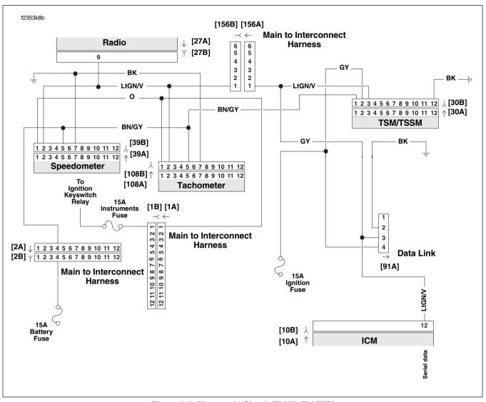
Figure 4-5. Diagnostic Check (FLHX, FLHT/C)
