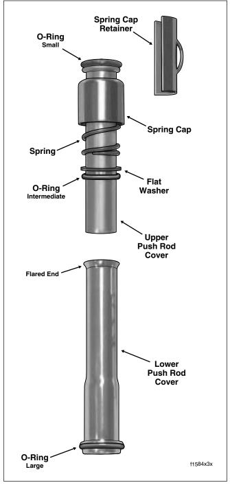
Figure 3-61. Push Rod Cover Assembly
