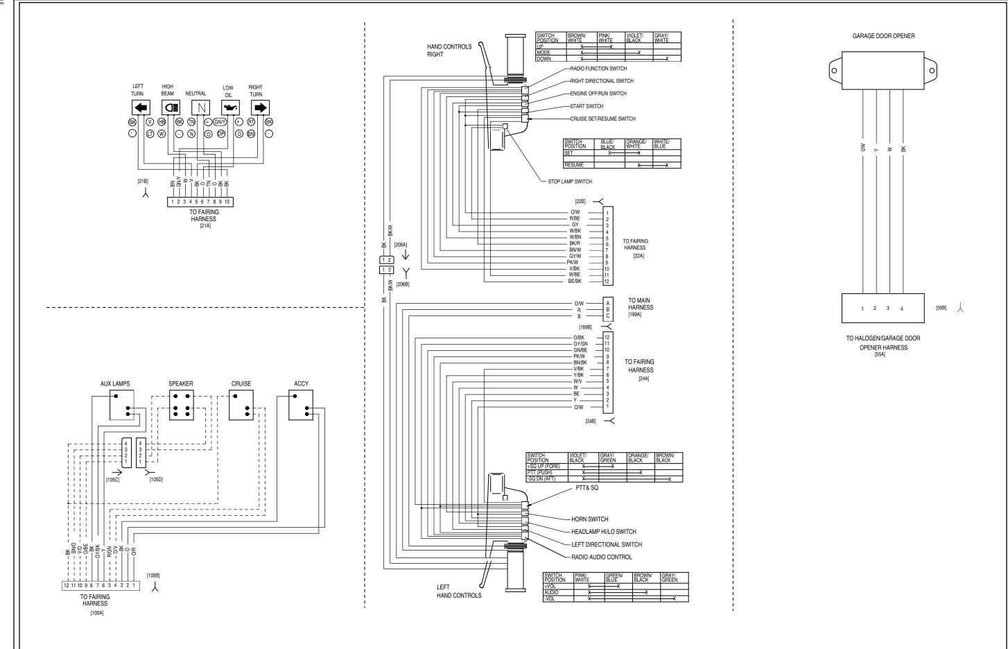
2006 FLHTCUSE DOM. and INT. MODELS, HANDLEBAR CONTROLS, INDICATOR LAMPS, FAIRING CAP SWITCHES
