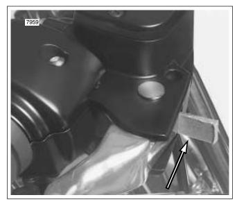
Figure 2-43. Install Cardboard Insert
