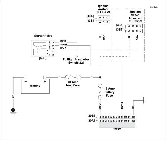
Figure 3-35. Starter/TSSM Circuit
