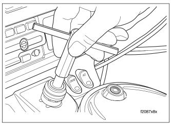
Figure 8-77. Rotate Alignment Tool Without Bottoming
