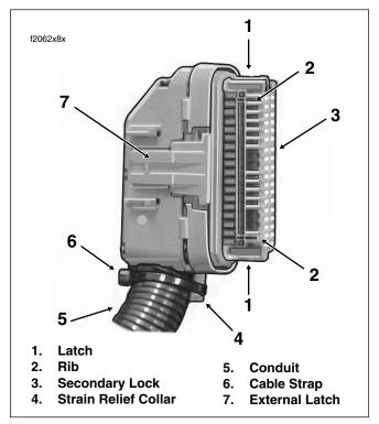
Figure B-33. Remove Secondary Lock
