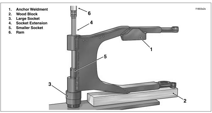
Figure 2-97. Press Out Drive Side Bearing
