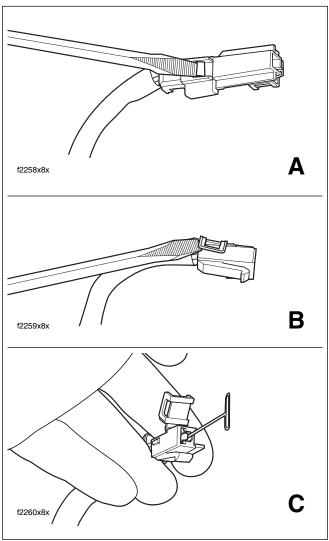
Figure B-24. Remove Socket Terminal
