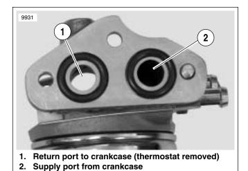
Figure 3-44. Oil Filter Mount Ports to Crankcase
