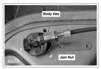
Figure 2-142. Cable Adjustment
