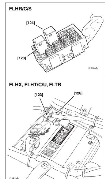
Figure 5-2. Locate Starter Relay
