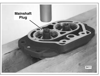
Figure D-2. Press Out Countershaft
