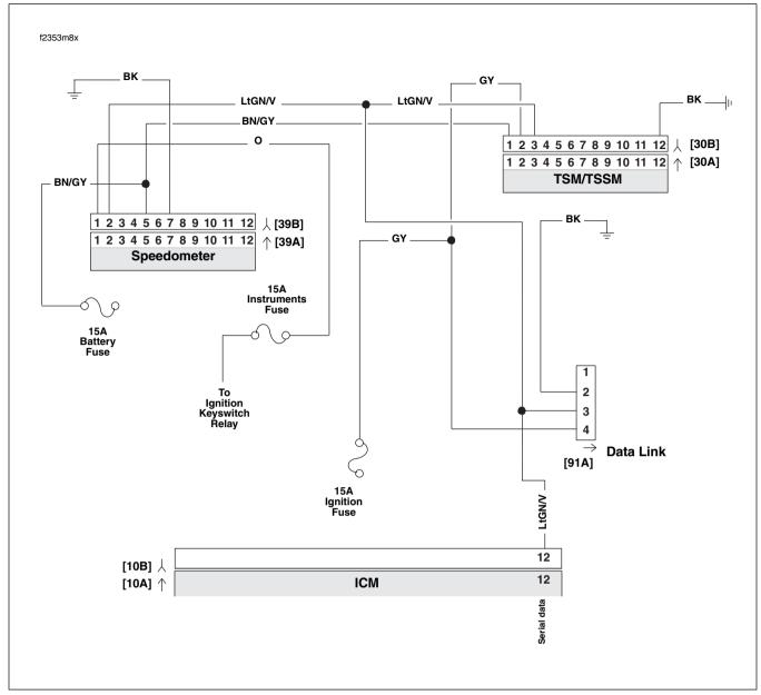
Figure 3-11. Diagnostic Check: FLHR/S (Carbureted)
