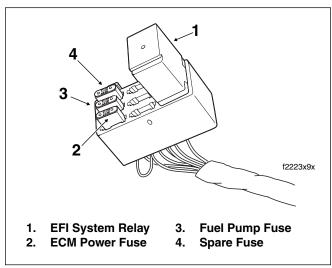
Figure 9-1. EFI Fuses (Under Right Side Cover)
