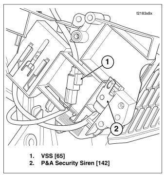
Figure 8-117. Electrical Bracket (Inboard Side)
