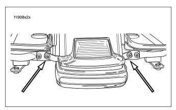
Figure 2-192. Rear Bumper Screws (T40 TORX)
