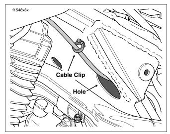
Figure 8-136. Cruise Cable Routing (Left Side)
