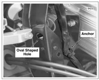
Figure 8-175. Anchor Conduit of Fairing Cap Switch Connector
