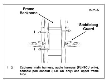
Figure 8-168. Capture Main Harness Conduit
