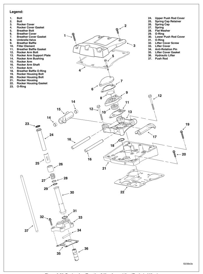
Figure 3-56. Rocker Arm/Breather/Lifter Assemblies (Exploded View)
