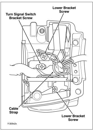
Figure 8-104. Lower Right Handlebar Switch Housing (Without Splices) - Classic/Ultra Models
