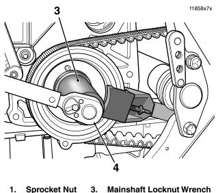
Figure 6-13. Install Mainshaft Locknut Pilot/Wrench and Torque Sprocket Nut
