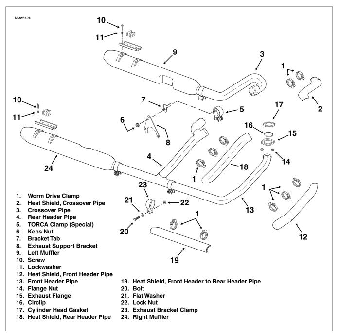
Figure 2-206. Remove/Install Exhaust System
