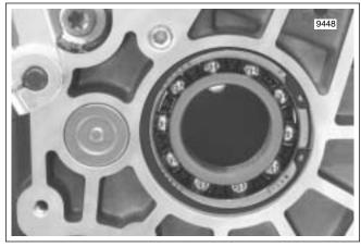
Figure 7-38. Install Retaining Ring With Gap Facing Rear
