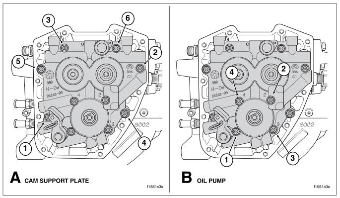
Figure 3-50. Cam Support Plate/Oil Pump Torque Sequence
