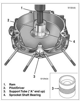
Figure 3-126. Install Sprocket Shaft Bearing
