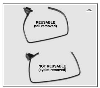
Figure 8-152. Cut Cable Straps
