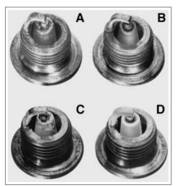
Figure 8-10. Types of Plug Base Deposits
