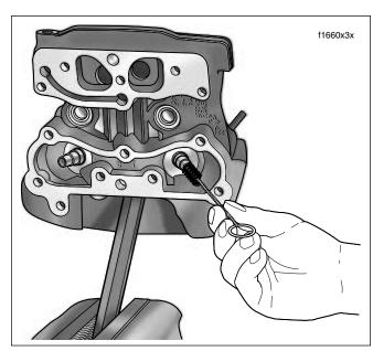
Figure 3-22. Scrub Valve Guide Bore
