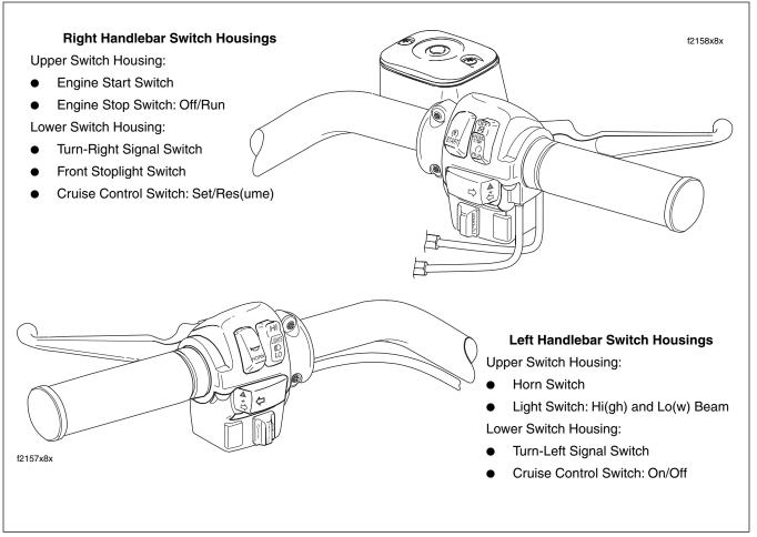
Figure 8-96. Road King Classic Handlebar Switch Assemblies
