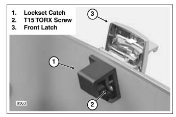
Figure 2-153. Front Latch Assembly
