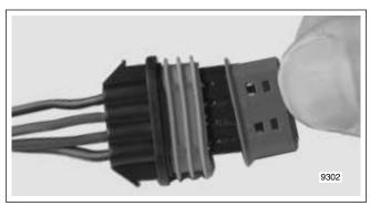
Figure B-17. Remove Terminal Lock
