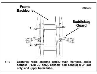
Figure 8-183. Capture Radio Antenna Cable
