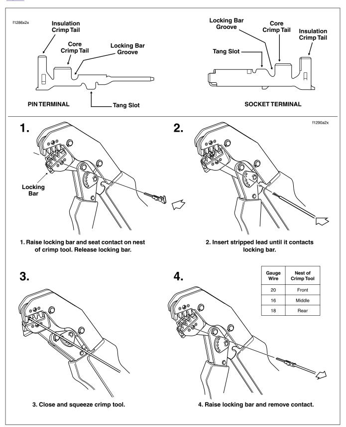
Figure B-15. Multilock Crimping Procedure
