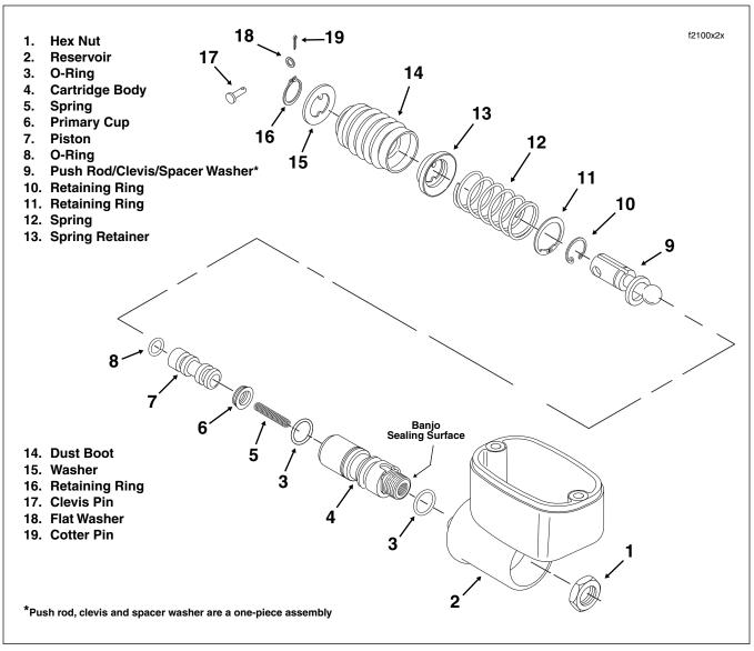
Figure 2-52. Rear Brake Master Cylinder Assembly (Exploded View)
