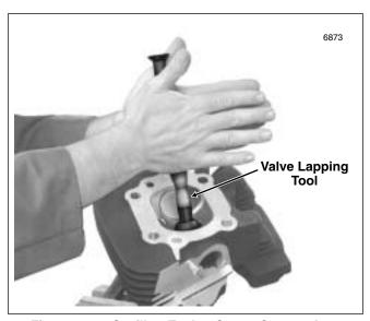
Figure 3-79. Oscillate Tool to Create Contact Area
