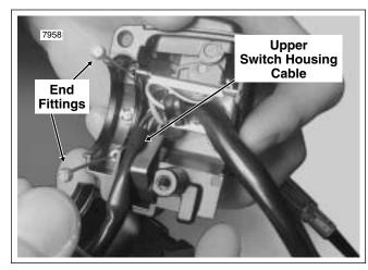
Figure 8-89. Route Cable to Upper Switch Housing
