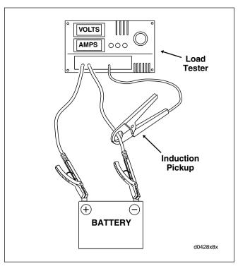
Figure 1-20. Load Test Battery
