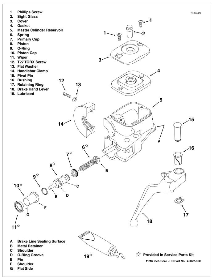
Figure 2-44. Front Brake Master Cylinder Assembly
