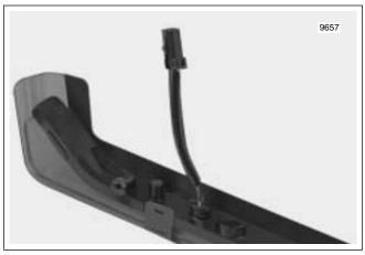
Figure 2-155. Side Marker Lights Assembly (FLHTCU)
