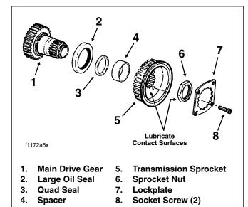
Figure 7-41. Install Transmission Sprocket Components
