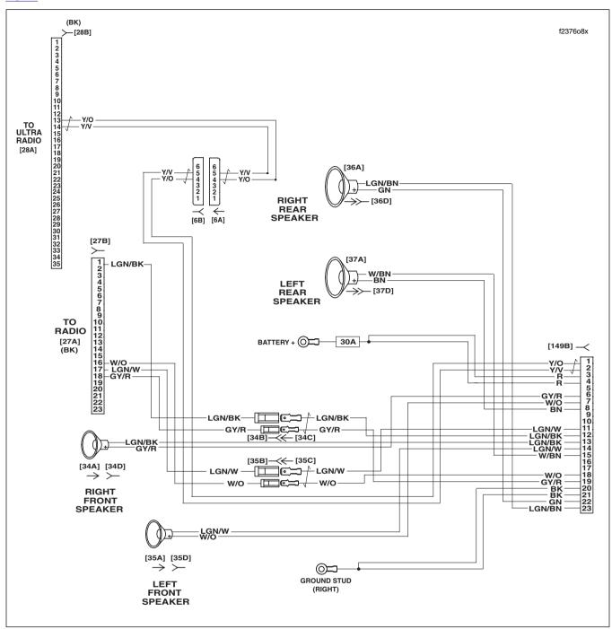
Figure 6-40. Front/Rear Speaker Circuits With Amplifier
