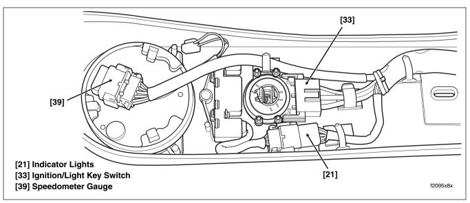
Figure 8-56. Instrument Console Connectors (FLHR/C)
