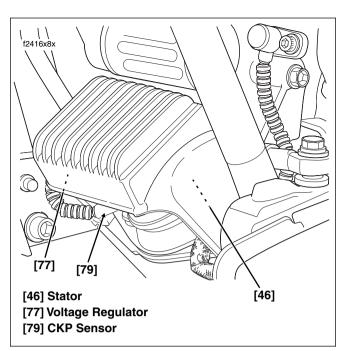
Figure 8-51. Voltage Regulator (Left Side View)
