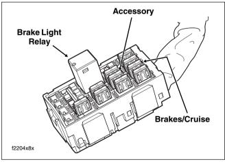
Figure 7-10. Fuse Block (FLHTCU-I)
