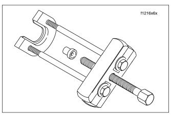
Figure 6-22. Mainshaft Bearing Inner Race Remover (Part No. HD-34902B)
