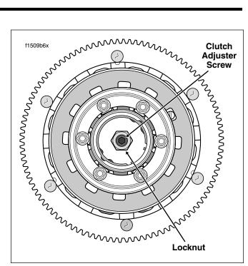
Figure 1-9. Clutch Assembly
