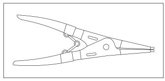
Part No. HD-95017-61 Large External Retaining **Ring Pliers**
