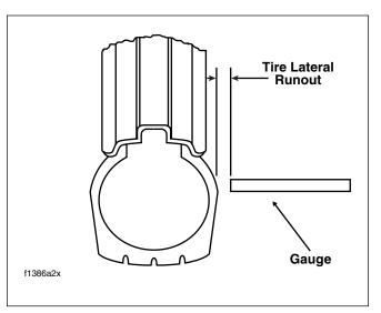
Figure 2-36. Checking Tire Lateral Runout
