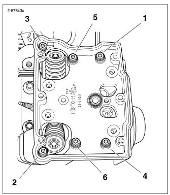
Figure 3-5. Rocker Housing Torque Sequence
