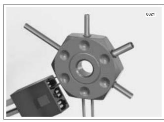
Figure 8-38. Depress Tangs and Remove Terminal
