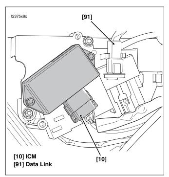
Figure 8-160. Electrical Bracket (Under Right Side Cover)
