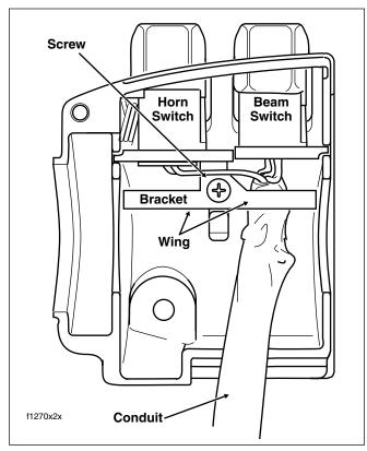
Figure 8-101. Upper Left Handlebar Switch Housing (Without Splices)
