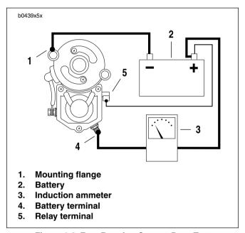
Figure 1-8. Free Running Current Draw Test
