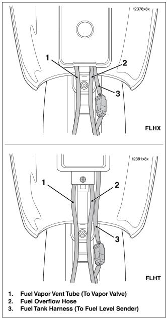
Figure 4-18. Console Cable/Hose Routing (FLHX, FLHT)
