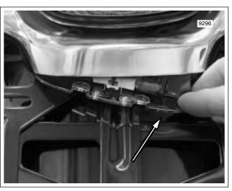
Figure 8-67. Release Lamp Assembly
