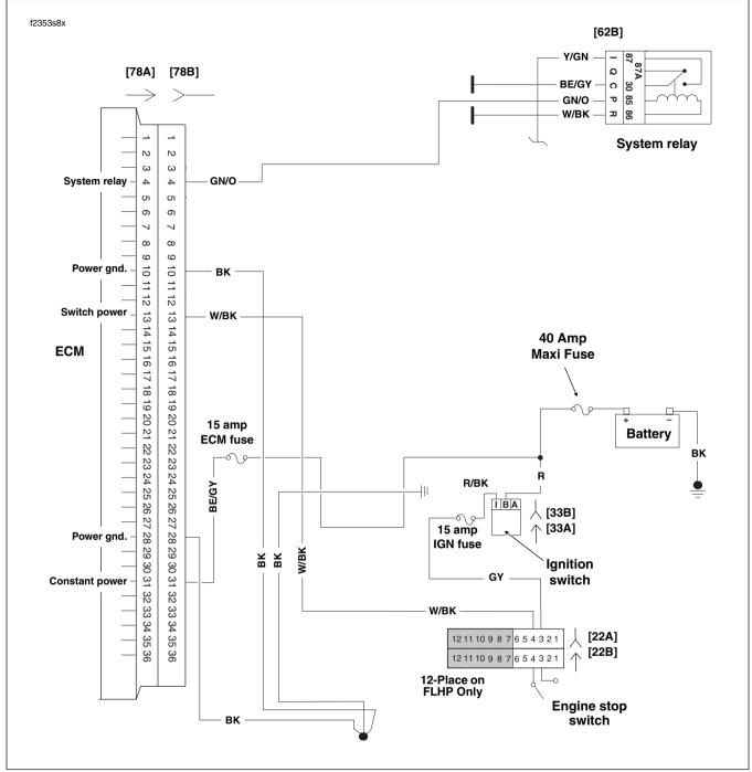
Figure 5-61. Battery Voltage Circuit (FLHR/C/S)
