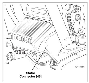
Figure 8-13. Voltage Regulator (Left Side View)
