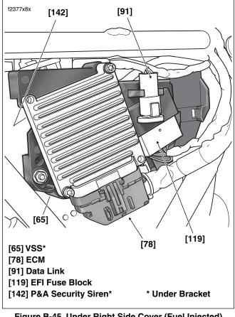
Figure B-45. Under Right Side Cover (Fuel Injected)
