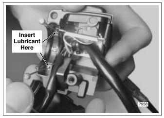
Figure 2-112. Right Handlebar Lower Switch Housing
