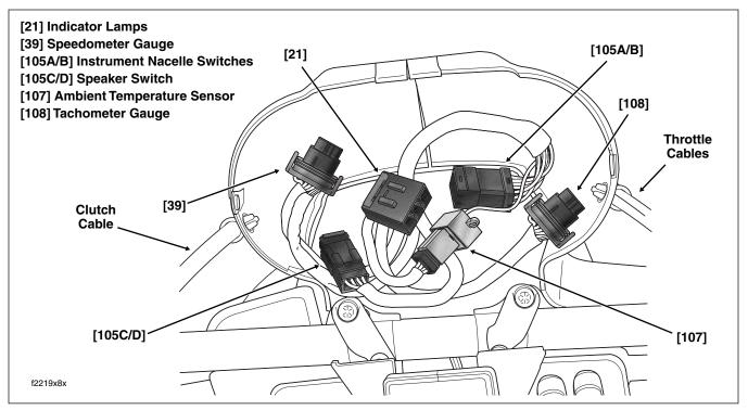
Figure 2-177. Instrument Nacelle (Bezel Removed)
