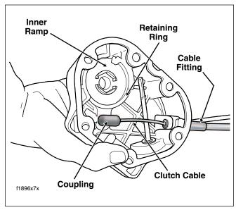
Figure 7-4. Clutch Release Cover Assembly
