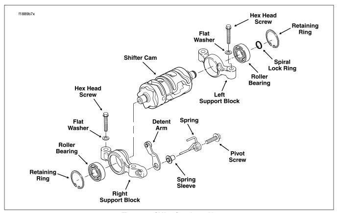
Figure 7-3. Shifter Cam Assembly
