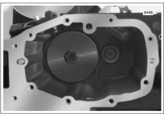
Figure 7-36. Main Drive Gear Installation (Right Side)
