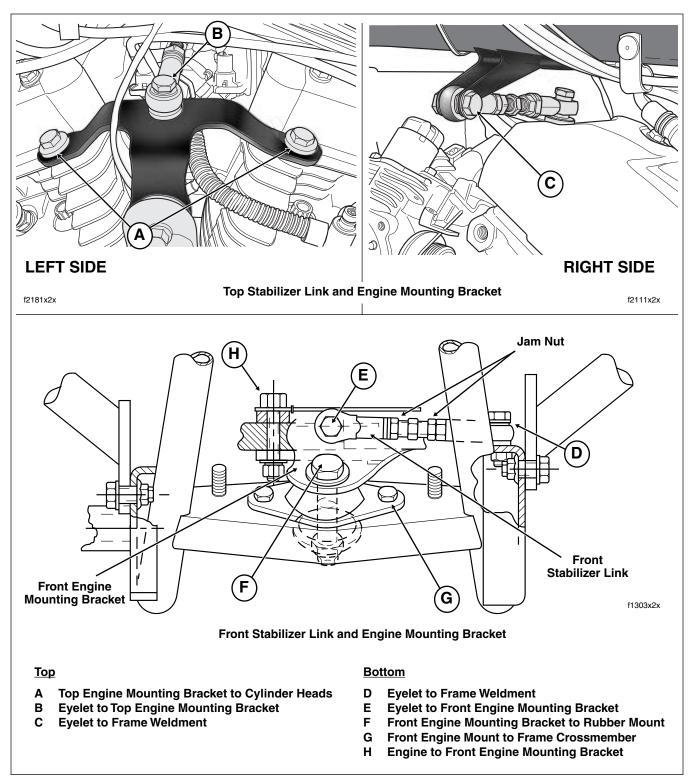
Figure 2-39. Engine Mounting Bracket Bolts
