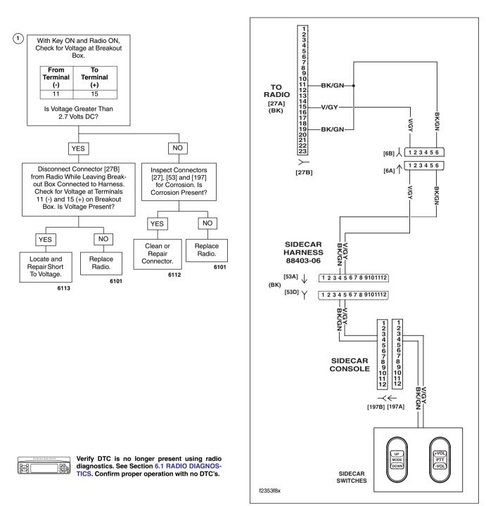
Figure 6-18. Sidecar Switch Circuit
