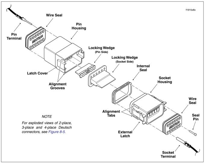
Figure 8-3. 12-Place Deutsch Connector (Exploded View)
