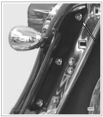
Figure 2-198. Remove Flange Nuts
