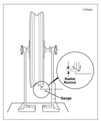
Figure 2-29. Truing Steel Laced Rim Radially
