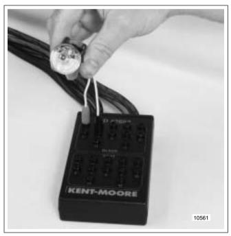
Figure 4-16. Ignition Coil Circuit Test
