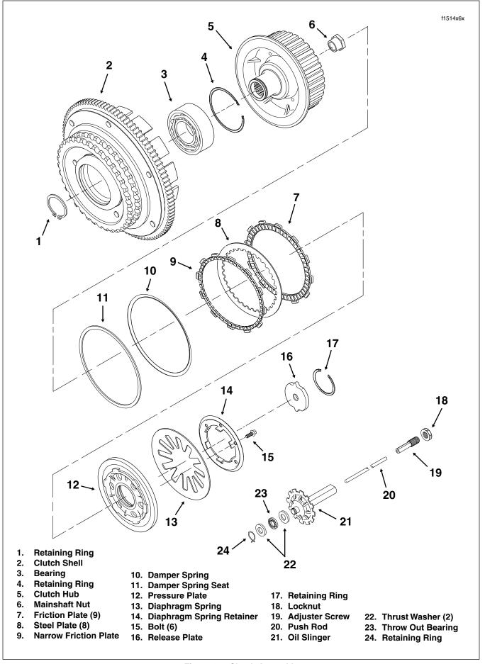
Figure 6-3. Clutch Assembly
