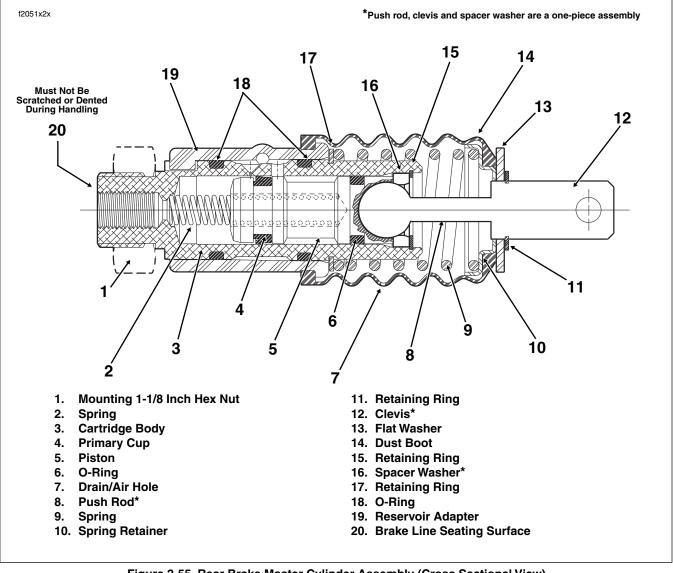
Figure 2-55. Rear Brake Master Cylinder Assembly (Cross Sectional View)
