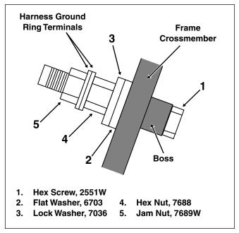
Figure 8-170. Install New Frame Ground Stud
