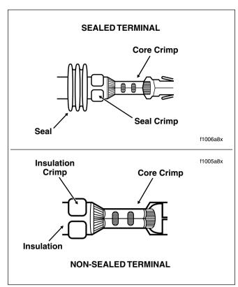
Figure 8-37. Inspect Core and Insulation/Seal Crimps
