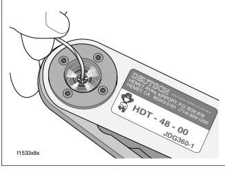
Figure 8-9. Deutsch Solid Barrel Contact Crimping Procedure
