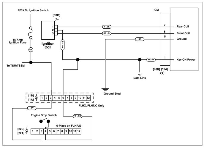
Figure 4-33. Battery Voltage Circuit
