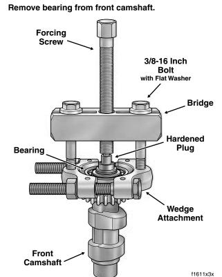
Figure 3-107. Remove Camshafts/Front Cam Bearing
