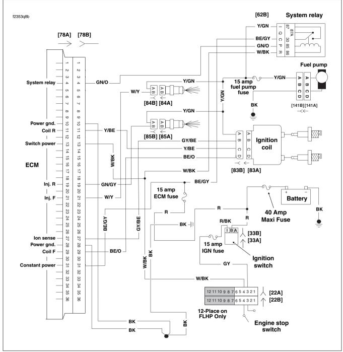
Figure 5-69. Battery Voltage Circuit (FLHR/C/S)
