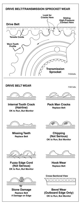
Figure 6-7. Drive Belt/Transmission Sprocket Wear
