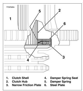
Figure 6-2. Clutch Pack Stack-Up (Cut-Away View)
