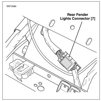
Figure B-49. Rear Fender (Under Seat)
