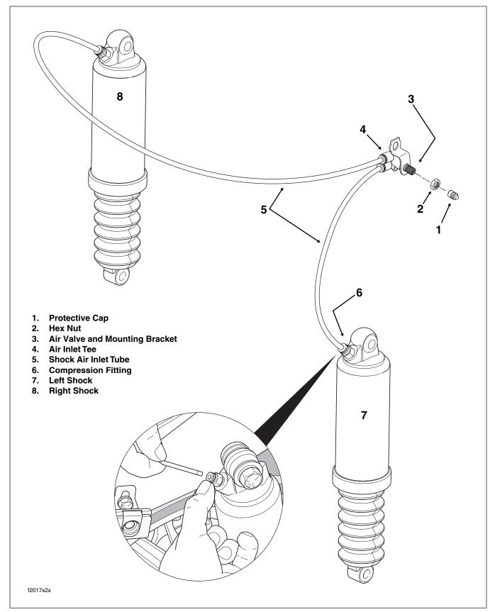
Figure 2-91. Rear Air Suspension System
