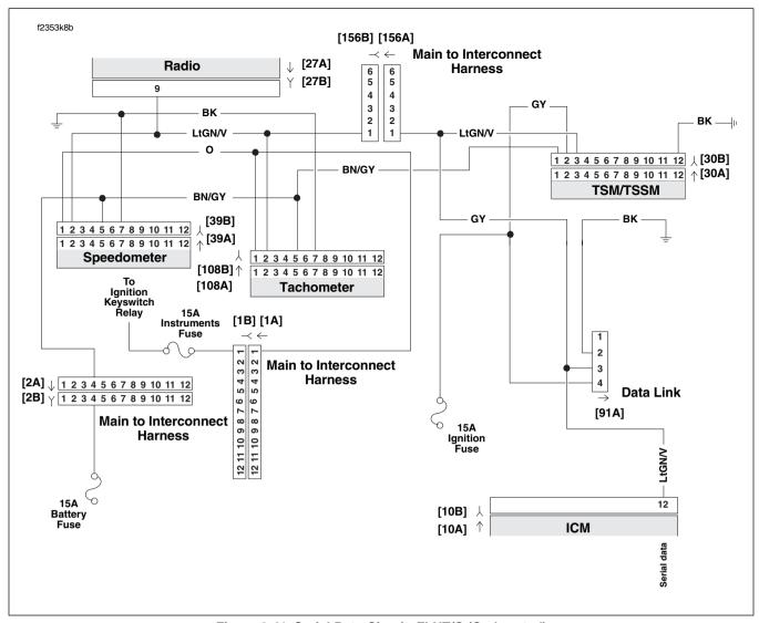
Figure 3-41. Serial Data Circuit: FLHT/C (Carbureted)
