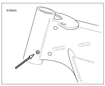
Figure 1-25. Steering Head Bearing Grease Fitting
