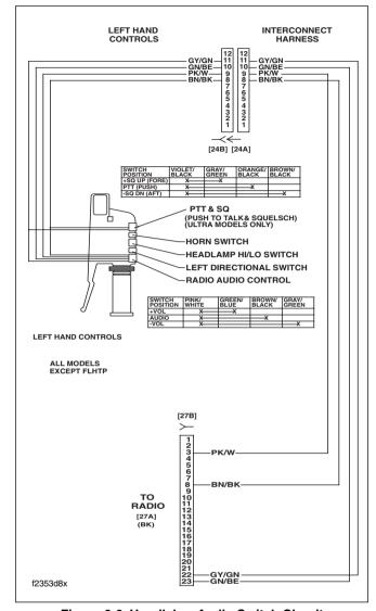
Figure 6-6. Handlebar Audio Switch Circuit
