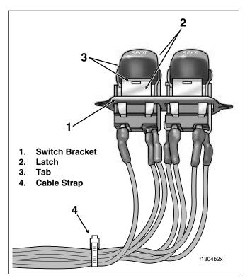
Figure 8-81. Bend Latches Outward to Release Tabs
