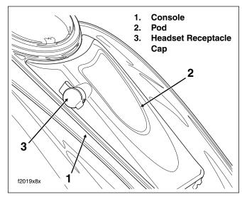
Figure 8-142. Console Pod Assembly
