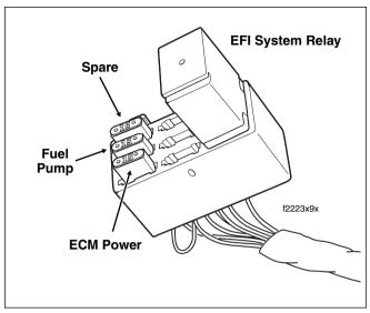
Figure 5-28. EFI Fuse Block
