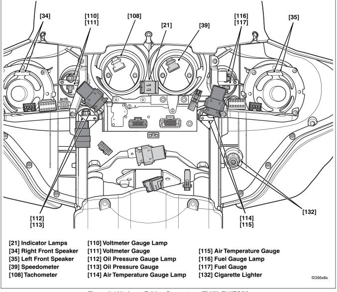
Figure 2-165. Inner Fairing Connectors (FLHX, FLHTC/U)
