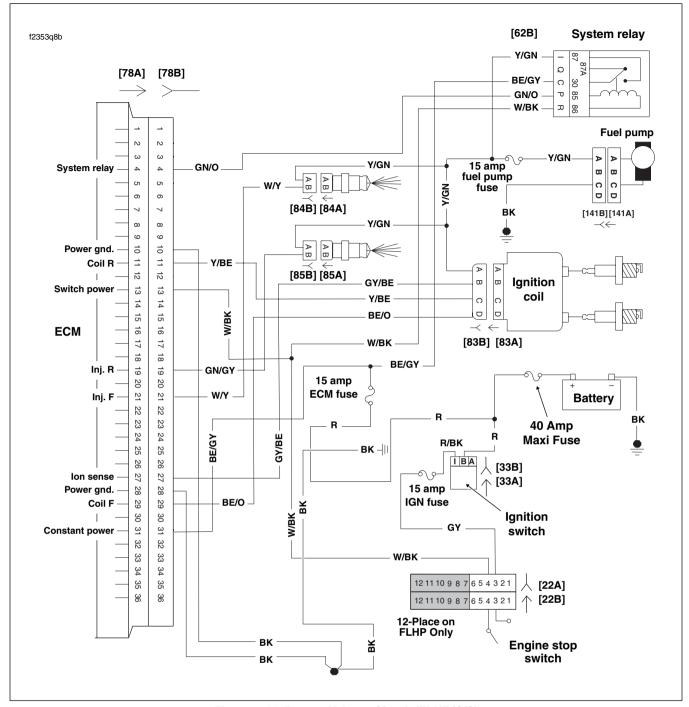
Figure 5-44. Battery Voltage Circuit (FLHR/C/S)
