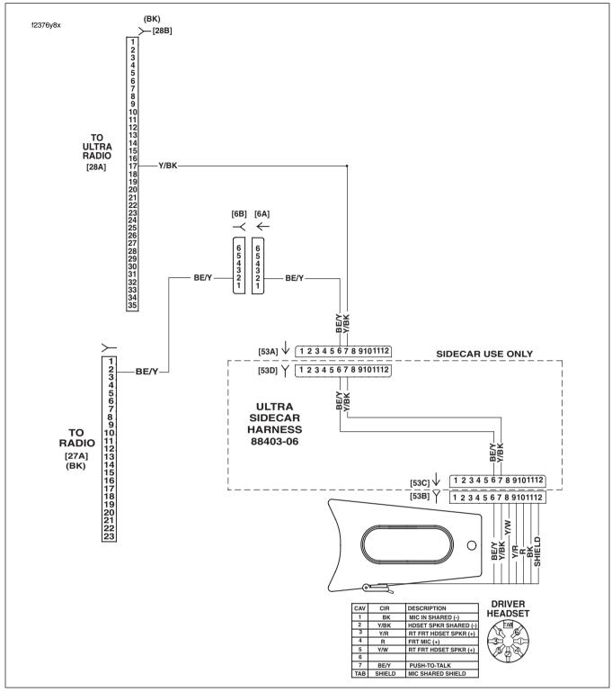
Figure 6-36. Handheld Microphone/PTT Circuit
