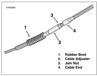
Figure 1-8. Clutch Cable Adjuster Mechanism
