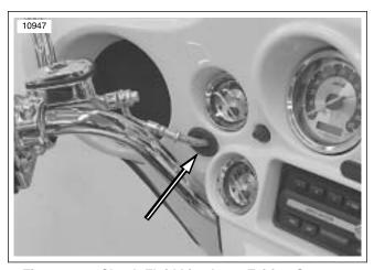
Figure 2-38. Clutch Fluid Line Inner Fairing Grommet
