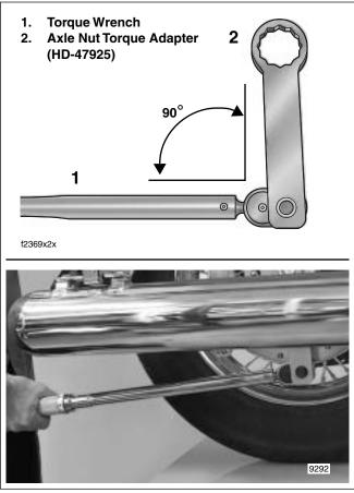
Figure 1-15. Install Tool Perpendicular to Torque Wrench
