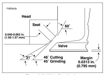
Figure 3-80. Valve Seat Angles
