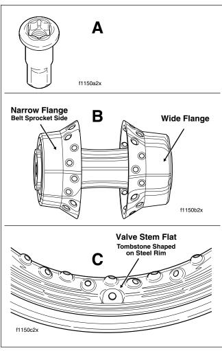
Figure 2-18. Spoke Nipple, Hub and Rim
