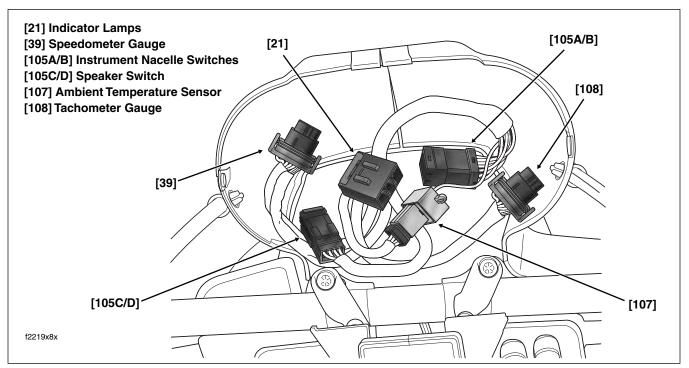
Figure B-53. Instrument Nacelle Connectors (FLTR)
