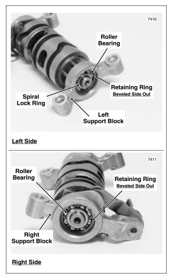
Figure 7-10. Shifter Cam Assembly
