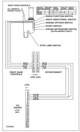
Figure 6-4. Handlebar Mode Switch Circuit
