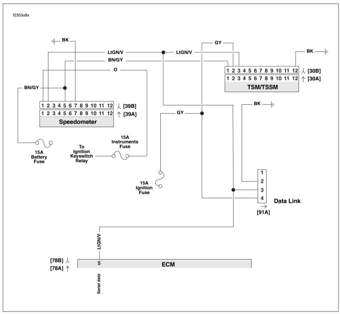
Figure 5-65. Serial Data Circuit (FLHR/C/S)
