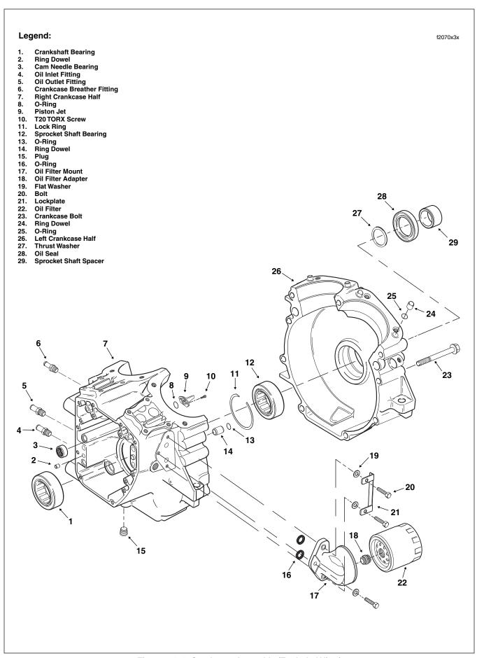
Figure 3-121. Crankcase Assembly (Exploded View)
