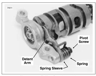
Figure 7-11. Shifter Cam Assembly
