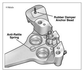
Figure 2-71. Install Anti-Rattle Spring
