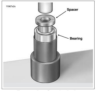
Figure 2-98. Press Spacer Into Bearing
