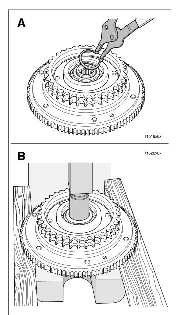
B Press clutch hub from bearing.
