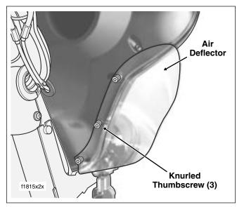
Figure 2-170. Remove/Install Air Deflectors
