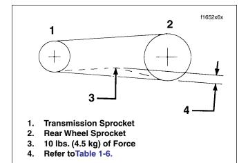
Figure 1-14. Check and Adjust Belt Deflection
