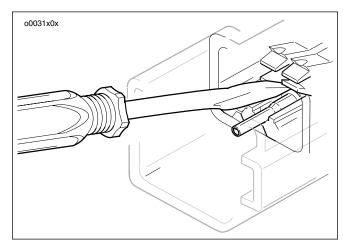
Figure 2-15. Internal Deutsch Terminal Latches
