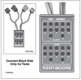
Figure 4-10. Breakout Box (Part No. HD-42682)
