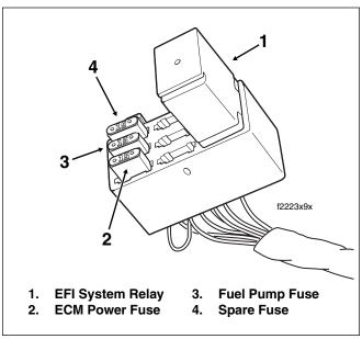
Figure 9-3. EFI Fuse Block
