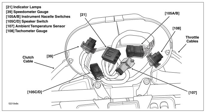
Figure 8-83. Instrument Nacelle (Bezel Removed)
