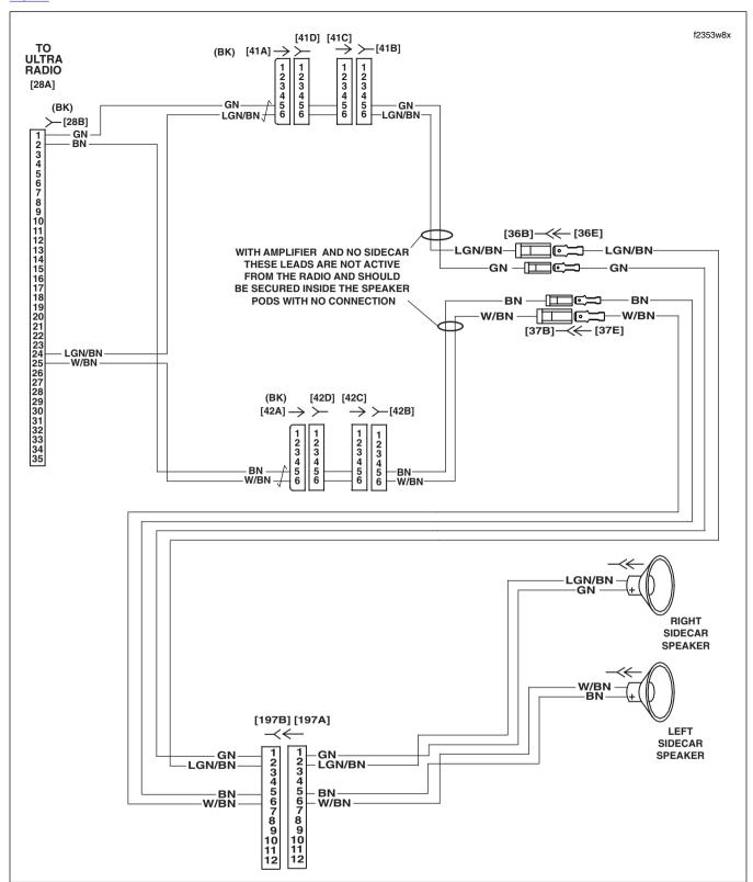
Figure 6-23. Sidecar Speaker Circuit
