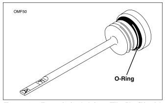
Figure 2-120. Transmission Lubricant Filler Plug/Dipstick
