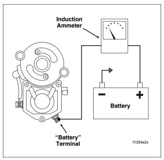
Figure 1-4. Starter Current Draw Test
