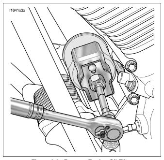
Figure 3-3. Remove Engine Oil Filter
