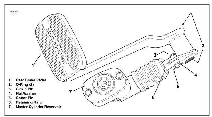
Figure 2-47. Rear Brake Pedal/Master Cylinder Assembly
