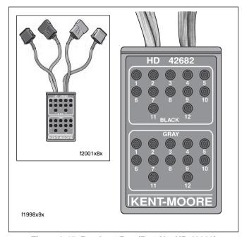
Figure 2-17. Breakout Box (Part No. HD-42682)
