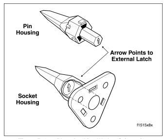
Figure B-4. 3-Place Locking Wedge Orientation
