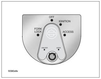
Figure 4-3. Ignition Switch (FLHX, FLHT/C)
