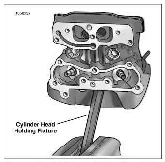
Figure 3-8. Install Cylinder Head Holding Fixture in Vise
