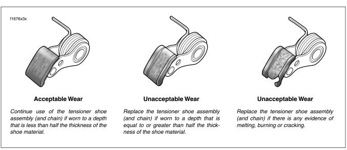
Figure 3-114. Cam Chain Tensioner Shoe Wear
