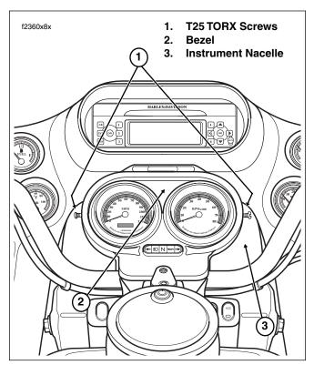
Figure 2-176. Remove Instrument Bezel Screws
