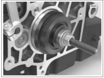
Figure 7-35. Main Drive Gear Bearing Installation (Left Side)
