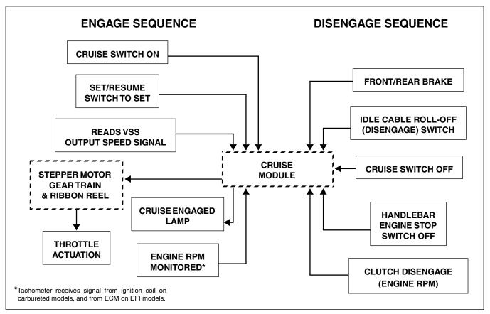
Figure 8-131. Cruise System Diagram
