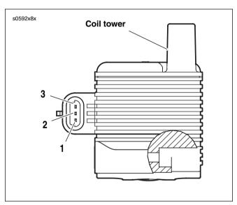
Figure 4-32. Ignition Coil Connector Terminals
