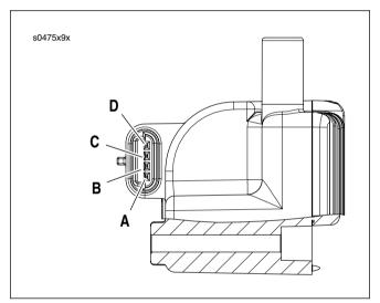
Figure 5-67. Ignition Coil Connector Terminals
