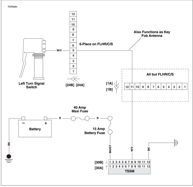
Figure 3-25. Antenna Circuit
