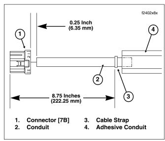
Figure 2-196. Install Cable Strap on Conduit
