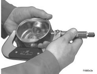
Figure 3-87. Measure Early Style Piston for Running Clearance
