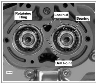
Figure 7-23. Side Door Bearings
