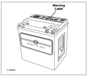
Figure 8-17. Maintenance-Free Battery
