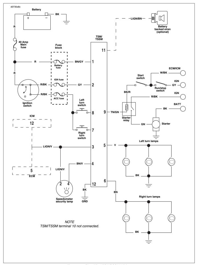
Figure 3-3. Simplified TSM/TSSM Wiring
