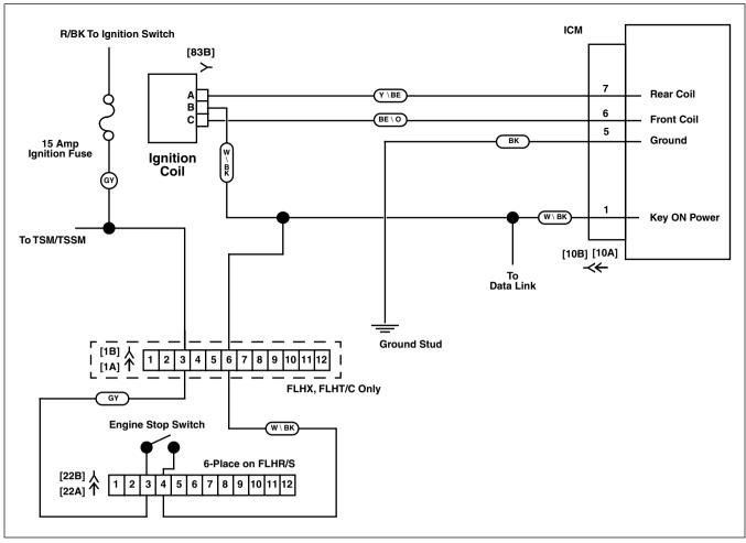
Figure 4-26. Battery Voltage Circuit
