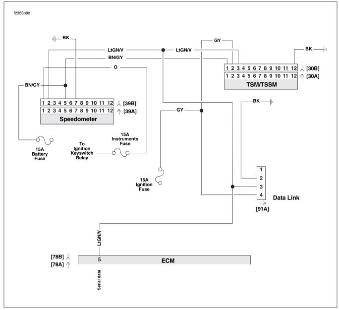
Figure 5-77. Serial Data Circuit (FLHR/C/S)
