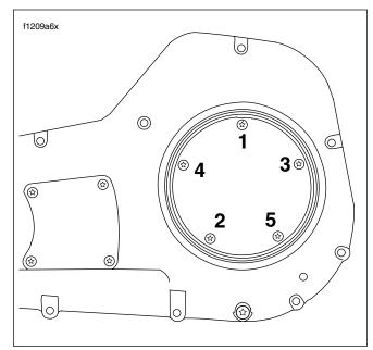
Figure 6-3. Clutch Inspection Cover Torque Sequence
