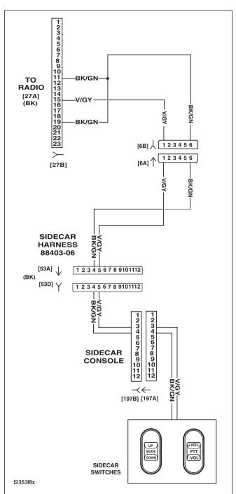
Figure 6-20. Sidecar Switch Circuit
