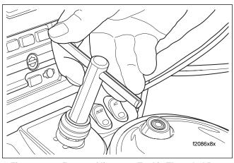
Figure 8-73. Bottom Alignment Tool in Threaded Post and Rotate to Desired Position
