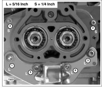
Figure 7-40. Side Door Screw Size and Torque Sequence
