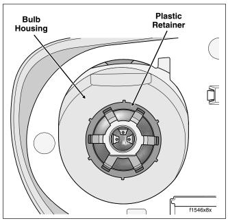
Figure 8-29. Remove Retainer to Release Bulb
