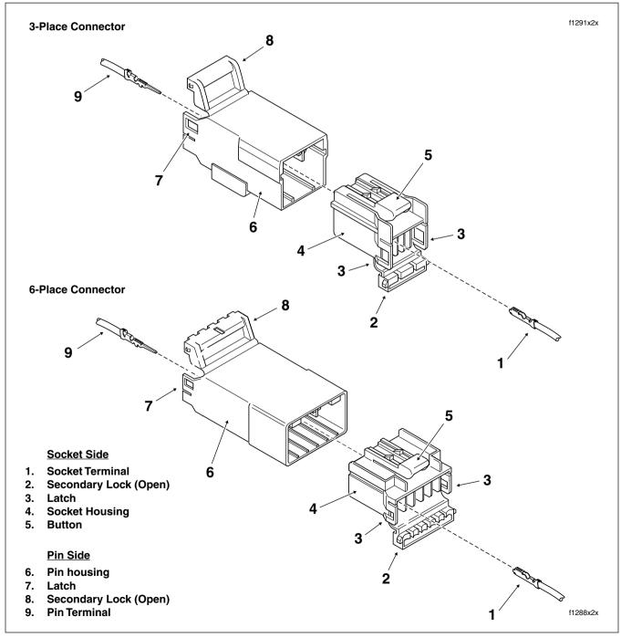
Figure 8-14. 3-Place and 6-Place Multilock Connectors
