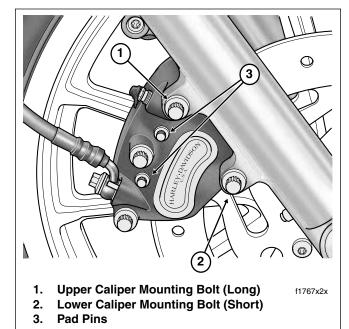
Figure 2-57. Loosen Pad Pins and Remove Caliper Mounting Bolts (Right Side View)
