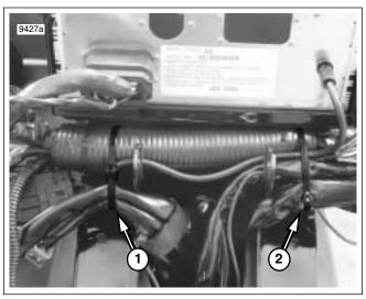
Figure 8-179. Cable Strap Convoluted Tubing and Conduit
