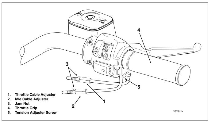
Figure 2-106. Throttle Cable Assembly - Throttle Side (FLHR)
