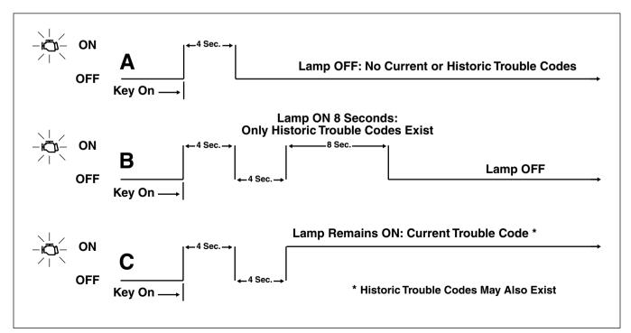
Figure 4-4. Check Engine Lamp Operation
