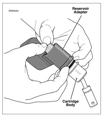
Figure 2-51. Remove Cartridge From Reservoir Adapter
