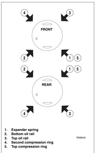
Figure 3-90. Piston Ring Gap Alignment
