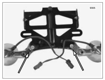
Figure 8-69. Remove License Plate Bracket
