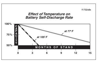
Figure 8-23. Battery Self-Discharge Rate
