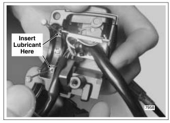
Figure 1-19. Lubricate Throttle/Idle Cables
