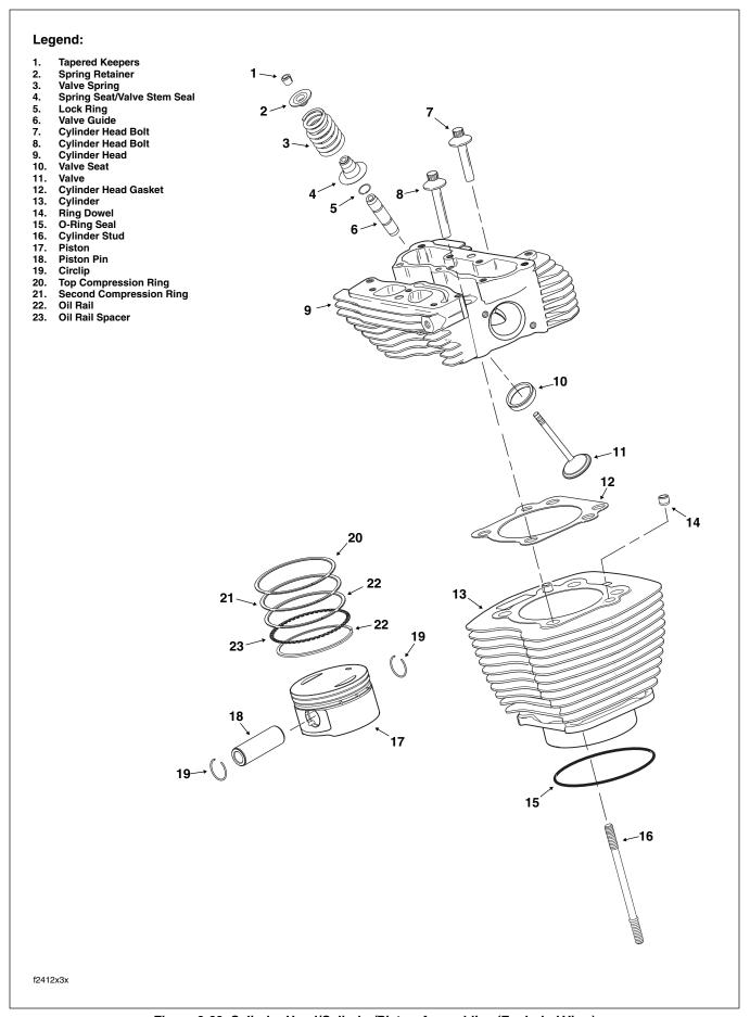
Figure 3-62. Cylinder Head/Cylinder/Piston Assemblies (Exploded View)
