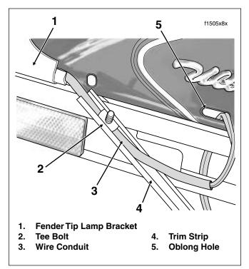
Figure 8-48. Install Conduit in Trim Strip
