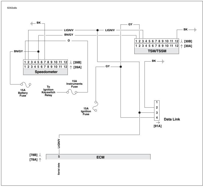
Figure 3-44. Serial Data Circuit: FLHR/C/S (Fuel Injected)
