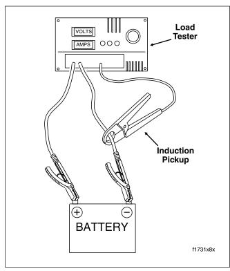
Figure 8-21. Load Test Battery
