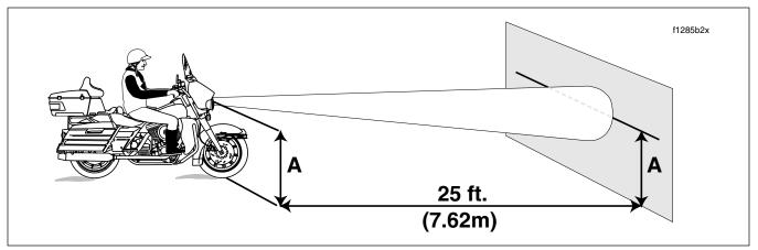
Figure 8-26. Check Headlamp Alignment
