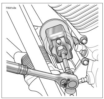
Figure 1-1. Remove Engine Oil Filter
