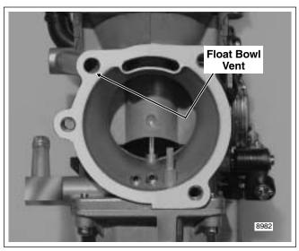
Figure 4-4. Drain Carburetor Float Bowl
