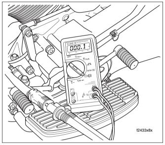
Figure 1-16. Check for Stator Resistance
