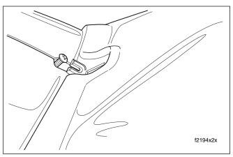
Figure 2-186. Remove Screw From Slot in Wind Deflector
