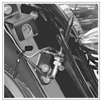
Figure 8-167. Capture Radio Antenna Cable (FLHX)
