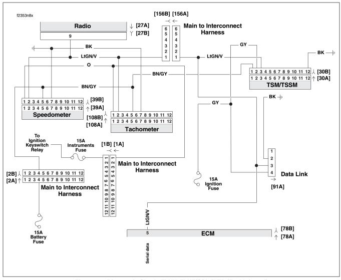
Figure 2-9. Diagnostic Check: FLHX, FLHT/C/U, FLTR (Fuel Injected)
