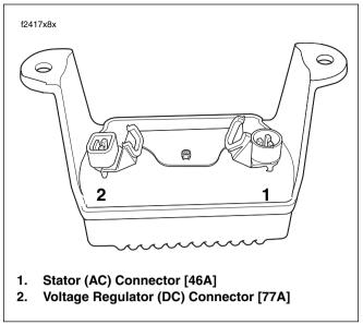
Figure 1-10. Voltage Regulator (Bottom View)
