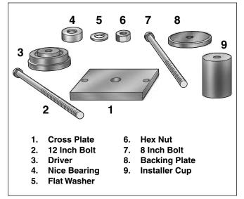
Figure 7-28. Main Drive Gear/Bearing Remover/Installer (Part No. HD-35316B)
