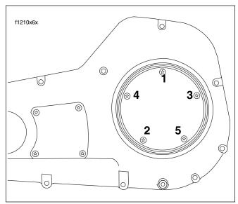
Figure 6-34. Clutch Inspection Cover Torque Sequence
