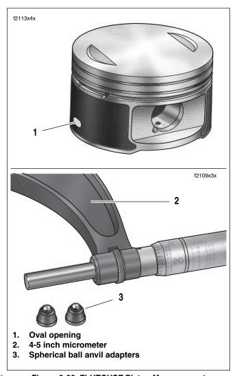
Figure 3-33. FLHTCUSE Piston Measurement
