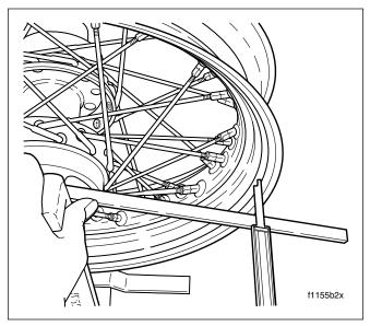
Figure 2-28. Checking Steel Laced Hub Offset Dimension
