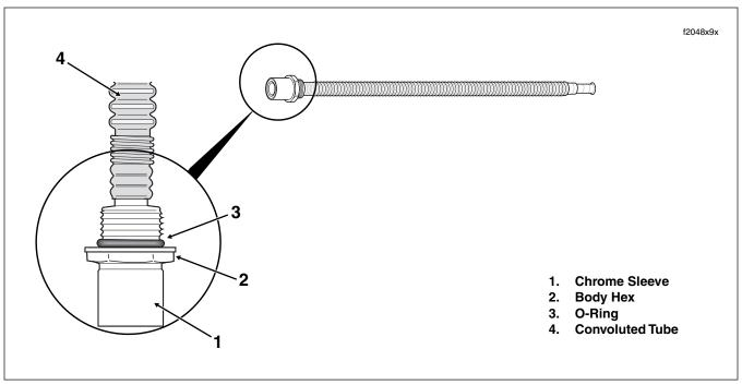
Figure 9-22. Fuel Supply Check Valve/Tube (Quick-Connect Fitting)
