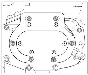
Figure 7-13. Clutch Release Cover Torque Sequence
