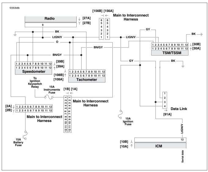
Figure 2-34. Serial Data Circuit: FLHX, FLHT/C (Carbureted)
