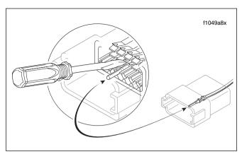
Figure 8-2. Depress Terminal Latches/Back Out Pins
