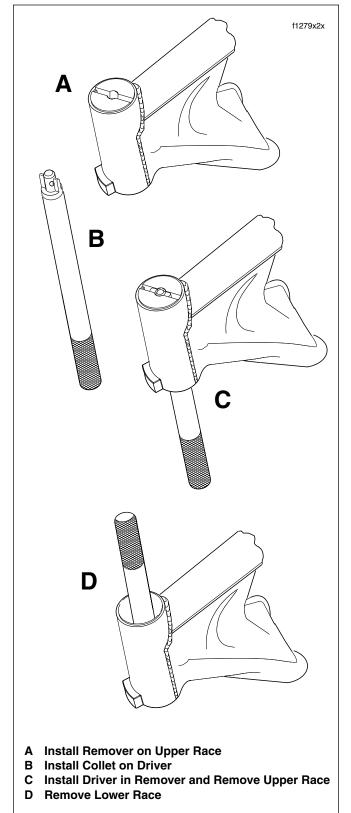
Figure 2-89. Remove Upper and Lower Steering Head Bearing Races
