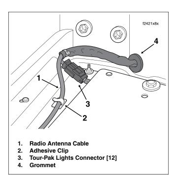
Figure 2-144. Disconnect Tour-Pak Lights Connector
