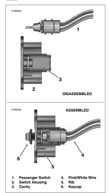
Figure 8-147. Install Switch in Housing
