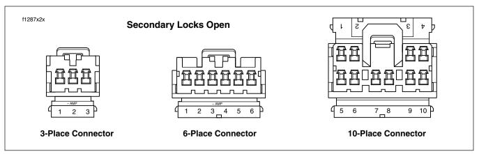
Figure 8-13. Numbers Stamped on Secondary Locks for Wire Color Locations (Socket Housings Shown)
