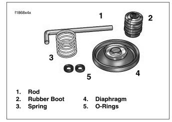
Figure 4-9. Accelerator Pump Components
