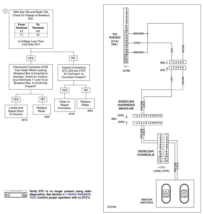
Figure 6-19. Sidecar Switch Circuit
