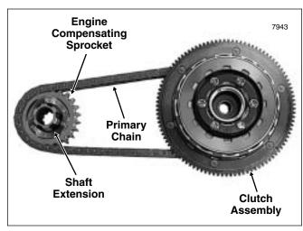
Figure 6-21. Remove Clutch Assembly, Primary Chain, Engine Compensating Sprocket and Shaft Extension
