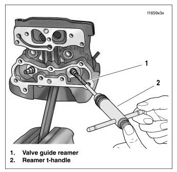
Figure 3-18. Ream Valve Guide Bore
