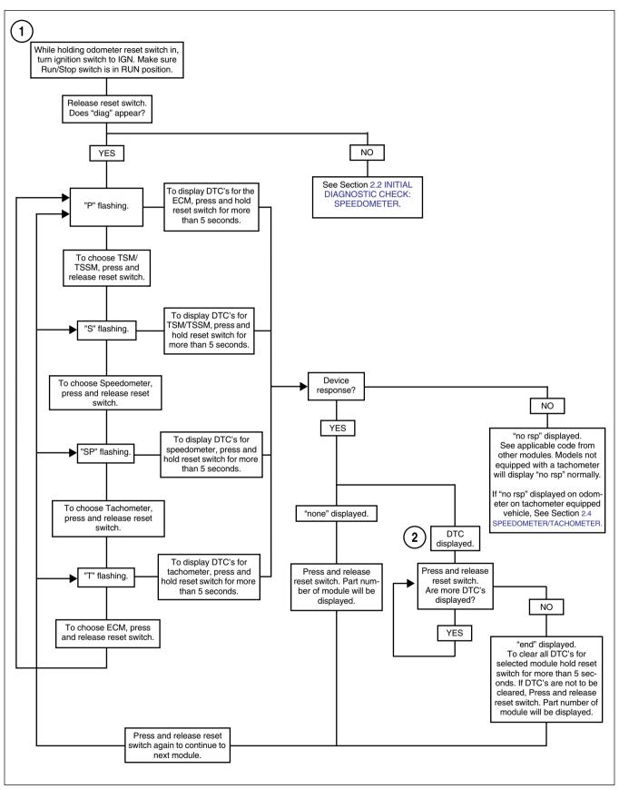
Figure 5-9. Speedometer Self Diagnostics
