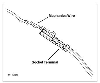
Figure 8-58. Fix Mechanics Wire to Socket Terminals
