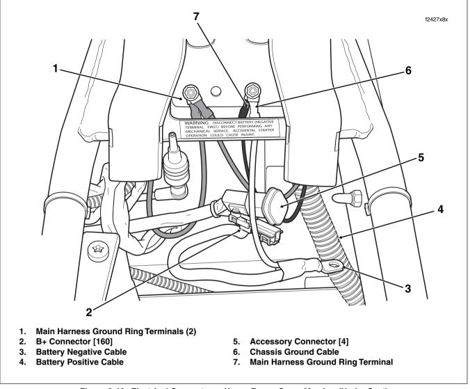
Figure 8-46. Electrical Connectors - Upper Frame Cross Member (Under Seat)
