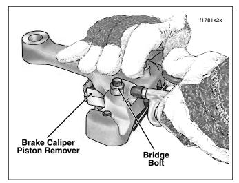
Figure 2-69. Direct Compressed Air Into Banjo Bolt Hole
