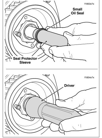
Figure 7-48. Install Small Oil Seal Using Seal Protector Sleeve and Driver
