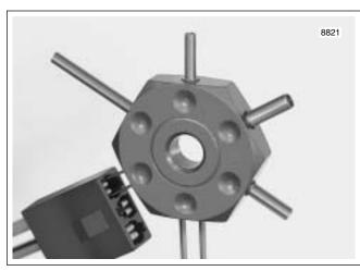
Figure B-38. Depress Tangs and Remove Terminal
