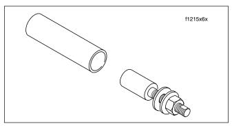
Figure 6-24. Mainshaft Bearing Inner Race Installer (Part No. HD-34902B)
