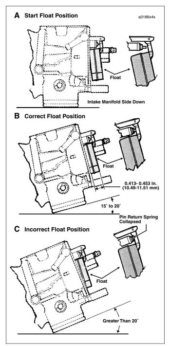
Figure 4-12. Float Check and Adjustment
