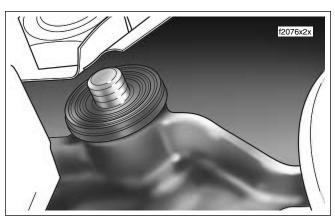
Figure 2-123. Remove Upper Bushing (Right Side)
