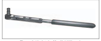
Figure 3-13. Intake Manifold Wrench (Part No. HD-47250)
