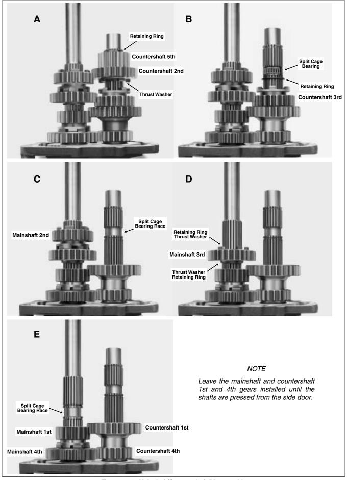
Figure 7-21. Mainshaft/Countershaft Disassembly
