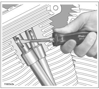
Figure 3-21. Remove Spring Cap Retainer
