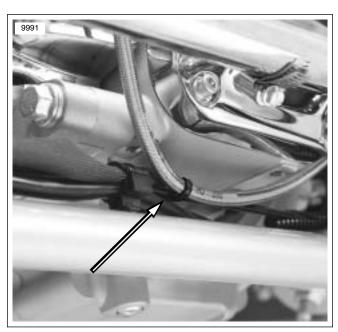
Figure 2-40. Cable Wrap Locations around Clutch Fluid Line
