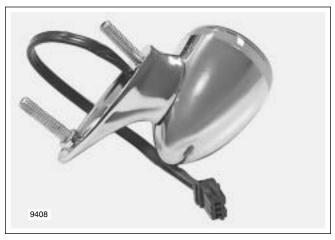
Figure 2-175. Front Turn Signal Lamp
