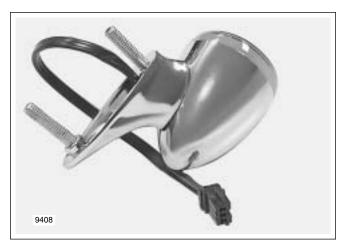
Figure 8-64. Front Turn Signal Lamp (FLTR)
