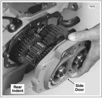
Figure 7-27. Remove Transmission Side Door
