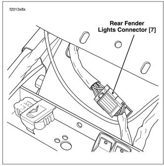
Figure 8-49. Rear Fender (Under Seat)
