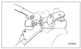
Figure 8-30. Raise Locking Bar and Barrel Holder
