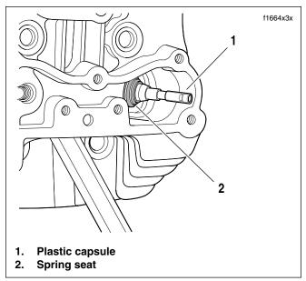
Figure 3-27. Install Plastic Capsule on Valve Stem
