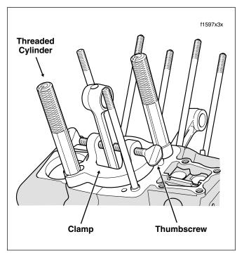
Figure 3-92. Install Connecting Rod Clamping Tool
