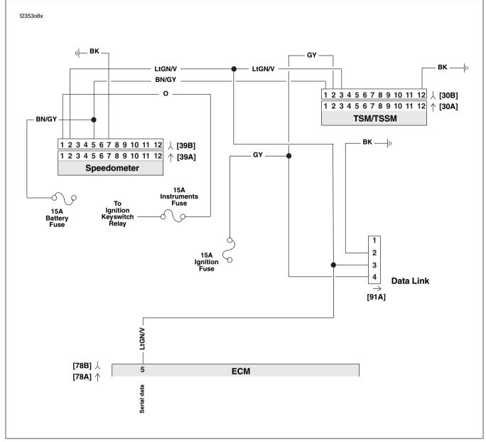
Figure 5-24. Serial Data Circuit (FLHR/C/S)
