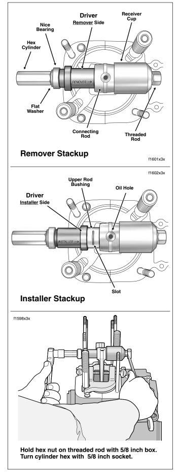
Figure 3-94. Remove/Install Connecting Rod Bushing
