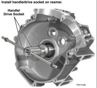
Figure 3-104. Ream Crankshaft Bushing
