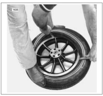
Figure 2-33. Starting Bead on Rim
