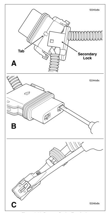
Figure 8-25. Remove Socket Terminals
