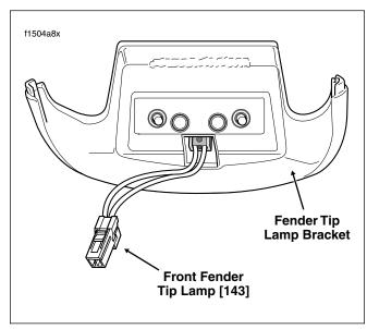
Figure 8-47. Fender Tip Lamp Assembly
