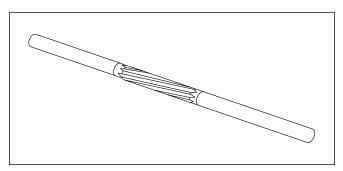
Part No. HD-94804-57 Rocker Arm Bushing Reamer
