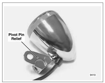
Figure 8-61. Front Right Turn Signal Lamps (FLHRS)
