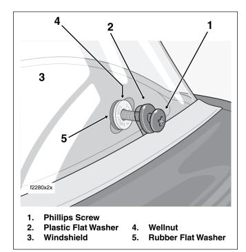
Figure 2-172. Install Windshield (Decal Removed for Illustration Purposes)
