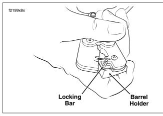
Figure B-31. Position Contact in Crimper
