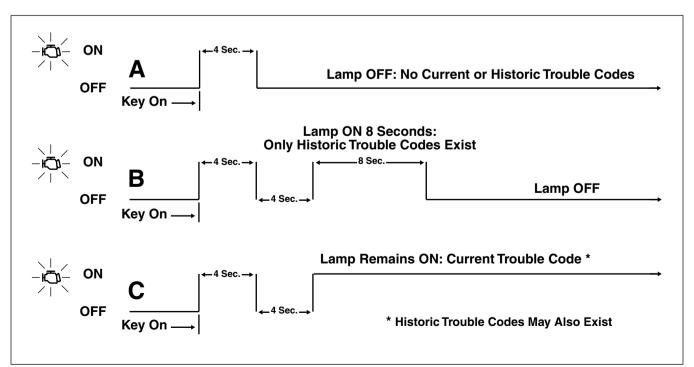
Figure 5-5. Check Engine Lamp Operation
