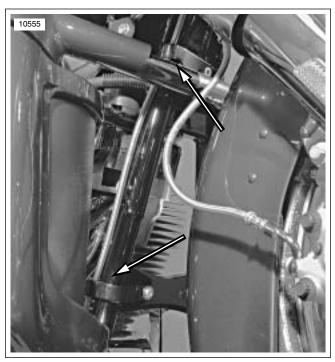
Figure 2-39. Clamp Locations on Frame Down Tube
