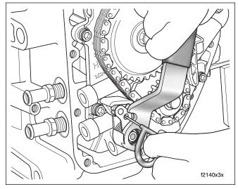
Figure 3-42. Retract Primary Cam Chain Tensioner
