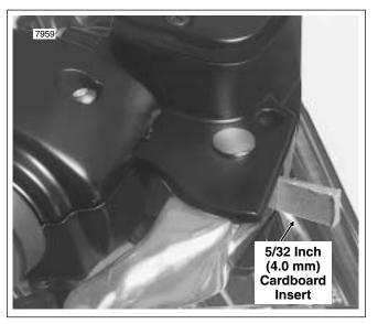
Figure 8-87. Install Cardboard Insert
