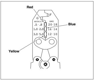
Figure 8-39. Packard Crimp Tool (HD-38125-8)
