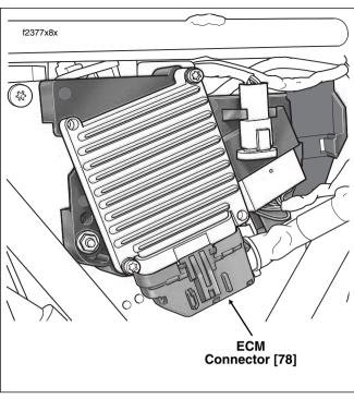
Figure 5-10. Electrical Bracket (Under Right Side Cover)
