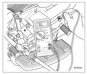
Figure 1-15. Test for Grounded Stator
