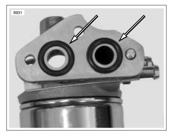
Figure 3-51. Oil Filter Mount O-rings (thermostat removed)
