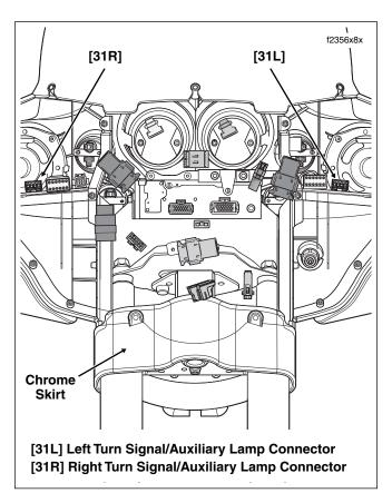
Figure 2-164. Inner Fairing (Front View)
