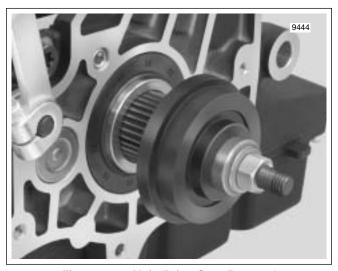
Figure 7-30. Main Drive Gear Removal (Left Side)
