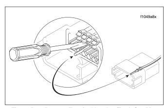
Figure B-2. Depress Terminal Latches/Back Out Pins
