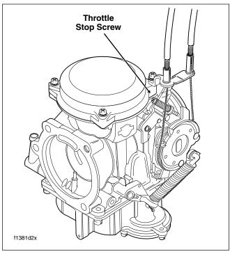
Figure 1-24. Idle Speed Adjustment
