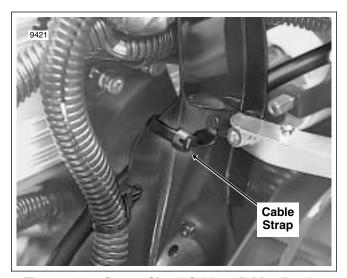
Figure 2-118. Secure Clutch Cable to Fairing Bracket
