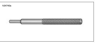
Figure 3-13. Valve Guide Driver (Part No. HD-34740)
