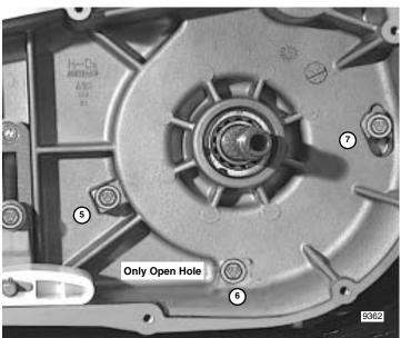
Figure 6-28. Primary Chaincase Screw Size and Torque Sequence
