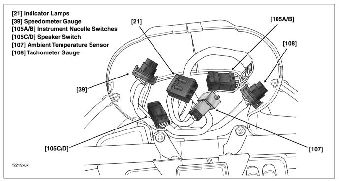
Figure 8-53. Instrument Nacelle Connectors (FLTR)
