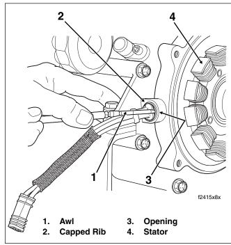
Figure 8-14. Remove Grommet From Crankcase
