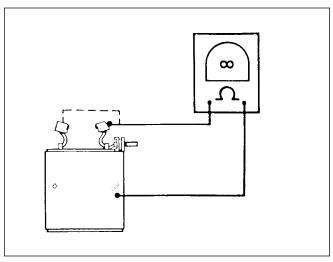
Figure 5-14. Grounded Field Test
