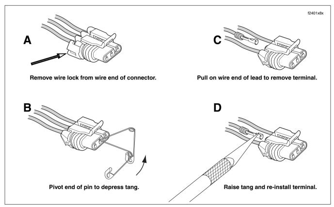
Figure 8-20. Depress Tang and Extract Terminal From Wire End of Push-to-Seat Connector
