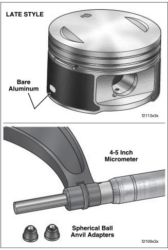
Figure 3-88. Measure Late Style Piston for Running Clearance
