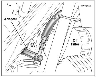
Figure 3-5. Install Adapter and Oil Pressure Gauge
