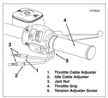
Figure 1-20. Throttle Cable Assembly - Throttle Side (FLHR/S)
