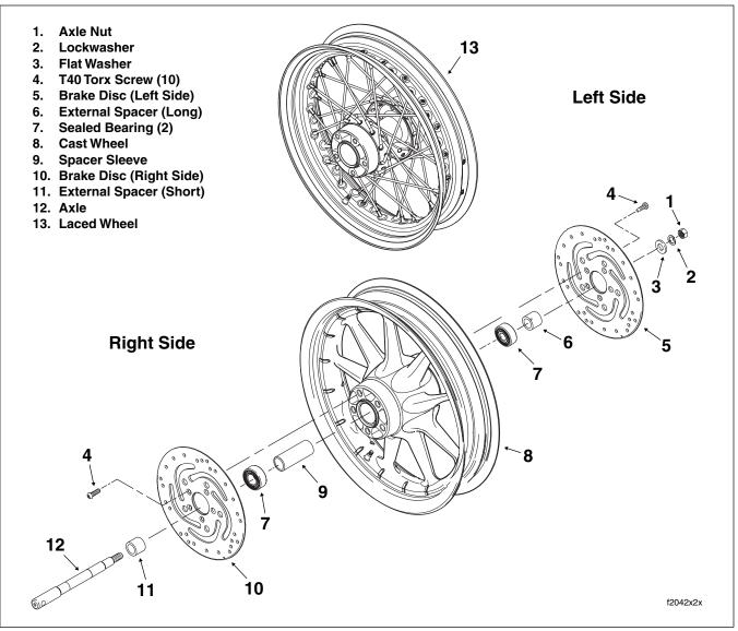
Figure 2-5. Front Wheel (Exploded View)
