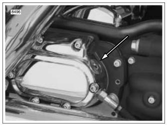
Figure 2-119. Clutch Release Cover
