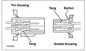
Figure 8-12. Tang Location (Cross Sectional View)
