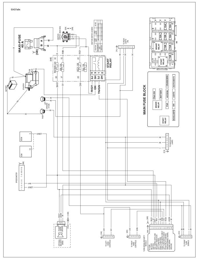
Figure 3-28. Turn Signal Circuit: FLHR/C/S
