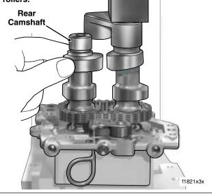
Figure 3-112. Install Cam Bearings/Camshafts
