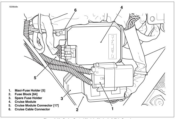
Figure 8-43. Cruise Control Module (Under Left Side Cover)
