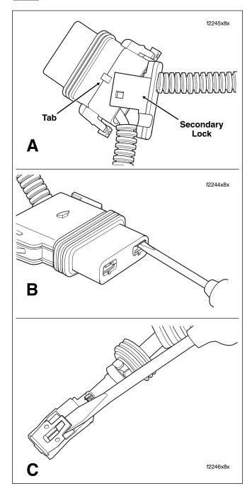
Figure B-25. Remove Socket Terminals
