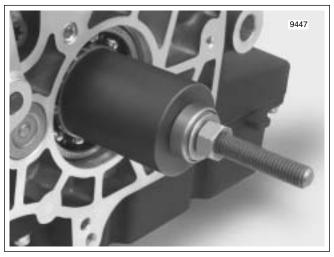
Figure 7-37. Main Drive Gear Installation (Left Side)
