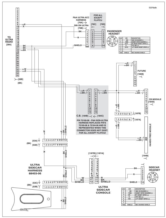
Figure 6-39. Microphone Audio Input Circuit
