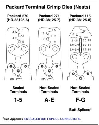
Figure 8-36. Packard Terminal Crimp Tools
