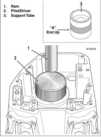
Figure 3-123. Remove Crankshaft Bearing
