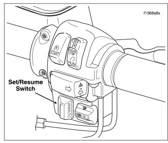
Figure 8-129. Right Handlebar Switch Assembly (FLTR, FLHTCU)
