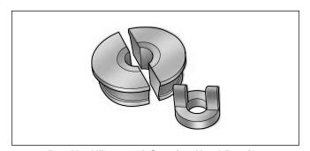
Part No. HD-39301A Steering Head Bearing Race Remover. Use with HD-33416.
