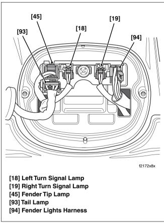
Figure 8-50. Rear Fender Lights Assembly
