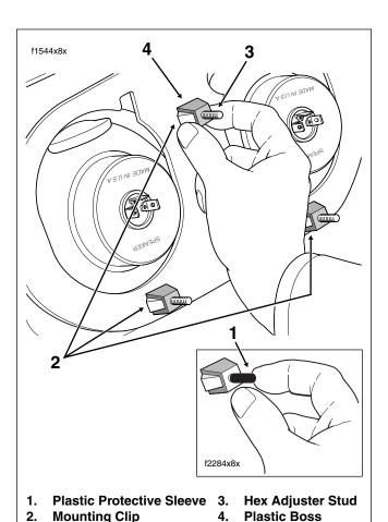
Figure 8-28. Depress Mounting Clips
