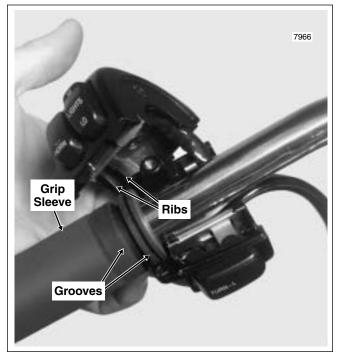
Figure 8-93. Install Left Handlebar Switch Housings
