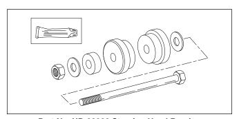
Part No. HD-39302 Steering Head Bearing Race Installer
