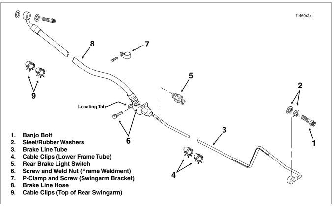
Figure 2-48. Rear Brake Line Assembly
