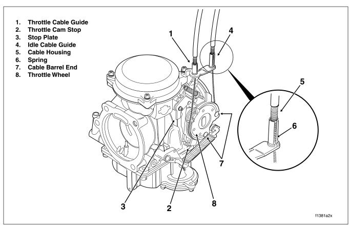
Figure 1-21. Throttle Cable Assembly - Carburetor Side
