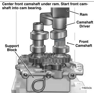
While applying pressure to front camshaft, wiggle rear camshaft to guide inner race between bearing rollers.
