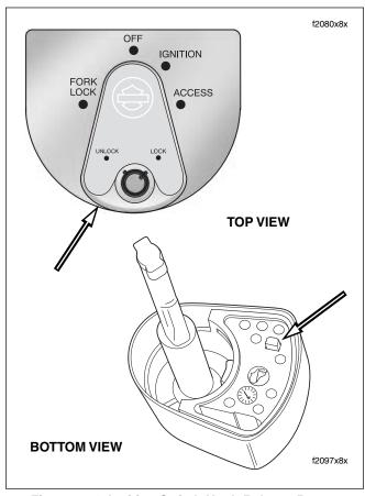
Figure 8-71. Ignition Switch Knob Release Button
