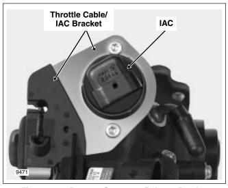
Figure 9-33. Remove Screws to Release Bracket
