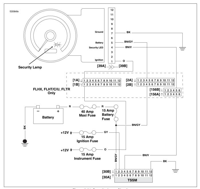
Figure 3-21. Security Lamp Circuit
