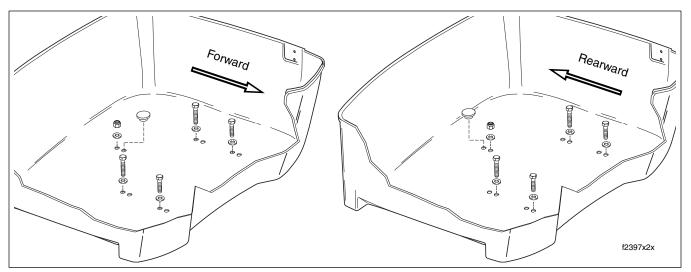
Figure 2-148. Adjust Position of Tour-Pak for Passenger Comfort
