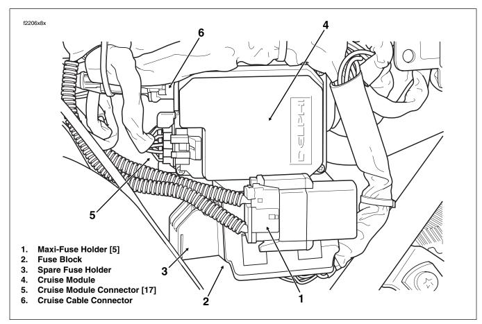
Figure 8-133. Cruise Control Module (Under Left Side Cover)
