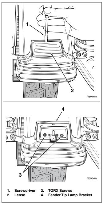
Figure 8-53. Remove Rear Fender Tip Lamp Lense and Bracket
