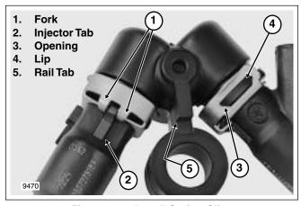
Figure 9-30. Install Spring Clips
