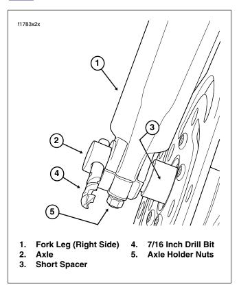
Figure 2-8. Align Front Wheel
