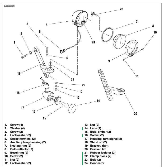
Figure 8-7. Front Turn Signal and Auxiliary Lamp Components
