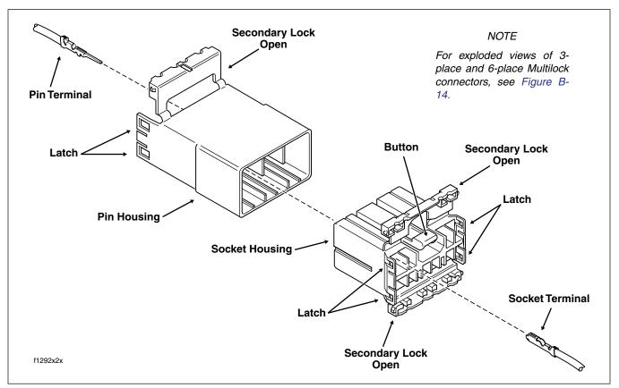
Figure B-10. 10-Place Multilock Connector (Exploded View)
