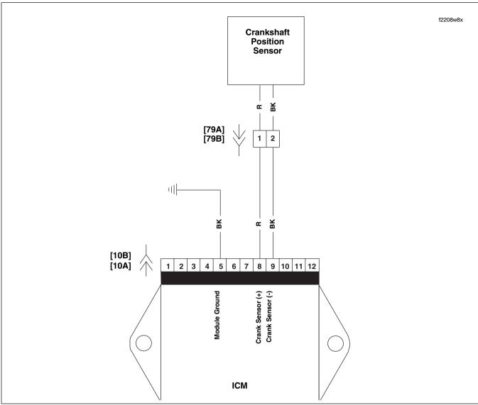
Figure 4-35. Ignition Circuit
