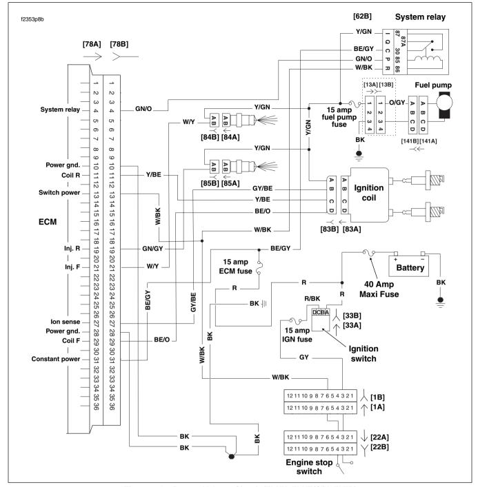
Figure 5-43. Battery Voltage Circuit (FLHX, FLHT/C/U, FLTR)
