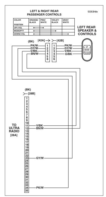
Figure 6-13. Passenger Mode Switch Circuit
