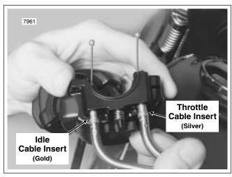
Figure 8-88. Install Throttle/Idle Control Cables in Lower Switch Housing
