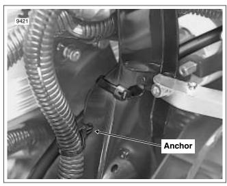
Figure 8-174. Anchor Convoluted Tubing of Headlamp Connector
