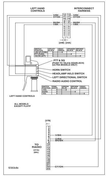
Figure 6-8. Handlebar PTT/Squelch Switch Circuit
