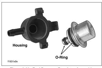
Figure 9-20. Fuel Pressure Regulator Assembly
