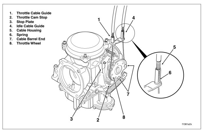
Figure 2-107. Throttle Cable Assembly - Carburetor Side
