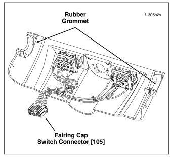
Figure 2-163. Fairing Cap Assembly (FLHX, FLHT/C/U)
