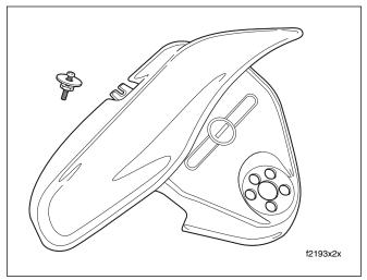
Figure 2-187. Handlebar Clamp Shroud/Wind Deflector and Screw Assembly
