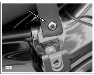
Figure 2-132. Seat Strap Bracket Screw (FLHT/C/U)
