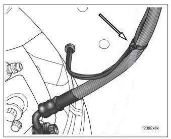
Figure 8-51. Install Cable Strap to Brake Hose
