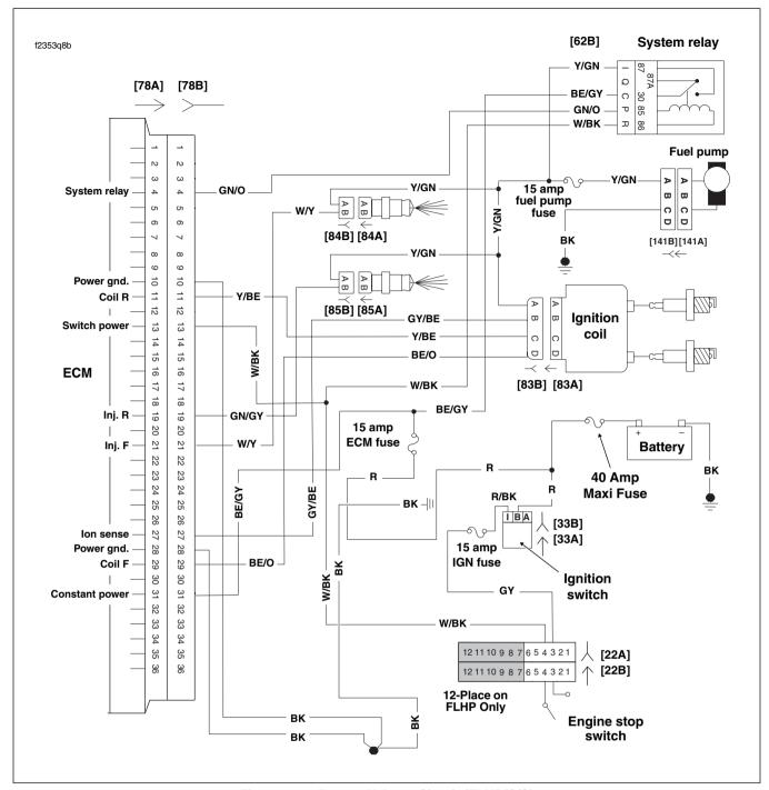
Figure 5-52. Battery Voltage Circuit (FLHR/C/S)
