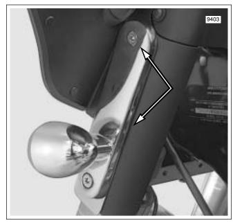
Figure 8-62. Front Turn Signal Lamp (FLHX)
