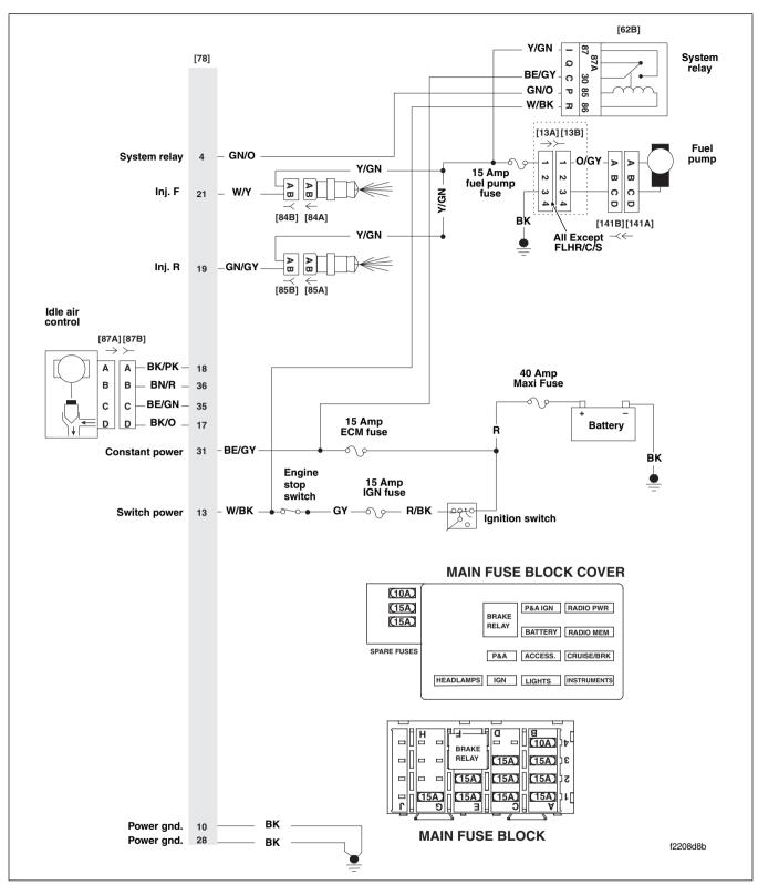
Figure 5-27. Fuel Pump Circuit
