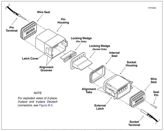
Figure B-3. 12-Place Deutsch Connector (Exploded View)
