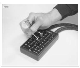
Figure 5-66. Ignition Coil Circuit Test
