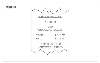
Figure 1-13. Charging System Test Results-Printout
