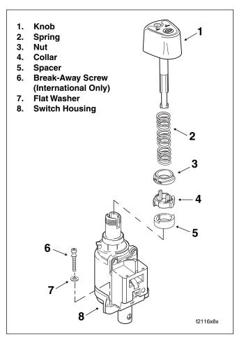
Figure 8-76. Ignition Switch Assembly (International)
