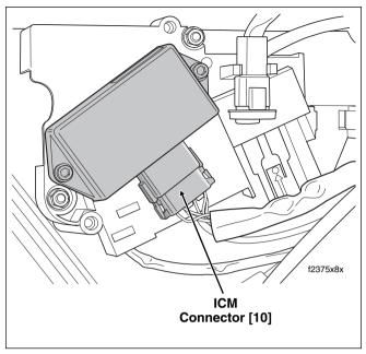
Figure 4-9. Electrical Bracket (Under Right Side Cover)
