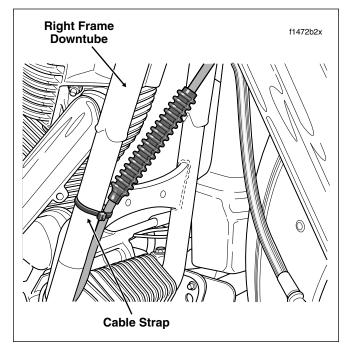
Figure 2-116. Clutch Cable Routing (Right Side View)
