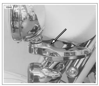
Figure 8-13. Front Turn Signal Fastener Location
