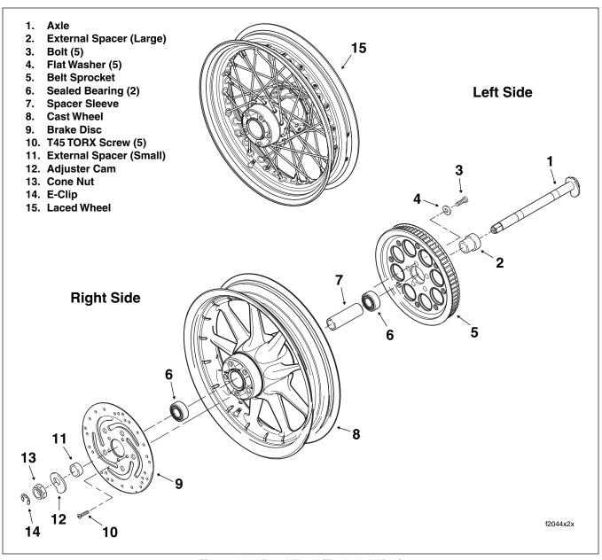
Figure 2-11. Rear Wheel (Exploded View)
