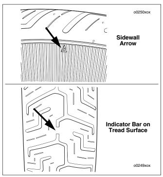
Figure 1-4. Tread Wear Indicator Bars
