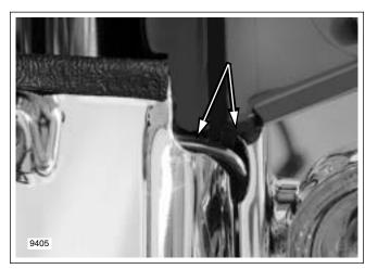
Figure 8-63. Route Conduit Thru Mounting Bracket and Chrome Skirt Reliefs (FLHX)
