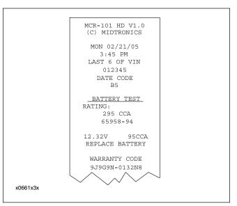
Figure 8-20. Battery Test Results-Printout
