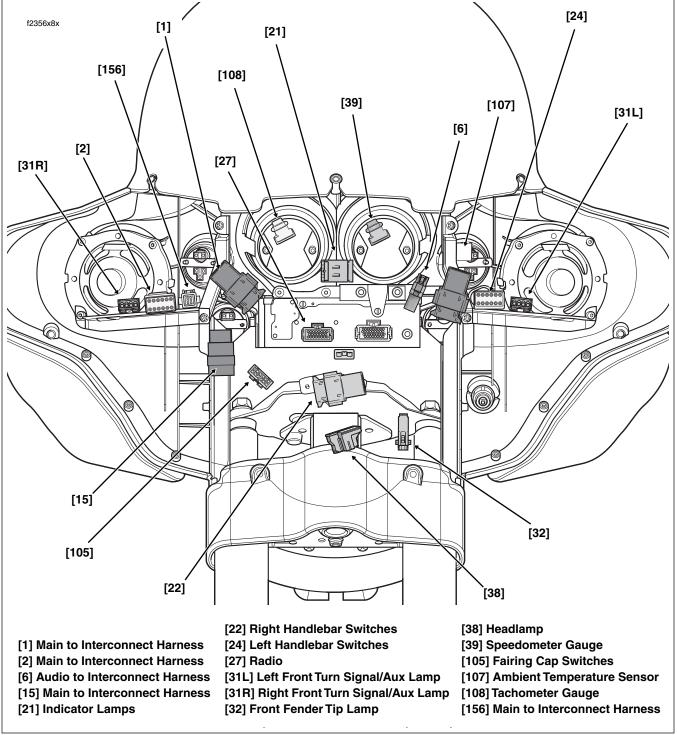
Figure 8-172. Inner Fairing - Interconnect Harness Connectors (FLHX, FLHT/C/U)
