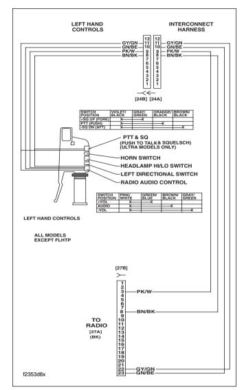
Figure 6-3. Handlebar Audio Switch Circuit
