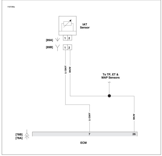
Figure 5-47. IAT Sensor Circuit
