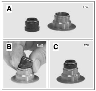
Figure 3-82. Valve Stem Seal/Spring Seat Assembly
