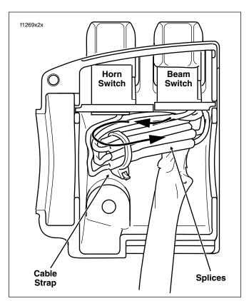
Figure 8-102. Upper Left Handlebar Switch Housing (With Splices)
