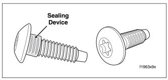
Figure 8-124. Canopy Sealing Screws
