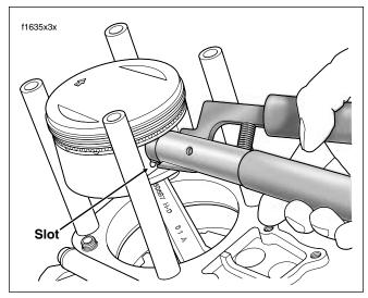
Figure 3-25. Remove Piston Pin Circlip
