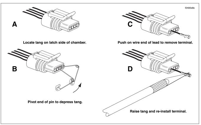
Figure B-19. Depress Tang and Extract Terminal From Mating End of Pull-to-Seat Connector
