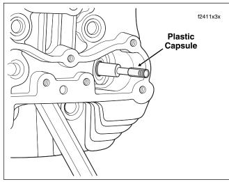
Figure 3-81. Lubricate Plastic Capsule
