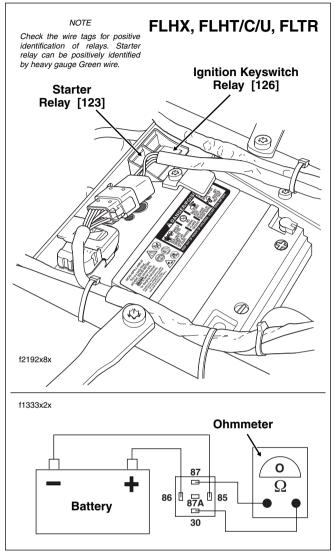
Figure 1-3. Locate Relay Under Seat
