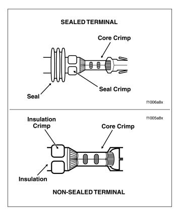
Figure B-37. Inspect Core and Insulation/Seal Crimps
