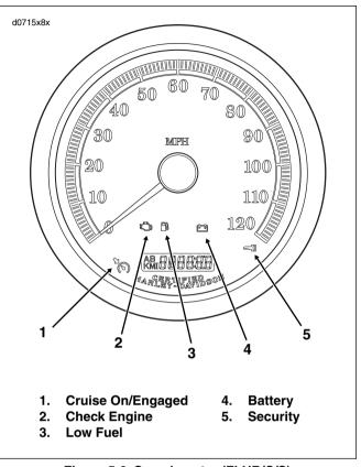
Figure 5-8. Speedometer (FLHR/C/S)
