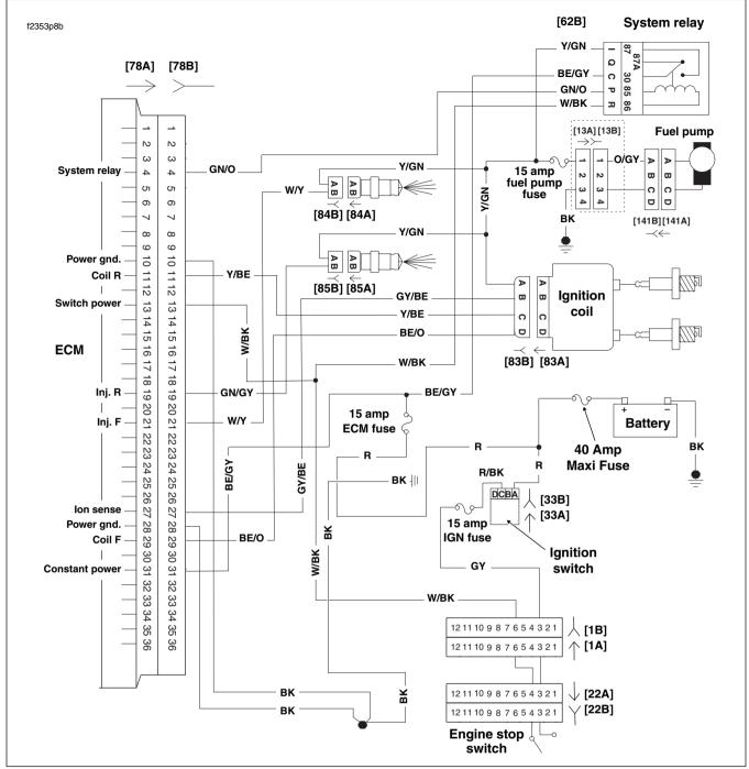
Figure 5-29. System Relay Circuit (FLHX, FLHT/C/U, FLTR)
