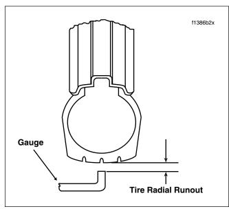
Figure 2-35. Checking Tire Radial Runout
