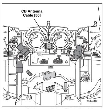
Figure 8-193. Remove Outer Fairing (FLHTCU)
