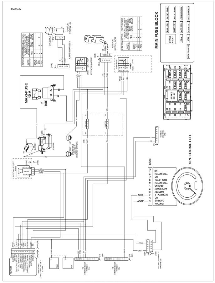
Figure 3-27. Turn Signal Circuit: FLHX, FLHT/C/U, FLTR
