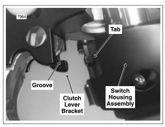
Figure 8-94. Fit Clutch Lever Bracket to Left Handlebar Switch Housings
