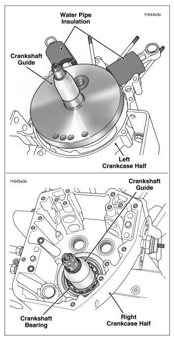
Figure 3-45. Install Crankshaft Guide to Protect Crankshaft Bearing
