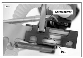
Figure 9-21. Either Crack Webbing or Depress Pin to Remove Hinge From Support Arm
