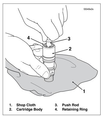
Figure 2-53. Compress Spring and Install Retaining Ring
