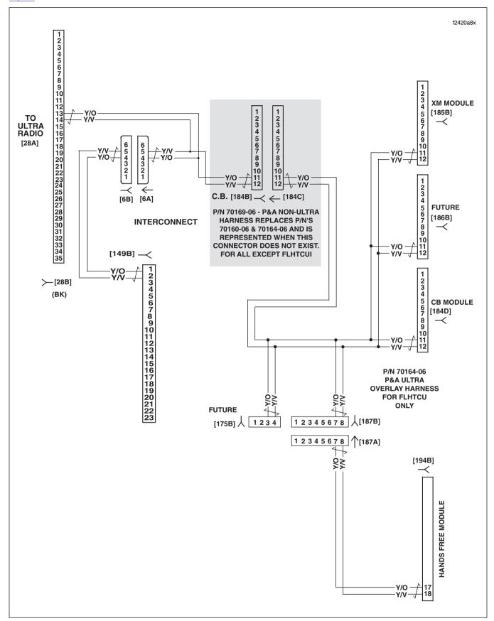
Figure 6-26. Infotainment BUS Circuit
