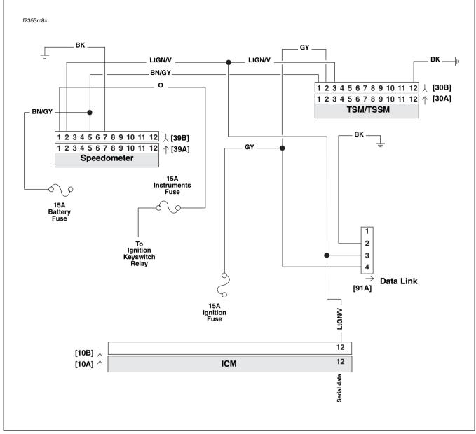
Figure 2-8. Diagnostic Check: FLHR/S (Carbureted)
