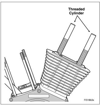
Figure 3-33. Install Threaded Cylinders to Studs (Part No. HD-95952-1)
