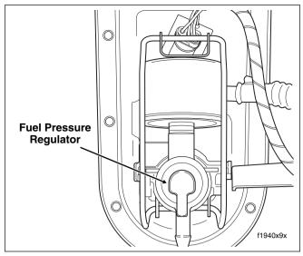
Figure 5-35. Underside of Canopy
