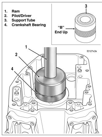
Figure 3-124. Install Crankshaft Bearing
