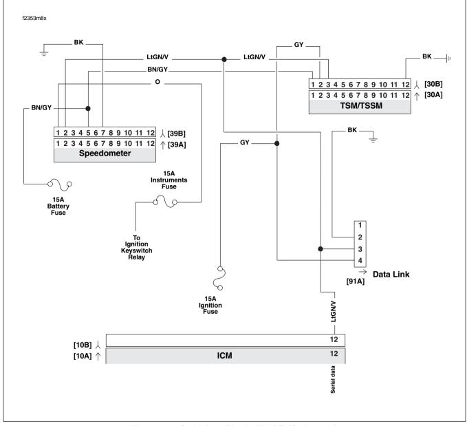
Figure 2-29. Serial Data Circuit: FLHR/S (Carbureted)
