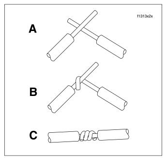
Figure 8-112. Splice Switch Wires
