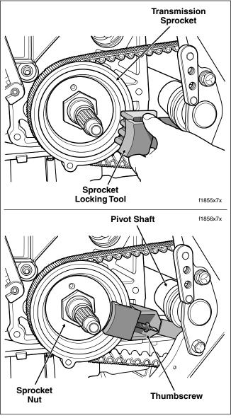
Figure 7-43. Install Final Drive Sprocket Locking Tool
