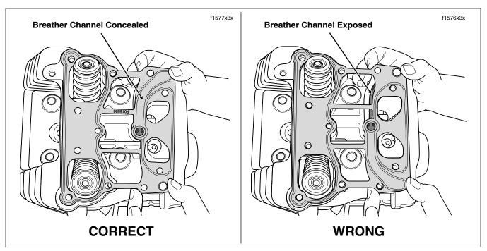
Figure 3-35. Install Rocker Housing Gasket (Rear Cylinder Shown)
