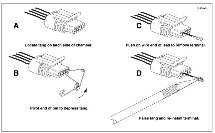
Figure 8-19. Depress Tang and Extract Terminal From Mating End of Pull-to-Seat Connector
