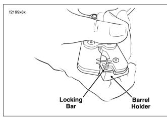
Figure 8-31. Position Contact in Crimper
