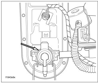
Figure 9-19. Remove Fuel Pressure Regulator (FLHR/C/S/I)
