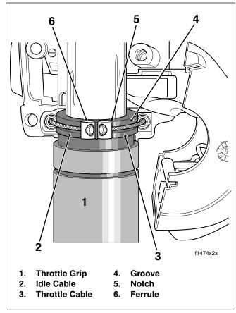
Figure 8-90. Install Throttle/Idle Cables
