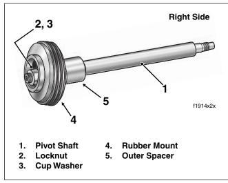
Figure 2-101. Pivot Shaft Assembly
