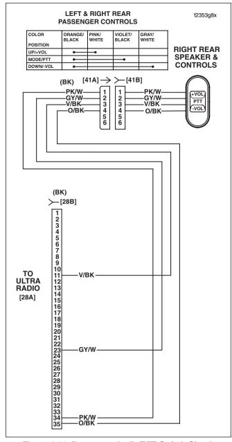
Figure 6-12. Passenger Audio/PTT Switch Circuit
