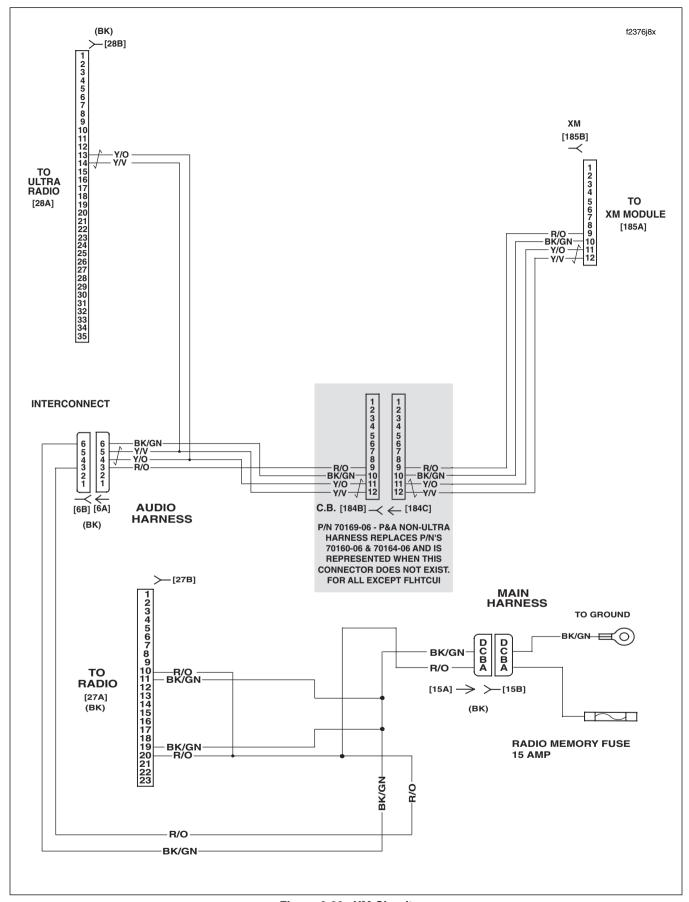
Figure 6-29. XM Circuit
