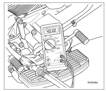
Figure 1-17. Check AC Output
