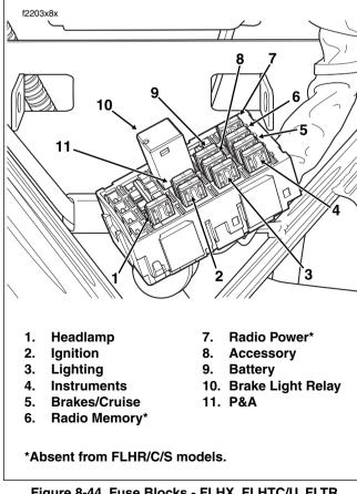
Figure 8-44. Fuse Blocks - FLHX, FLHTC/U, FLTR (Under Left Side Cover)
