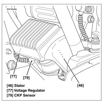
Figure 8-15. Voltage Regulator (Left Side View)
