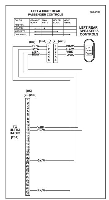
Figure 6-15. Passenger Mode Switch Circuit
