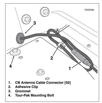
Figure 8-194. Disconnect CB Antenna Cable Connector
