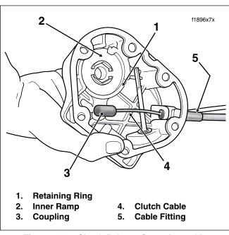
Figure 2-115. Clutch Release Cover Assembly
