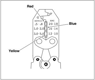
Figure B-39. Packard Crimp Tool (HD-38125-8)
