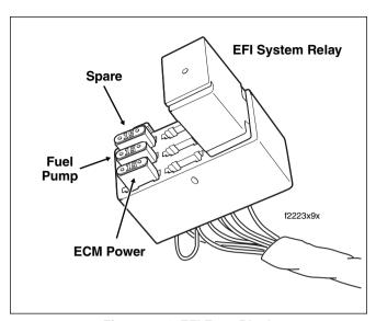
Figure 5-31. EFI Fuse Block
