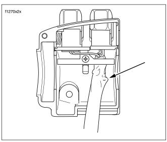
Figure 2-17. Run/Stop Switch Wiring in **Upper Right Hand Control Housing**
