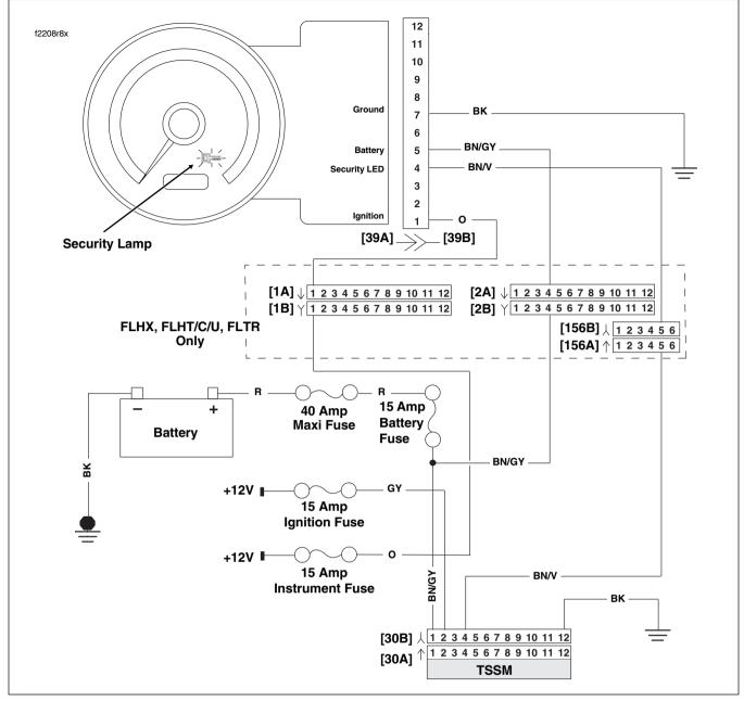
Figure 3-23. Security Lamp Circuit
