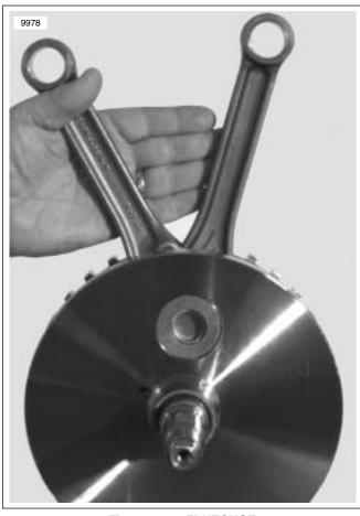
Figure 3-35. FLHTCUSE Flywheel/Connecting Rod Assembly
