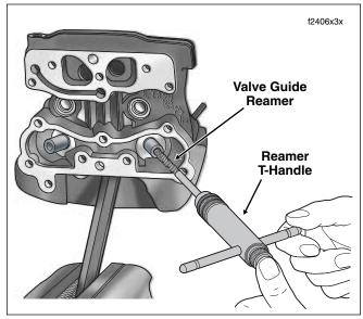
Figure 3-72. Ream Valve Guide Bore
