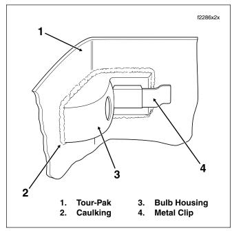
Figure 2-157. Wrap-Around Light Assembly
