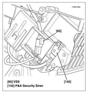
Figure 9-4. Electrical Bracket (Inboard Side)
