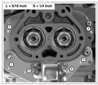
Figure 7-26. Side Door Screw Size and Torque Sequence
