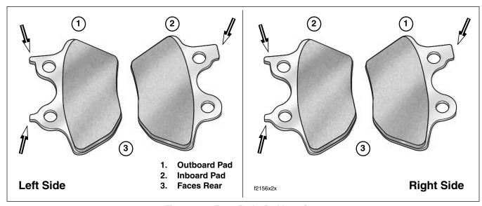
Figure 2-58. Front Brake Pad Locations
