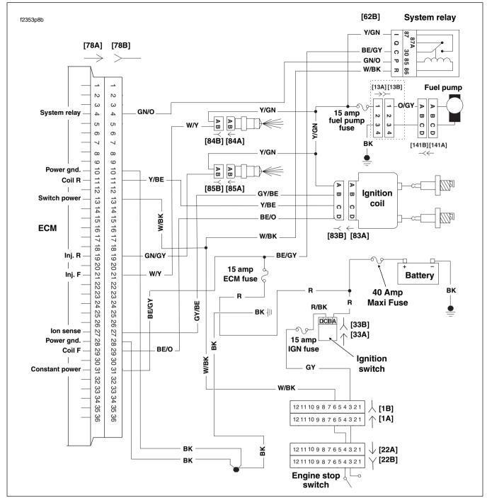
Figure 5-68. Battery Voltage Circuit (FLHX, FLHT/C/U, FLTR)
