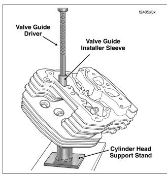
Figure 3-70. Install Valve Guide
