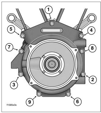
Figure 3-46. Crankcase Torque Sequence (Left Side View)
