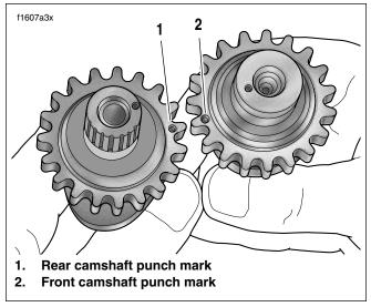
Figure 3-34. FLHTCUSE Cam Timing Marks
