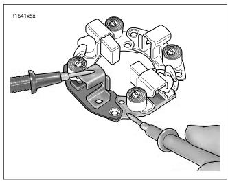
Figure 5-16. Brush Holder Insulation Test
