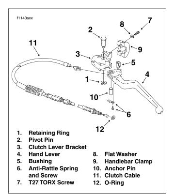
Figure 2-114. Clutch Hand Lever Assembly
