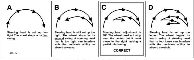
Figure 2-84. Check Steering Head Bearing Swing-By
