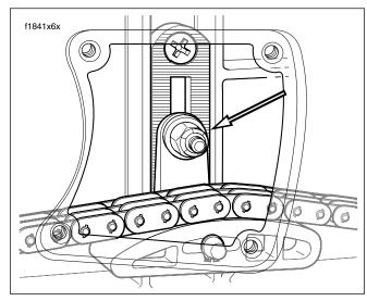
Figure 1-6. Primary Chain Tensioner Assembly
