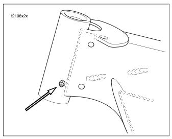
Figure 2-83. Steering Head Bearing Grease Fitting
