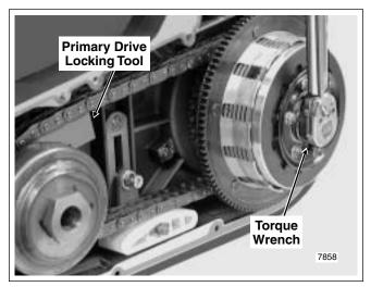
Figure 6-31. Place Primary Drive Locking Tool and Torque Clutch Hub Mainshaft Nut
