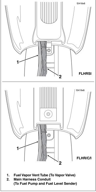
Figure 9-13. Console Cable/Hose Routing (FLHR/C/S/I)
