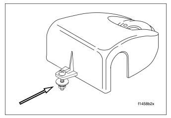
Figure 2-185. Handlebar Clamp Shroud and Screw Assembly
