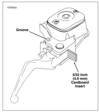
Figure 8-91. Leave Cardboard Insert in Place
