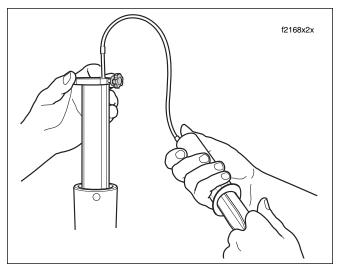
Figure 2-80. Remove Excess Fork Oil
