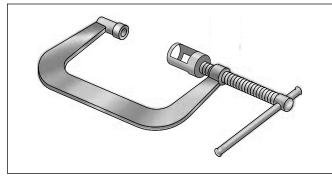
Figure 3-65. Valve Spring Compressor (Part No. HD-34736B)
