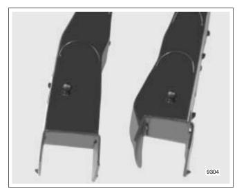
Figure 8-154. Rear Leg Index Pins
