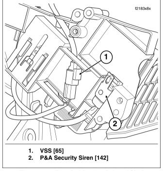
Figure 5-57. Electrical Bracket (Inboard Side)
