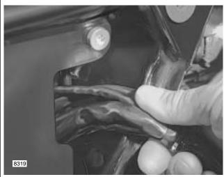
Figure 8-162. Remove Main Harness From Vehicle
