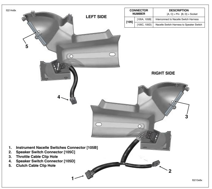
Figure 2-178. Instrument Nacelle Halves
