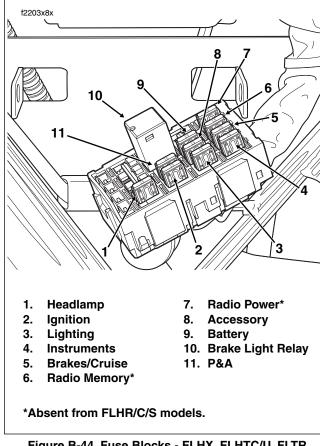
Figure B-44. Fuse Blocks - FLHX, FLHTC/U, FLTR (Under Left Side Cover)
