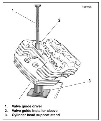
Figure 3-16. Install Valve Guide
