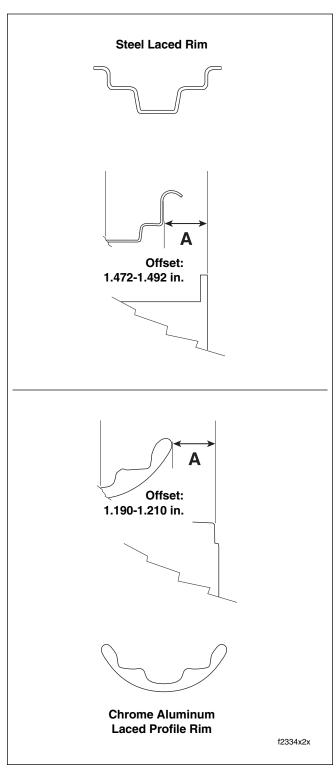
Figure 2-30. Laced Hub Offset Dimension (16 Inch Rear)
