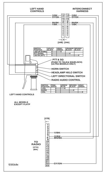
Figure 6-11. Handlebar PTT/Squelch Switch Circuit
