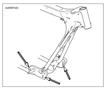
Figure 2-3. Footboard Position Adjustment Holes
