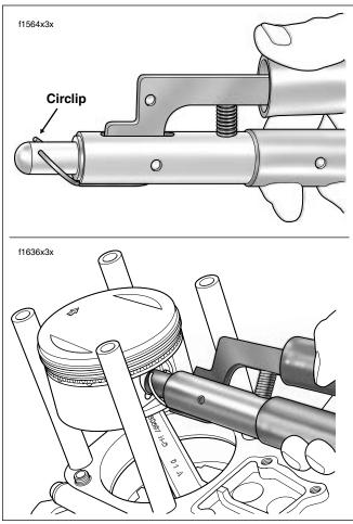
Figure 3-28. Install Piston Pin Circlip
