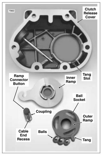
Figure 7-14. Clutch Release Cover Assembly
