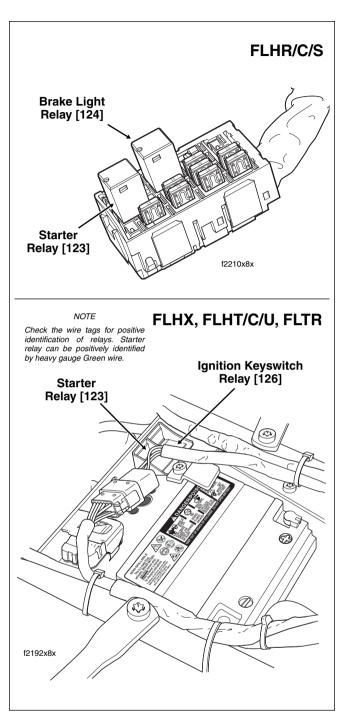
Figure 3-34. Locate Starter Relay
