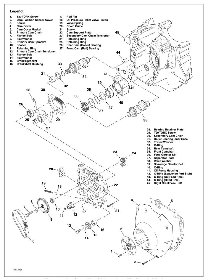
Figure 3-99. Cam Support Plate/Oil Pump Assemblies (Exploded View)
