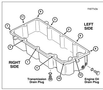
Figure 3-16. Oil Pan Torque Sequence
