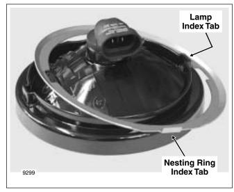
Figure 8-33. Auxiliary Lamp Assembly
