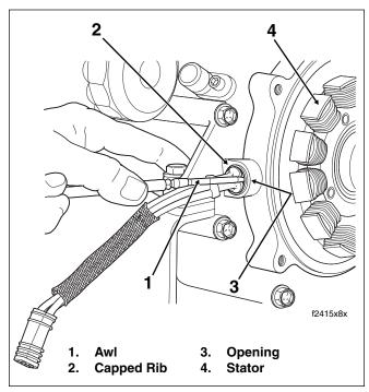
Figure 3-14. Remove Grommet From Crankcase
