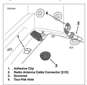
Figure 8-182. Feed Main Harness Thru Tour-Pak Hole
