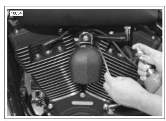
Figure 4-14. Checking for Leaks
