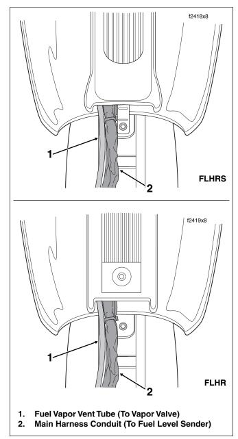
Figure 4-19. Console Cable/Hose Routing (FLHR/S)
