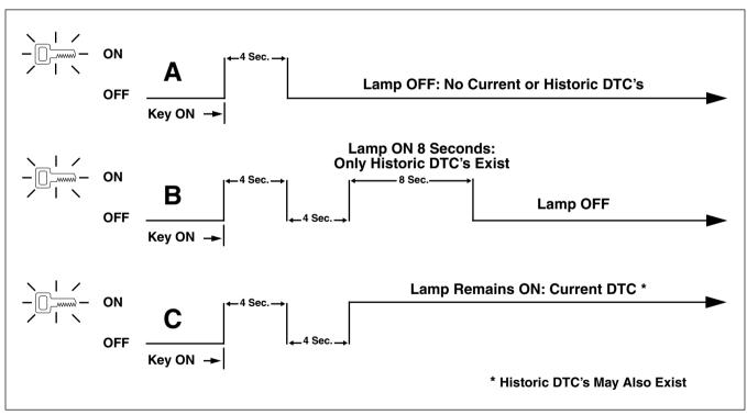
Figure 2-3. Check Engine and Security Lamp Operation
