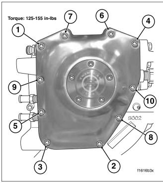
Figure 3-55. Cam Cover Torque Sequence
