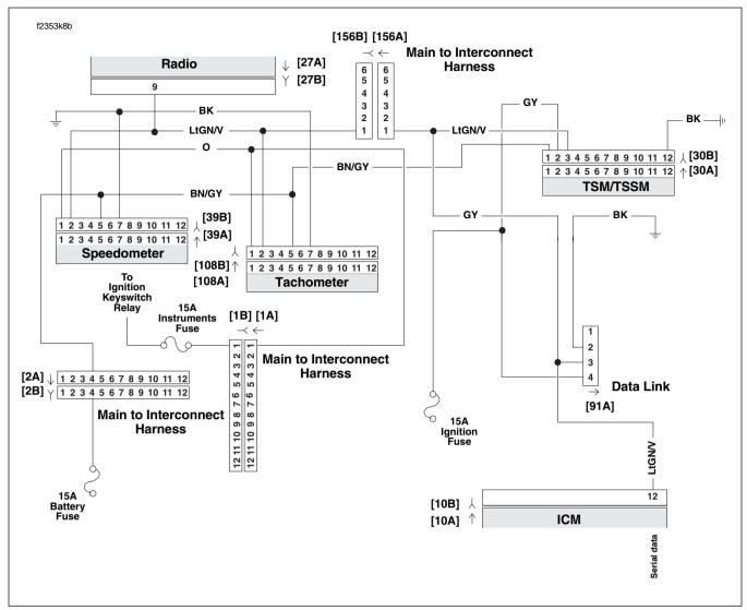
Figure 4-45. Serial Data Circuit (FLHX, FLHT/C)
