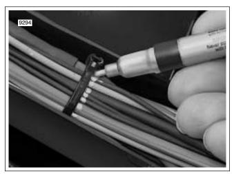
Figure 8-151. Mark Location of Cable Straps
