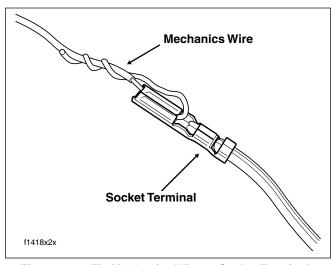
Figure 8-38. Fix Mechanics Wire to Socket Terminals
