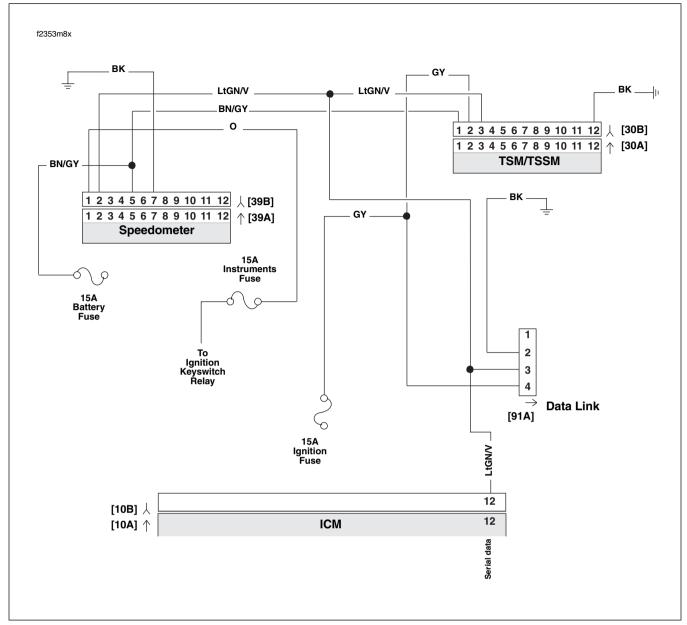
Figure 4-30. Serial Data Circuit (FLHR/S)
