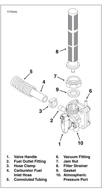
Figure 4-14. Vacuum Operated Fuel Valve
