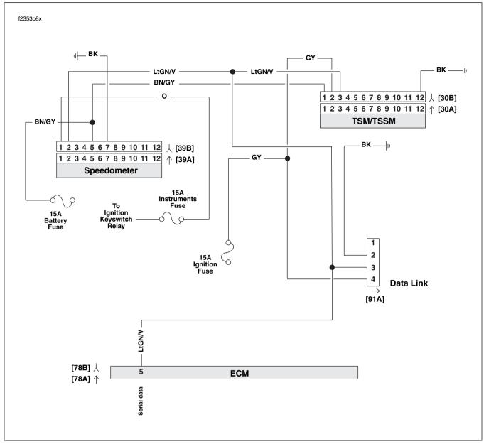
Figure 3-50. Serial Data Circuit: FLHR/C/S (Fuel Injected)
