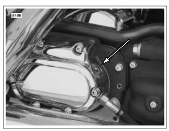
Figure 1-11. Clutch Release Cover
