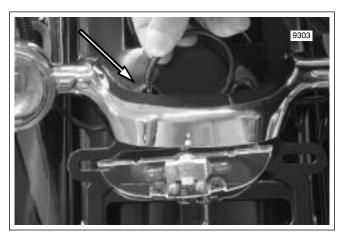
Figure 8-68. Draw Wires Through Fender Hole
