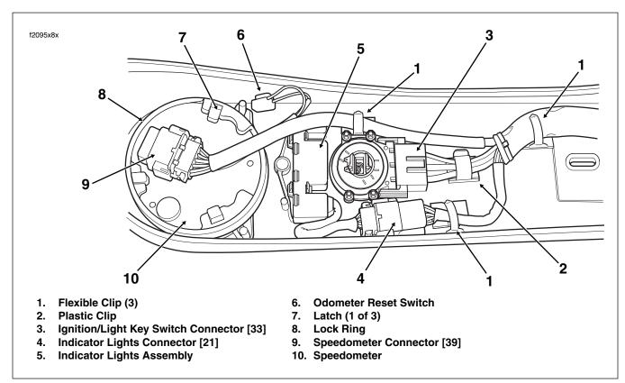
Figure 8-122. Instrument Console Assembly (FLHR/C)
