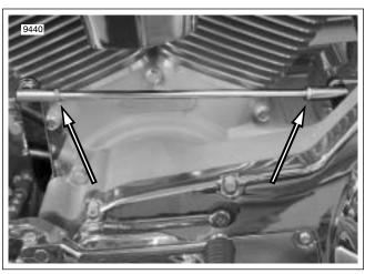
Figure 7-2. Loosen Locknuts and Adjust Rod
