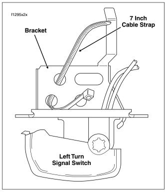
Figure 8-110. Insert Cable Strap in Switch Bracket
