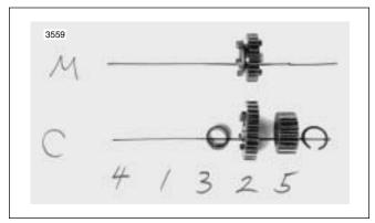
Figure 7-20. Note Gear Location During Disassembly
