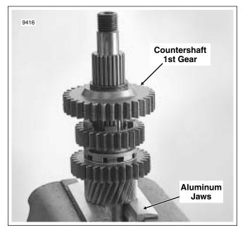
Figure D-4. Disassemble/Assemble Countershaft
