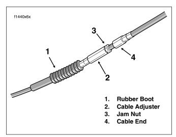
Figure 2-113. Clutch Cable Adjuster Mechanism
