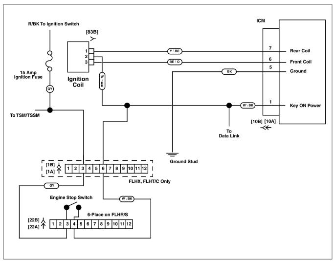
Figure 4-23. Ignition Coil Circuit
