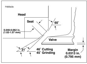
Figure 3-26. Valve Seat Angles
