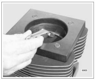
Figure 3-89. Measure Ring End Gap
