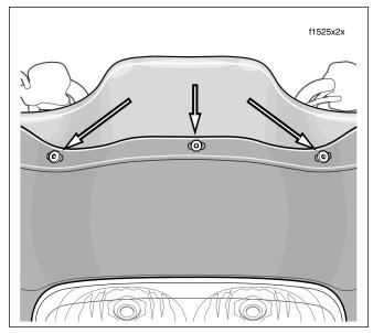
Figure 2-171. Remove Wellnuts From Outer Fairing
