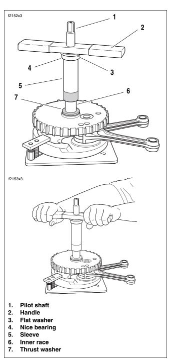
Figure 3-39. Press Inner Race Onto Sprocket Shaft
