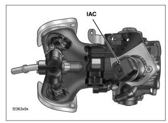
Figure 5-37. Induction Module (Top View)
