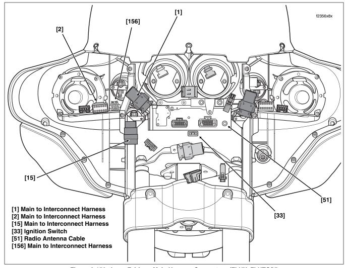
Figure 8-158. Inner Fairing - Main Harness Connectors (FLHX, FLHTC/U)
