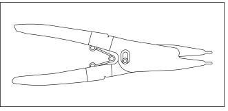
Part No. HD-96216-49 Large Internal **Retaining Ring Pliers**
