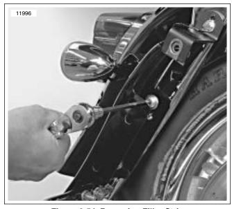
Figure 2-54. Removing Filler Strip
