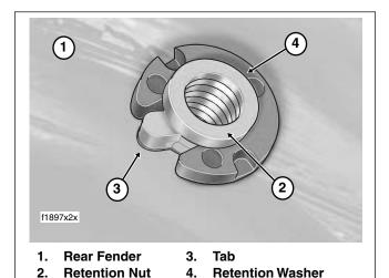
Figure 2-133. Seat Retention Nut and Washer
