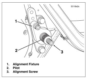
Figure 2-38. Install Vehicle Alignment Tool (Left Side)
