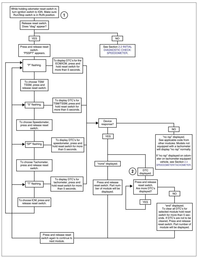
Figure 2-13. Speedometer Self Diagnostics
