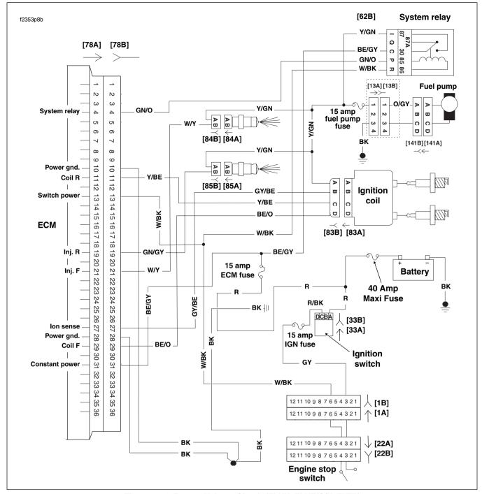
Figure 5-51. Battery Voltage Circuit (FLHX, FLHT/C/U, FLTR)
