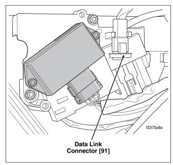
Figure 4-18. Electrical Bracket (Under Right Side Cover)
