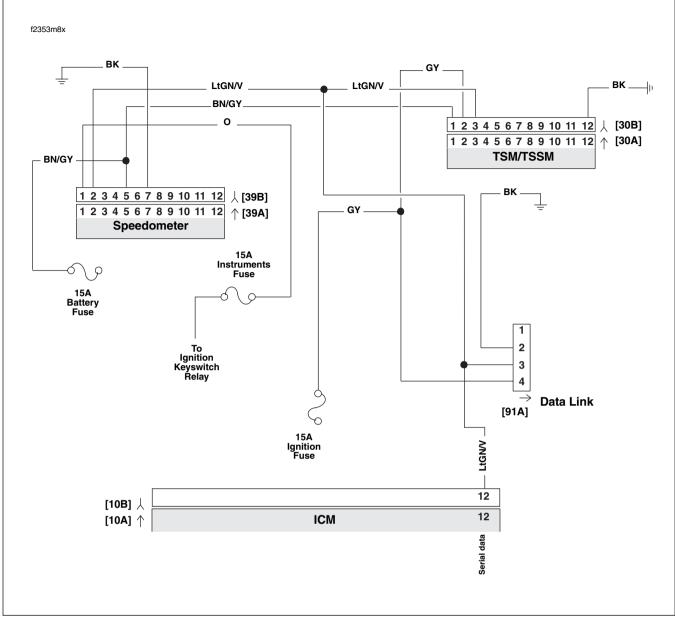
Figure 2-35. Serial Data Circuit: FLHR/S (Carbureted)
