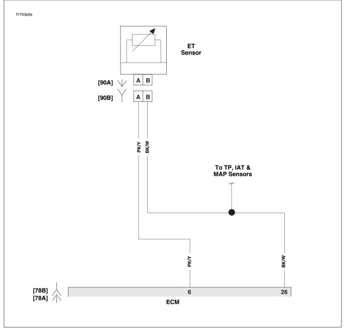
Figure 5-48. ET Sensor Circuit
