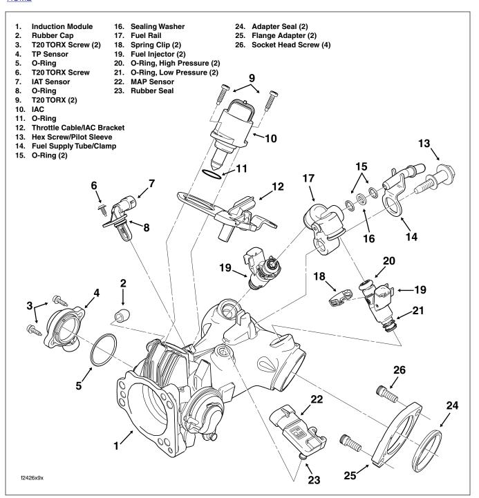
Figure 9-35. Induction Module Assembly
