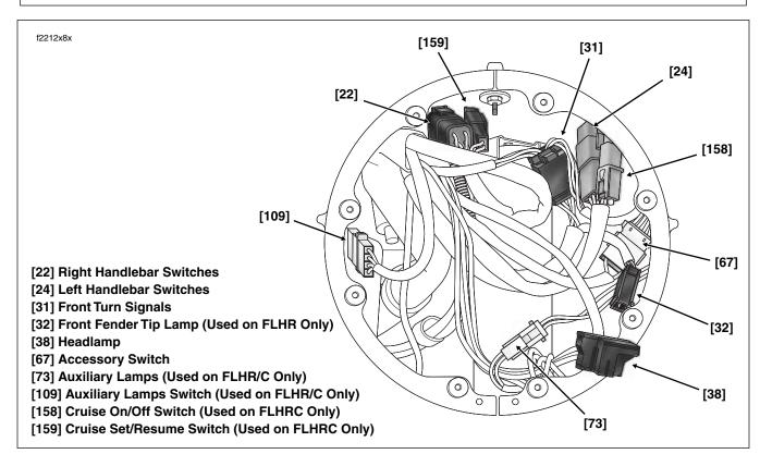
Figure B-55. Headlamp Nacelle Connectors (FLHR/C/S)
