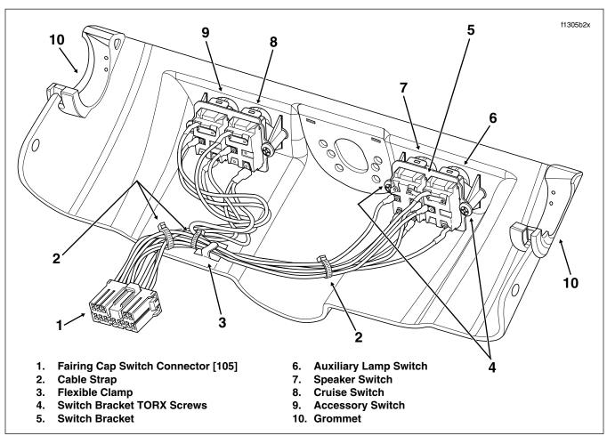
Figure 8-80. Fairing Cap (Inboard Side) - Ultra Model Shown
