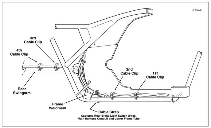
Figure 2-49. Rear Brake Line Routing (Right Side View)
