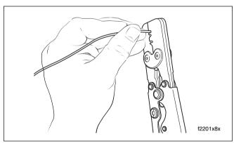
Figure 8-32. Crimp Terminal Onto Wire
