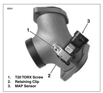
Figure 8-7. Intake Manifold
