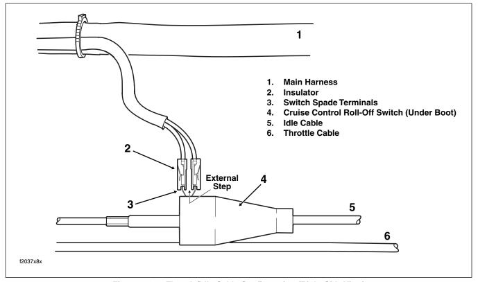
Figure 8-132. Throttle/Idle Cable Configuration (Right Side View)
