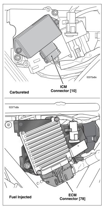
Figure 3-40. Electrical Bracket (Under Right Side Cover)
