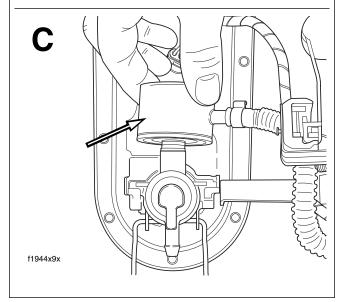
Figure 9-18. Remove Fuel Filter Canister (FLHR/C/S/I)
