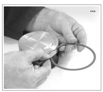
Figure 3-86. Measure Piston Ring Side Clearance
