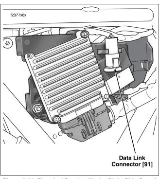
Figure 5-62. Electrical Bracket (Under Right Side Cover)
