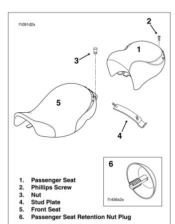
Figure 2-129. Seat Assembly - FLHR
