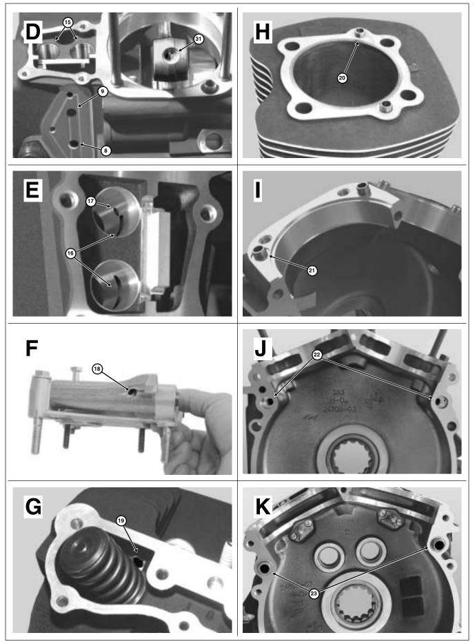
Figure 3-7. Engine Oil Flow - Top End
