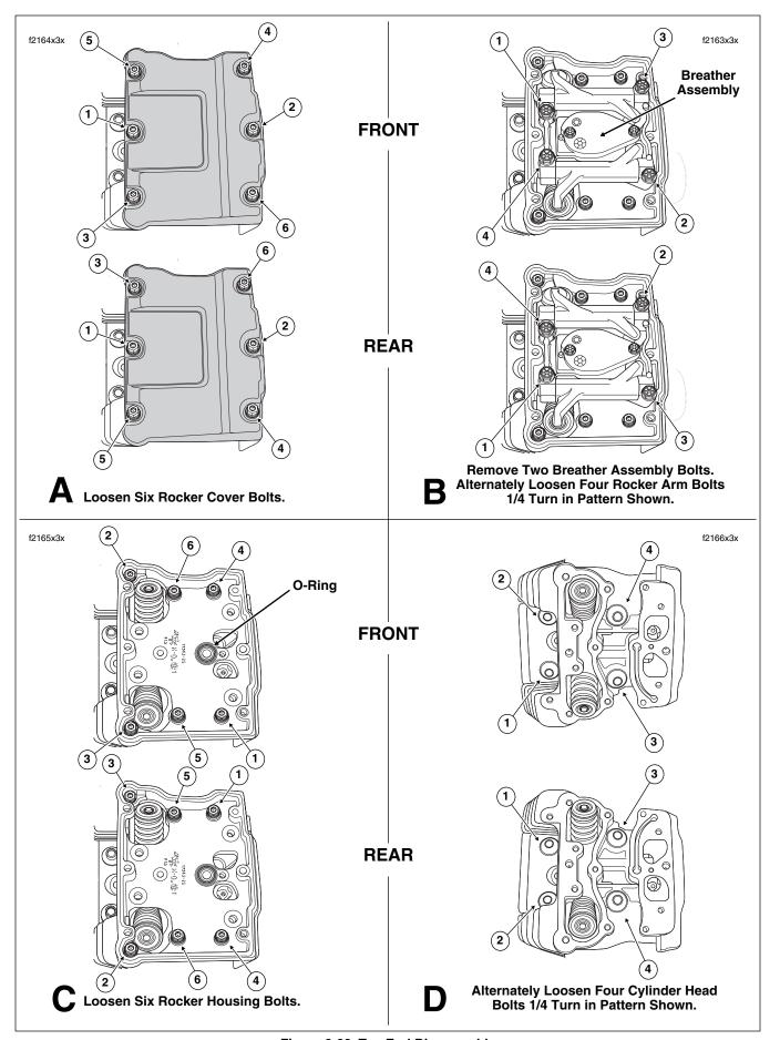
Figure 3-22. Top End Disassembly
