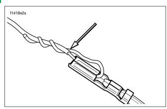
Figure 8-8. Fix Mechanic's Wire to Socket Terminals
