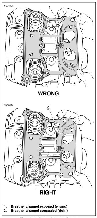
Figure 3-2. Rocker Housing Gasket
