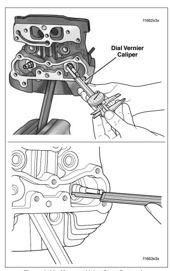
Figure 3-23. Measure Valve Stem Protrusion
