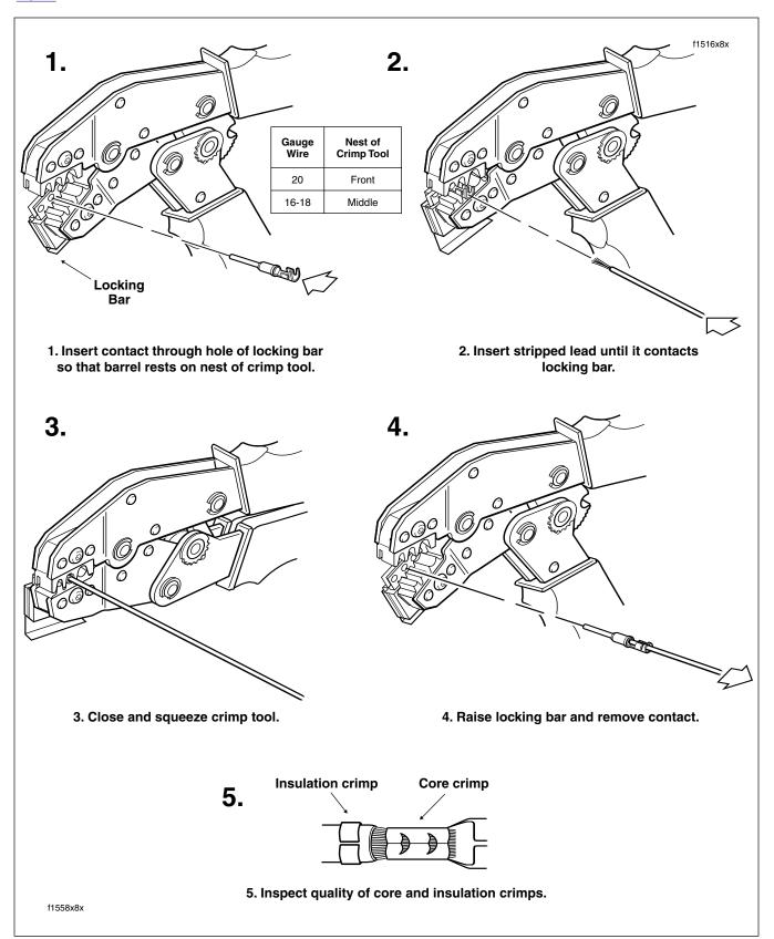
Figure B-7. Deutsch Crimping Procedure
