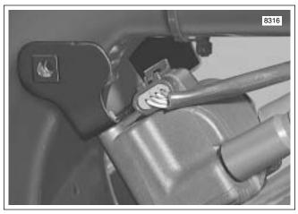
Figure 3-11. Remove Ignition Coil Bracket
