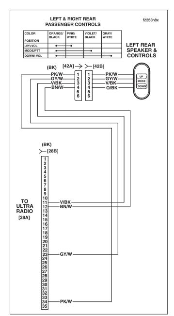
Figure 6-17. Passenger Mode Switch Circuit
