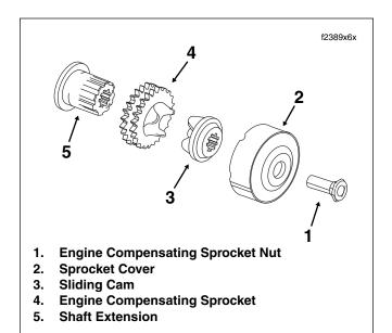
Figure 6-19. Engine Compensating Sprocket Assembly
