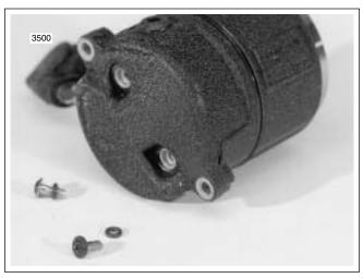
Figure 5-7. Remove End Cap Screws and O-Rings
