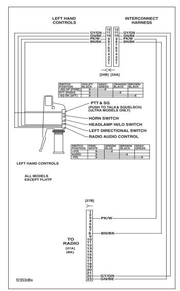
Figure 6-9. Handlebar Audio Switch Circuit
