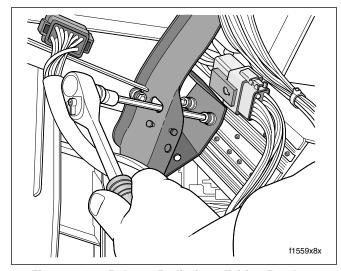
Figure 8-159. Release Radio from Fairing Brackets (FLHTC/U)
