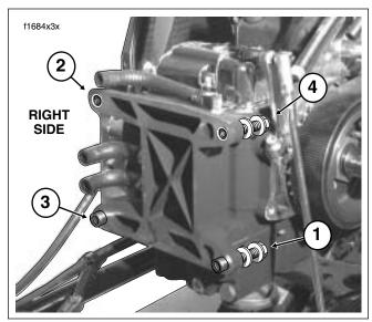
Figure 3-17. Transmission Housing to Crankcase Torque Sequence
