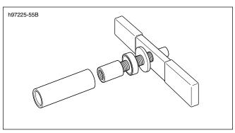
Figure 3-38. Sprocket Shaft Timken Bearing Cone Installer (Part No. HD-97225-55B)
