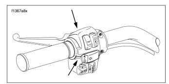
Figure 2-23. Left Handlebar Switch Housing Screws
