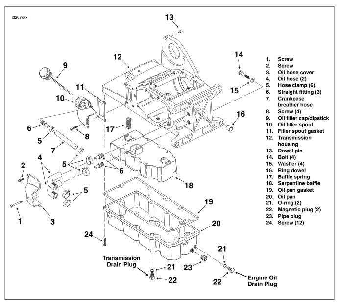
Figure 7-49. Transmission Case and Oil Pan
