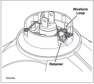
Figure 8-25. Headlamp Bulb Assembly
