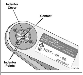
Insert bare wire strands into contact barrel. Squeeze handle of crimp tool until tightly closed.
