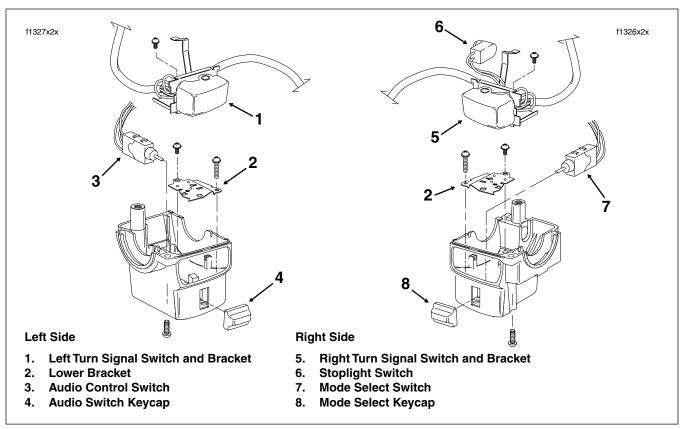
Figure 8-107. Lower Handlebar Switch Assemblies (Classic)
