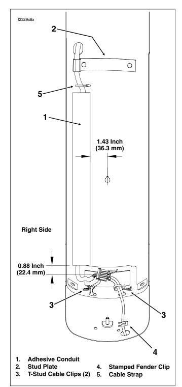
Figure 8-44. Rear Fender Well
