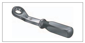
Figure 3-23. Engine Rotation Wrench (Part No. HD-47257)
