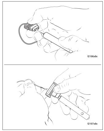
Figure B-28. Insert Tool and Remove Terminal
