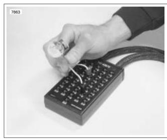
Figure 5-17. Ignition Coil Circuit Test
