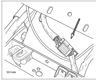
Figure 2-190. Rear Fender Lights Connector [7]
