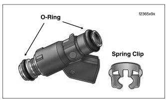
Figure 9-29. Fuel Injector Assembly
