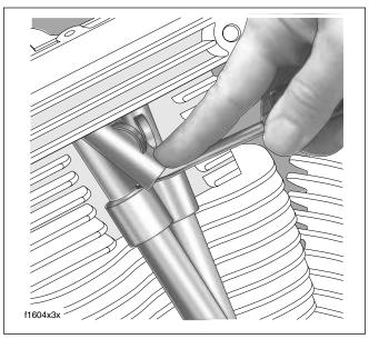
Figure 3-39. Install Spring Cap Retainer
