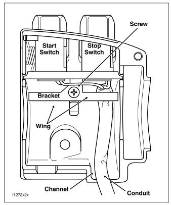
Figure 8-99. Upper Right Handlebar Switch Housing (Without Splices)
