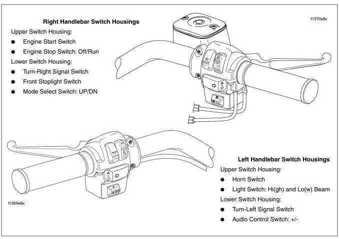
Figure 8-97. Classic Handlebar Switch Assemblies
