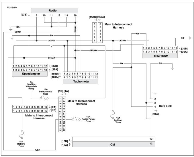
Figure 6-24. Serial Data Circuit: FLHX, FLHT/C (Carbureted)
