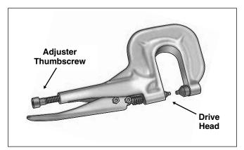
Figure 2-152. Rivet Tool (HD-39787A)
