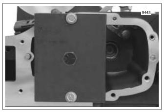
Figure 7-29. Main Drive Gear Removal (Right Side)
