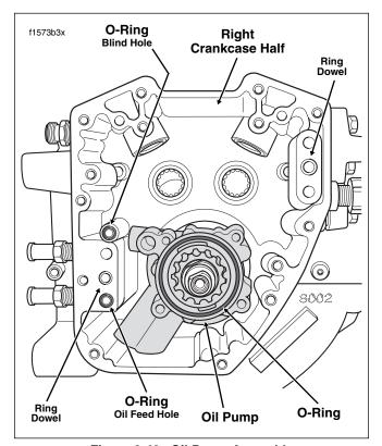
Figure 3-43. Oil Pump Assembly
