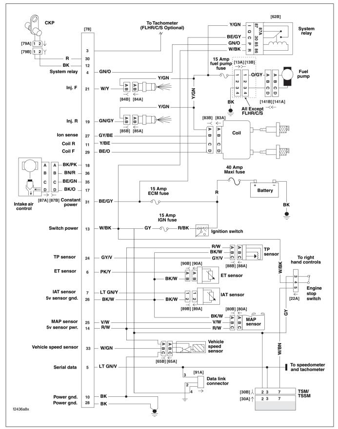
Figure 5-18. Simplified EFI System Circuit
