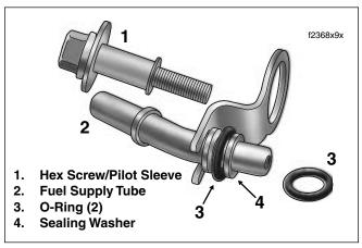
Figure 9-28. Fuel Supply Tube Assembly
