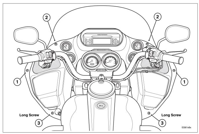
Figure 2-173. Remove/Install Six Outer Fairing Screws
