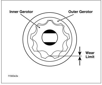
Figure 3-120. Measure Gerotor Sets for Wear
