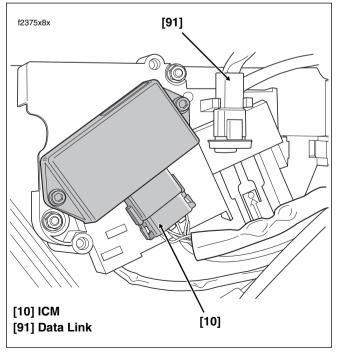
Figure 8-48. Under Right Side Cover (Carbureted)
