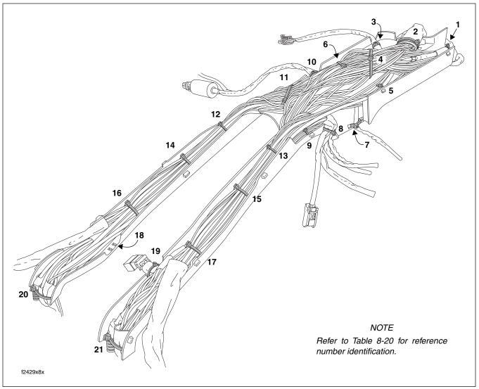
Figure 8-155. Wire Trough Cable Strap Locations (FLHTCU)
