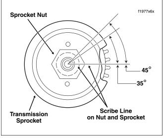
Figure 7-46. Tighten/Secure Sprocket Nut
