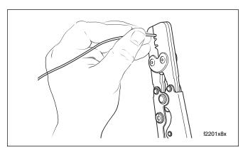
Figure B-32. Crimp Terminal Onto Wire
