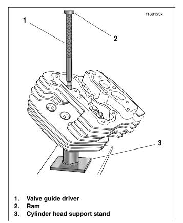
Figure 3-14. Remove Valve Guide
