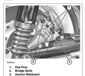
Figure 2-65. Loosen Both Pad Pins
