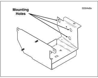
Figure 8-137. Battery Box (Right Side View)
