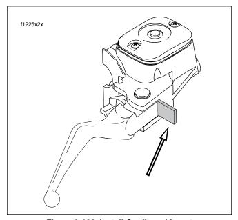
Figure 2-108. Install Cardboard Insert
