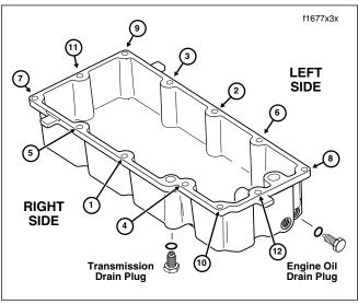
Figure 7-52. Oil Pan Torque Sequence
