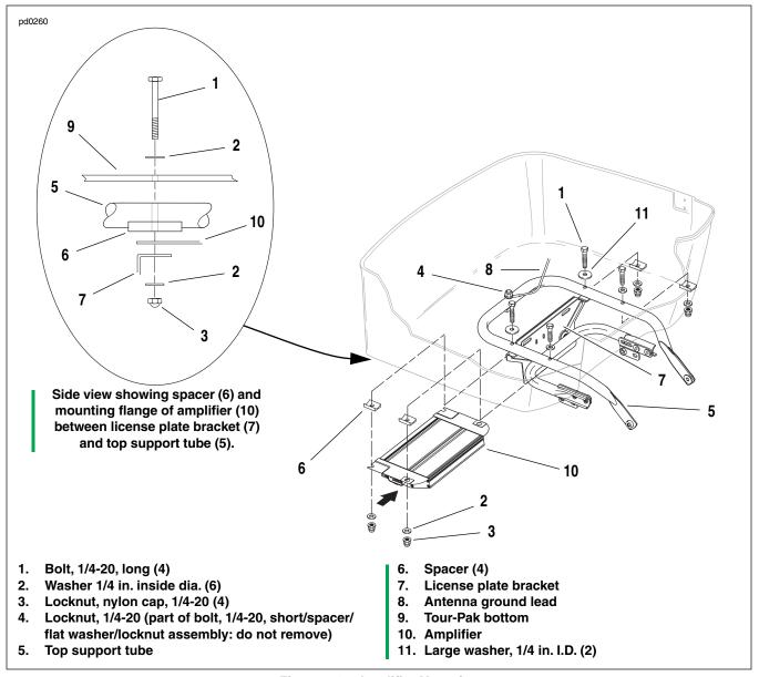
Figure 8-19. Amplifier Mounting
