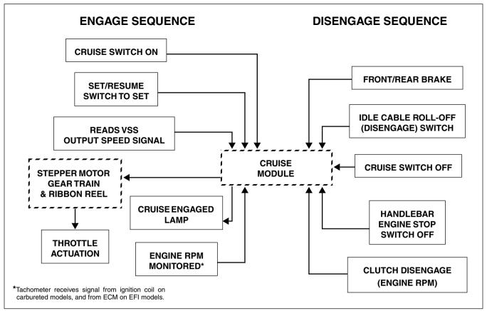
Figure 7-4. Cruise System Diagram
