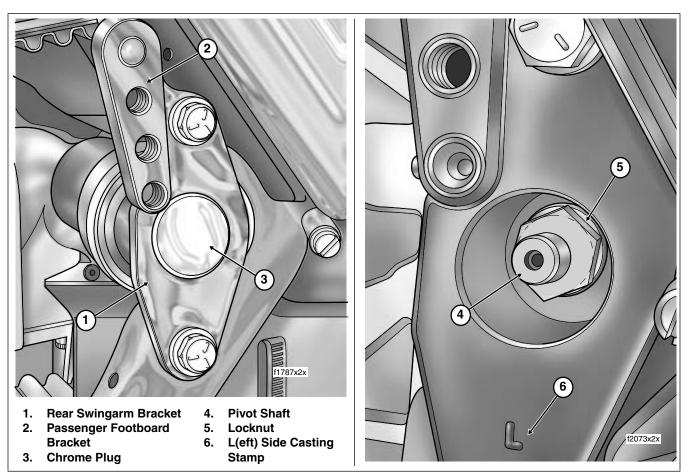
Figure 2-105. Remove Chrome Plugs and Check Pivot Shaft Locknut Torque (Left Side View)
