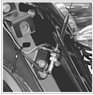
Figure 8-186. Capture Radio Antenna Cable (FLHX)
