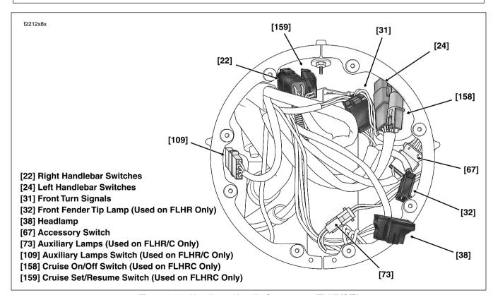
Figure 8-55. Headlamp Nacelle Connectors (FLHR/C/S)
