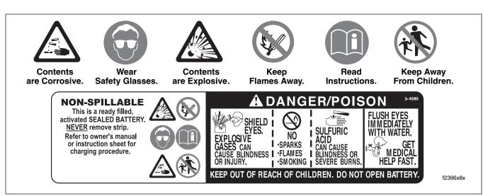
Figure 8-18. Battery Warning Label
