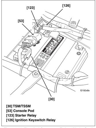
Figure 8-52. Electrical Connectors/Relays (Under Seat)
