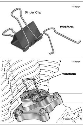
Figure 3-100. Fashion Tool to Hold Hydraulic Lifters
