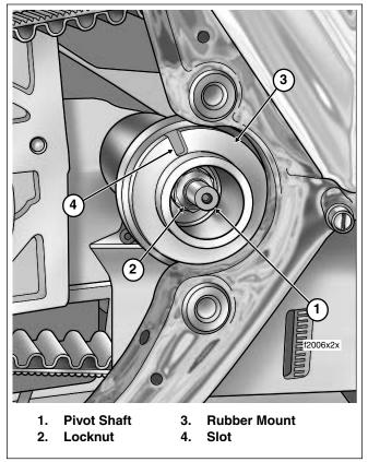
Figure 2-96. Remove Rear Swingarm Bracket (Left Side View)
