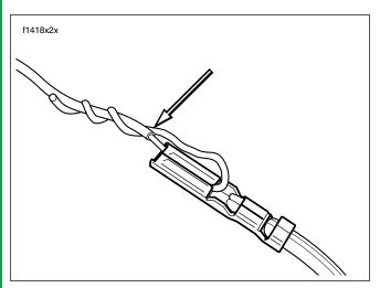
Figure 8-14. Fix Mechanic's Wire to Socket Terminals
