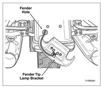
Figure 8-54. Feed Fender Tip Lamp Socket and Conduit
