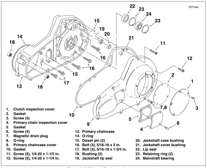
Figure 6-27. Primary Chaincase Assembly
