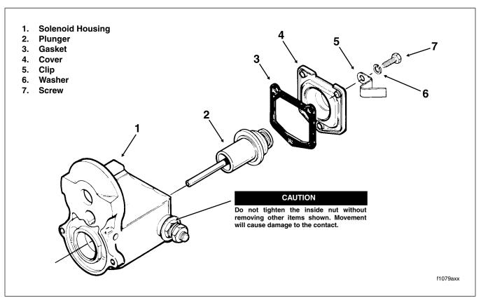
Figure 5-20. Starter Solenoid
