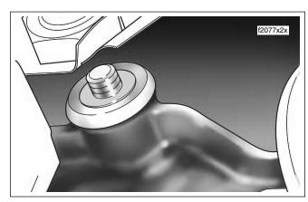
Figure 2-122. Remove Flat Washer and Upper Cup Washer (Right Side)
