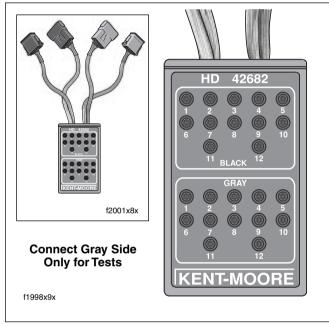
Figure 3-18. Breakout Box (Part No. HD-42682)
