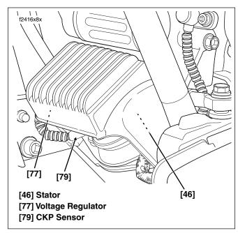
Figure 9-5. Voltage Regulator (Left Side View)
