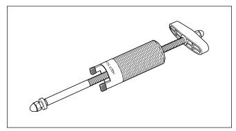
Figure 3-26. Piston Pin Remover (Part No. HD-42320A)
