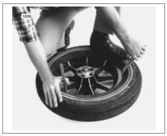
Figure 2-34. Starting Second Bead on Rim
