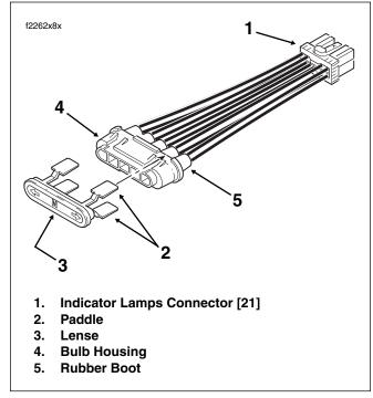
Figure 2-167. Indicator Lamp Assembly
