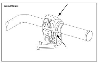
Figure 2-11. Right Handlebar Switch Housing Screws
