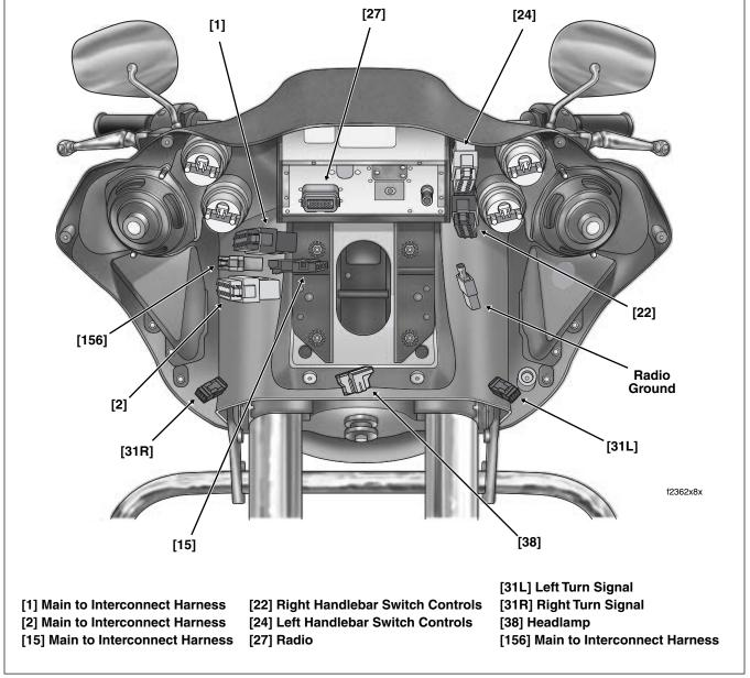
Figure 8-177. Inner Fairing - Interconnect Harness Connectors (FLTR)
