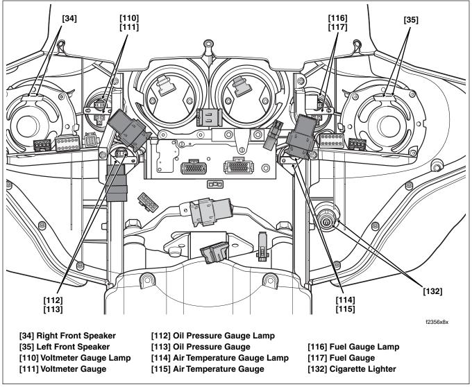
Figure 8-173. Inner Fairing - Interconnect Harness Connectors (FLHX, FLHTC/U)
