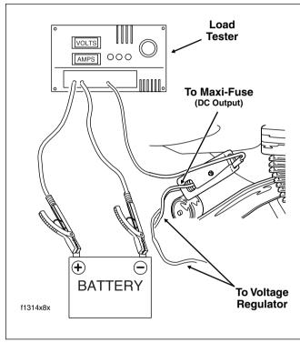
Figure 1-14. Current and Voltage Output Test
