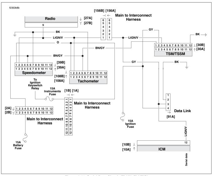
Figure 4-41. Serial Data Circuit (FLHX, FLHT/C)
