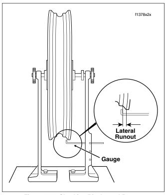
Figure 2-16. Checking Rim Lateral Runout
