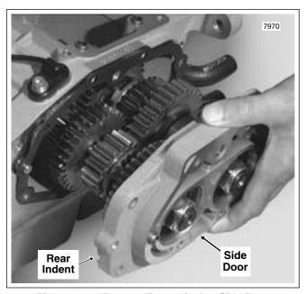
Figure 7-19. Remove Transmission Side Door
