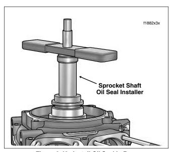
Figure 3-48. Install Oil Seal In Bore
