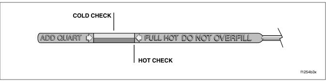
Figure 1-2. Engine Oil Dipstick
