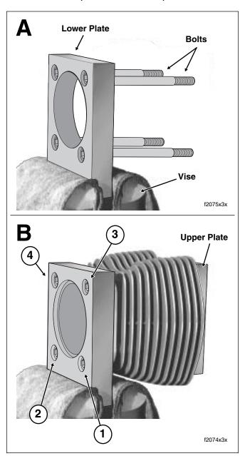
Figure 3-84. Install Cylinder to Torque Plates
