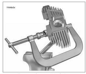
Figure 3-66. Compress Valve Springs
