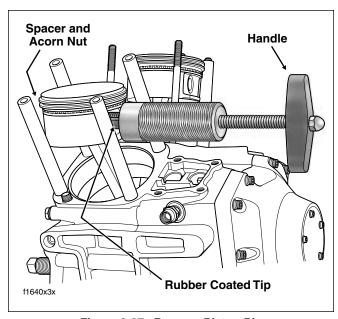
Figure 3-27. Remove Piston Pin
