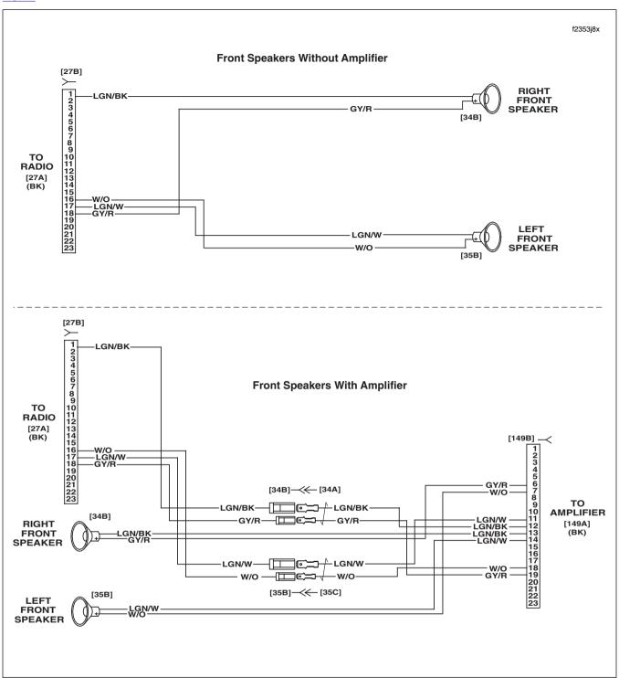
Figure 6-21. Front Speaker Circuit
