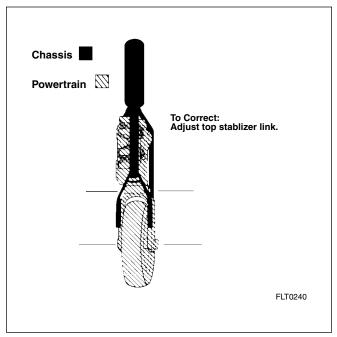
Figure 2-41. Vertically Misaligned
