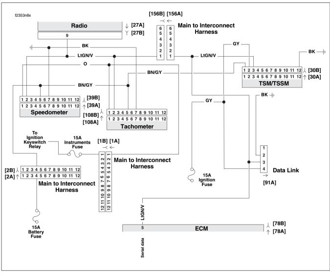
Figure 5-72. ECM and TSM/TSSM Circuit (FLHX, FLHT/C/U, FLTR)
