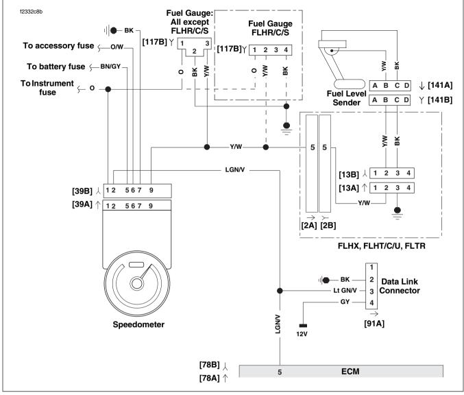
Figure 2-24. Fuel Sender Circuit
