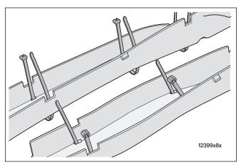
Figure 8-153. Install New Cable Straps in Wire Trough
