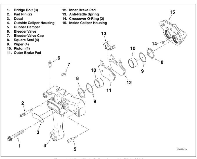
Figure 2-67. Rear Brake Caliper Assembly (Right Side)
