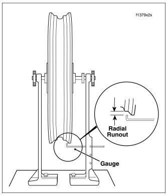
Figure 2-17. Checking Rim Radial Runout
