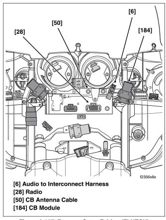
Figure 8-187. Remove Outer Fairing (FLHTCU)
