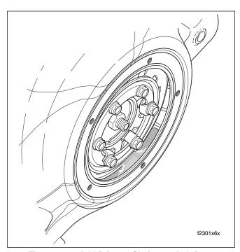
Figure 6-33. Add Primary Chaincase Lubricant
