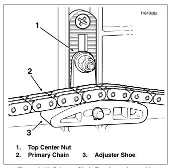
Figure 6-15. Primary Chain Tensioner Assembly
