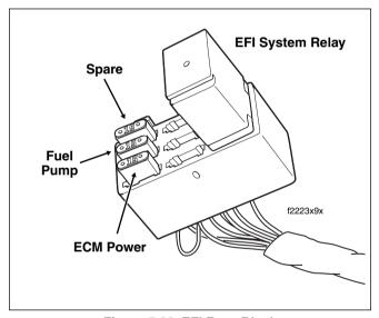
Figure 5-26. EFI Fuse Block
