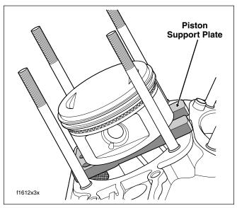
Figure 3-30. Install Piston Support Plate
