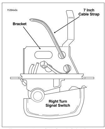
Figure 8-105. Insert Cable Strap in Switch Bracket
