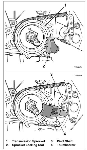
Figure 6-11. Install Final Drive Sprocket Locking Tool
