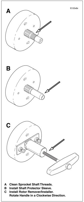
Figure 8-12. Remove Rotor from Engine Sprocket Shaft
