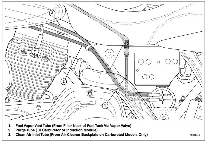
Figure 4-24. Charcoal Canister Tube/Hose Routing (Left Side View)
