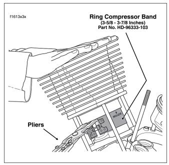
Figure 3-32. Install Cylinder
