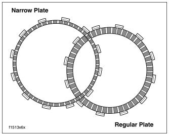
Figure 6-6. Friction Plates
