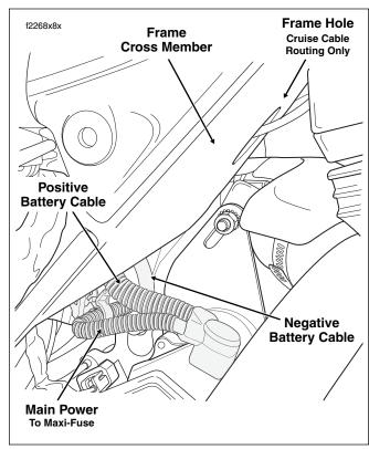
Figure 5-3. Battery Cable Routing (Right Side View)
