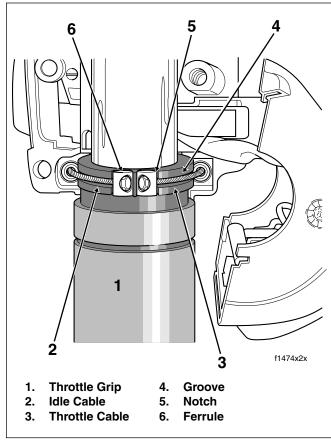
Figure 2-110. Install Throttle/Idle Cables
