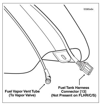
Figure 4-16. Fuel Level Sender Connector (FLHX, FLHT)
