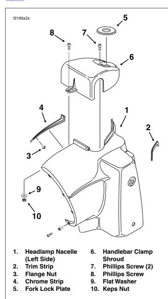
Figure 2-184. Headlamp Nacelle Assembly
