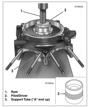
Figure 3-125. Remove Sprocket Shaft Bearing
