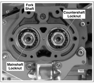
Figure 7-18. Remove Mainshaft/Countershaft Locknuts
