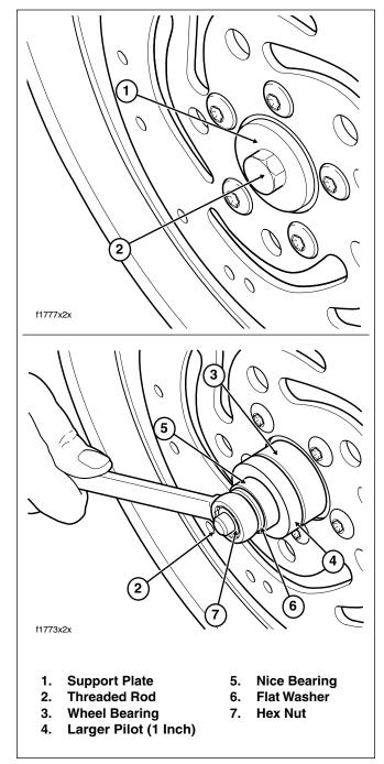
Figure 2-7. Install Sealed Wheel Bearings
