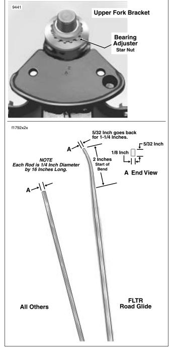
Figure 2-86. Fashion Steering Head Bearing Adjustment Tool From Drill Rod
