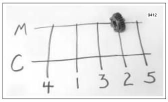
Figure D-1. Note Gear Location During Disassembly
