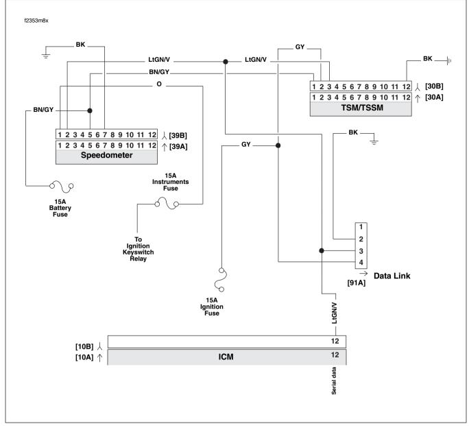
Figure 4-46. Serial Data Circuit (FLHR/S)
