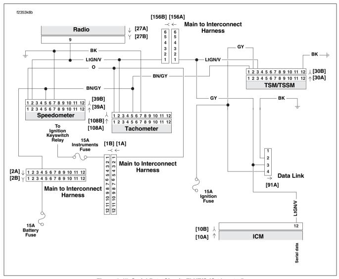
Figure 3-47. Serial Data Circuit: FLHT/C (Carbureted)
