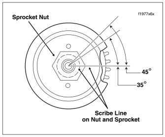
Figure 6-14. Tighten/Secure Sprocket Nut
