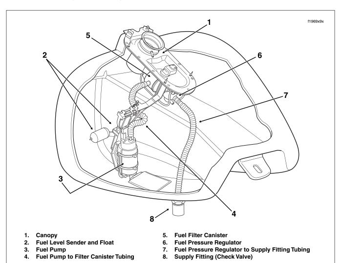
Figure 9-9. Fuel Tank Assembly (FLHXI, FLHT/C/U/I, FLTRI)
