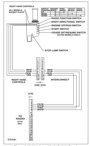
Figure 6-10. Handlebar Mode Switch Circuit
