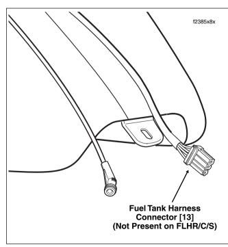
Figure 8-47. Rear of Fuel Tank (Under Seat)
