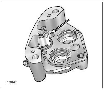
Figure 2-63. Install Anti-Rattle Spring
