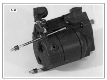
Figure 5-5. Remove Thru-Bolts
