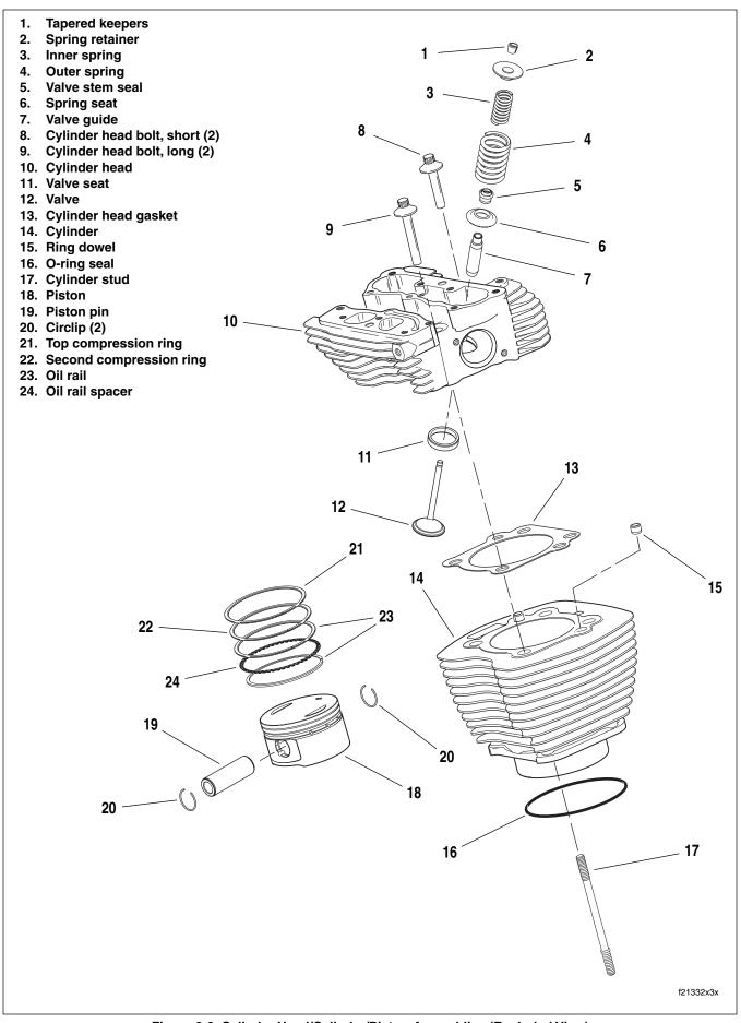
Figure 3-9. Cylinder Head/Cylinder/Piston Assemblies (Exploded View)
