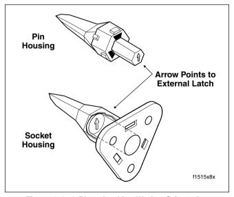
Figure 8-4. 3-Place Locking Wedge Orientation
