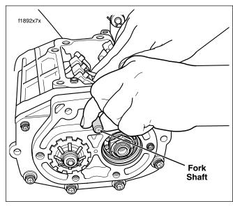
Figure 7-5. Remove Fork Shaft/Shifter Forks (Right Side View)
