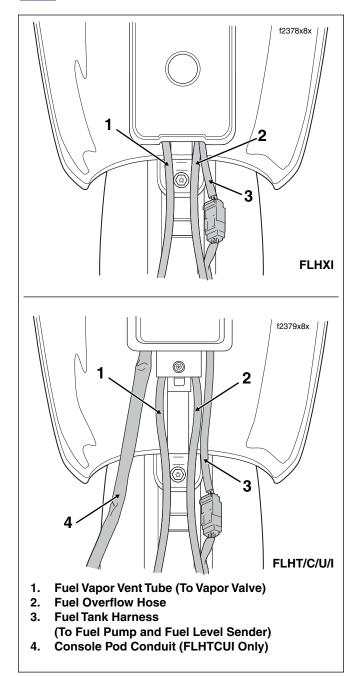
Figure 9-12. Console Cable/Hose Routing (FLHXI, FLHT/C/U/I)
