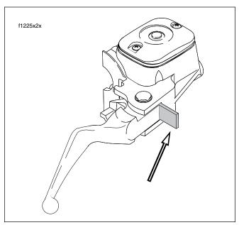
Figure 1-17. Install Cardboard Insert
