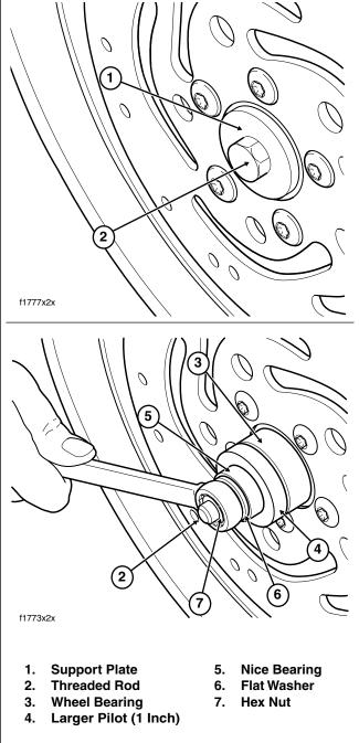
Figure 2-13. Install Sealed Wheel Bearings
