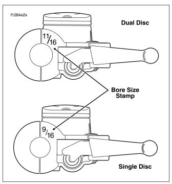
Figure 2-42. Verify Correct Bore Size Before Use
