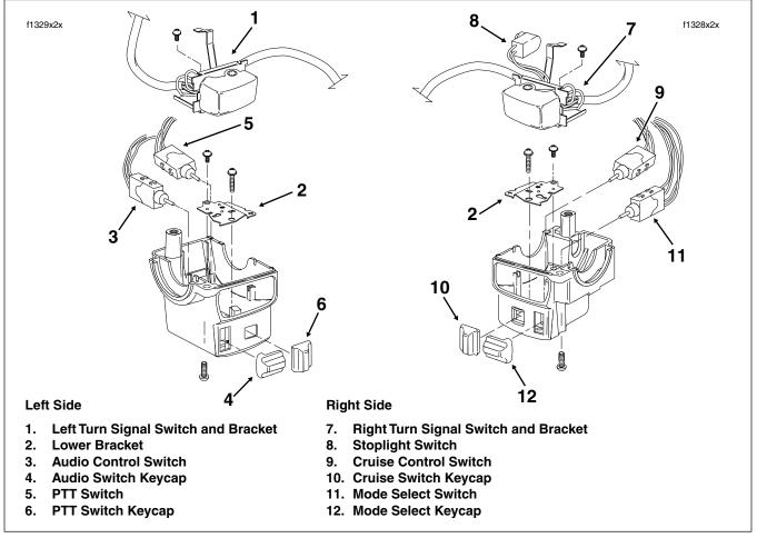
Figure 8-108. Lower Handlebar Switch Assemblies (Ultra)
