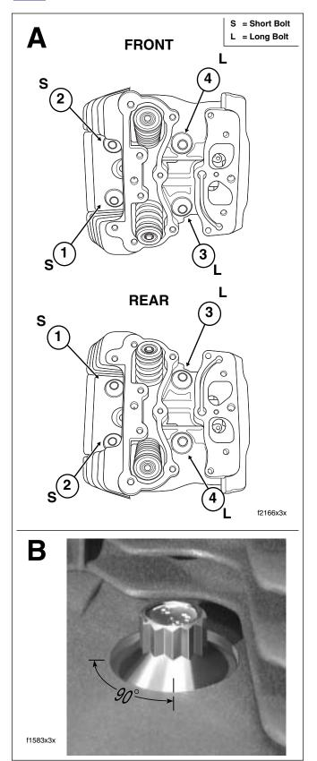
Figure 3-34. Cylinder Head Torque Sequence and Bolt Size
