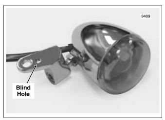
Figure 8-60. Front Left Turn Signal Lamps (FLHRS)
