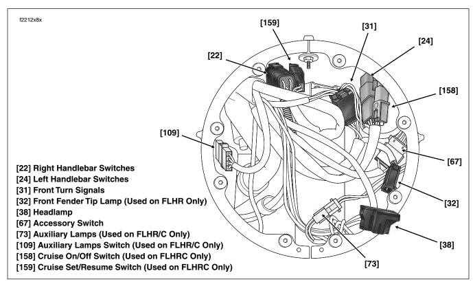
Figure 8-156. Headlamp Nacelle - Main Harness Connectors (FLHR/C/S)
