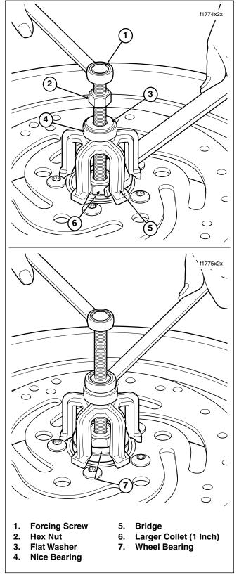
Figure 2-10. Remove Sealed Wheel Bearings
