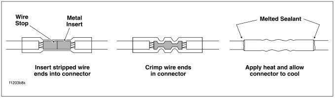
Figure B-40. Installing Sealed Butt Splice Connectors
