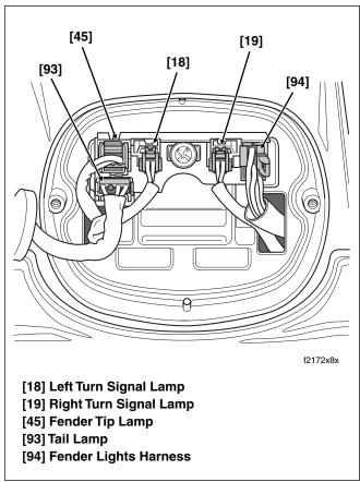
Figure B-50. Rear Fender Lights Assembly
