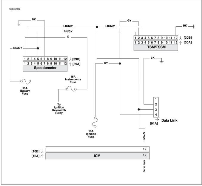
Figure 3-42. Serial Data Circuit: FLHR/S (Carbureted)
