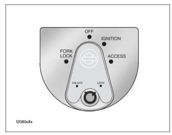
Figure 2-2. Ignition Switch (FLHX, FLHT/C/U, FLTR)
