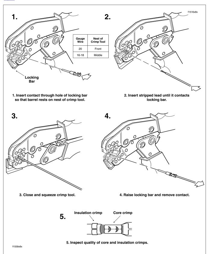
Figure 8-7. Deutsch Crimping Procedure
