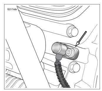
Figure 9-6. Remove Sensor Mount Socket Screw
