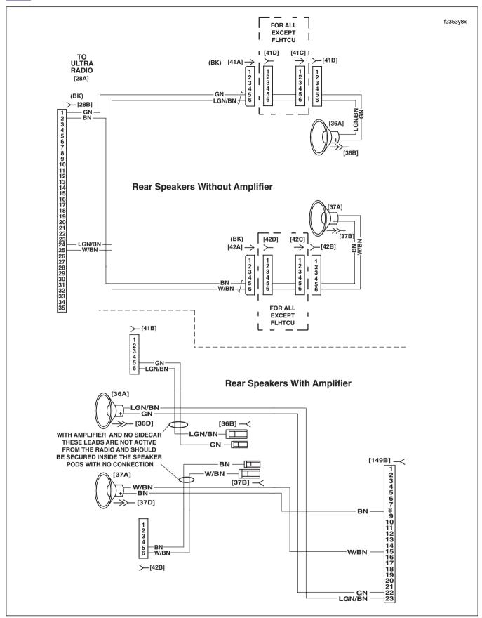
Figure 6-22. Rear Speaker Circuit
