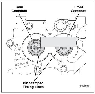
Figure 3-49. Verify Alignment of Timing Lines on Front and Rear Camshafts
