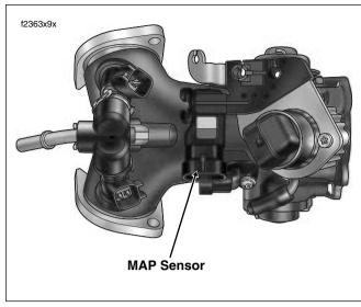
Figure 5-45. Induction Module (Top View)
