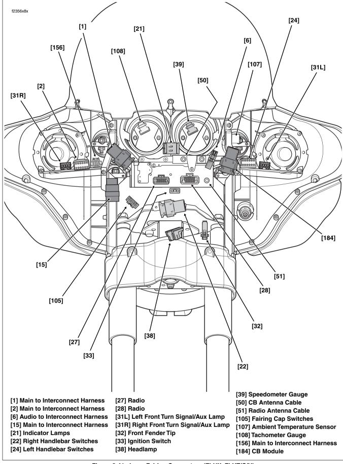
Figure 8-41. Inner Fairing Connectors (FLHX, FLHT/C/U)
