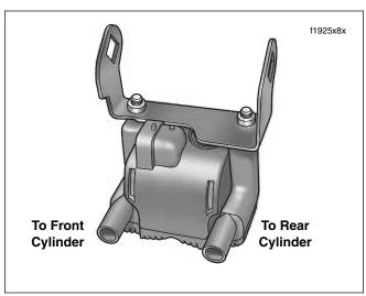
Figure 8-9. Install Bracket to Ignition Coil
