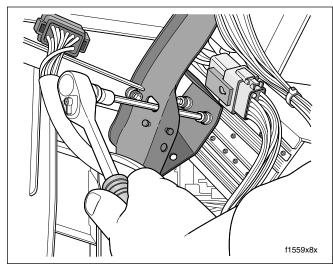
Figure 8-141. Release Radio from Fairing Brackets (FLHTC/U)
