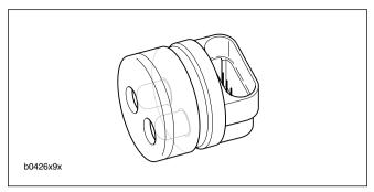
Figure 5-36. IAC Test Lamp (Part No. HD-41199-3)
