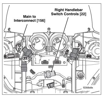
Figure 7-7. Outer Fairing Removed (FLHTC/U)
