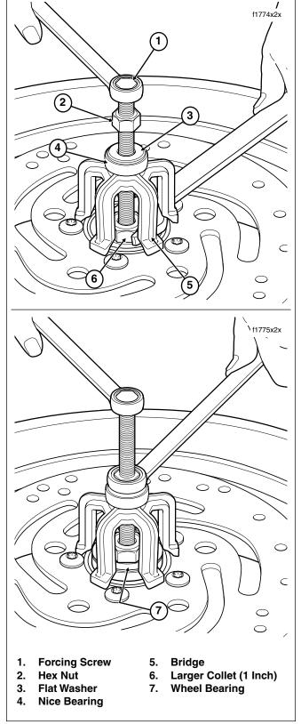
Figure 2-4. Remove Sealed Wheel Bearings
