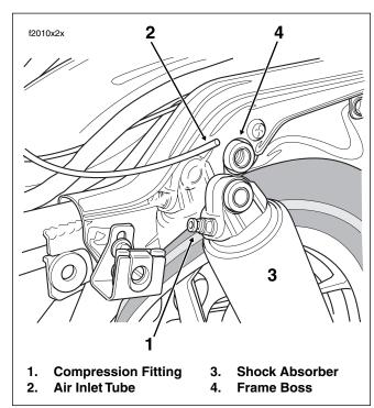
Figure 2-95. Remove Upper Shock Mounting Bolt (Left Side View)
