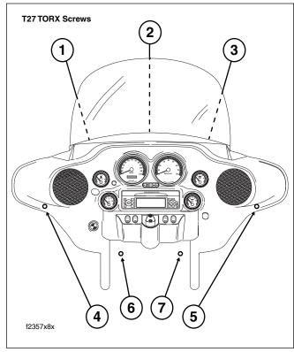
Figure 2-162. Outer Fairing TORX Screw Locations
