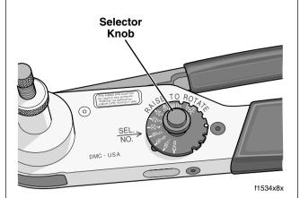
Turn adjusting screw as described in text. When contact is flush with bottom of depression in indentor cover, squeeze handles to center contact between indentor points.
