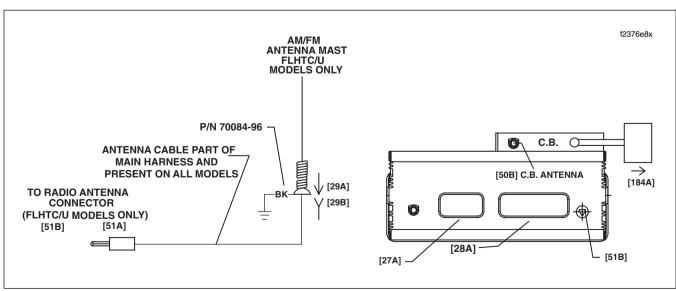
Figure 6-32. Radio Antenna Cable and Mast
