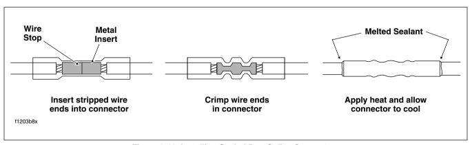
Figure 8-40. Installing Sealed Butt Splice Connectors
