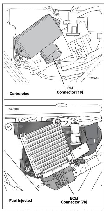
Figure 2-27. Electrical Bracket (Under Right Side Cover)
