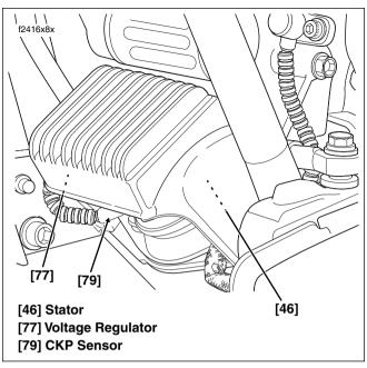
Figure 4-34. Voltage Regulator (Left Side View)
