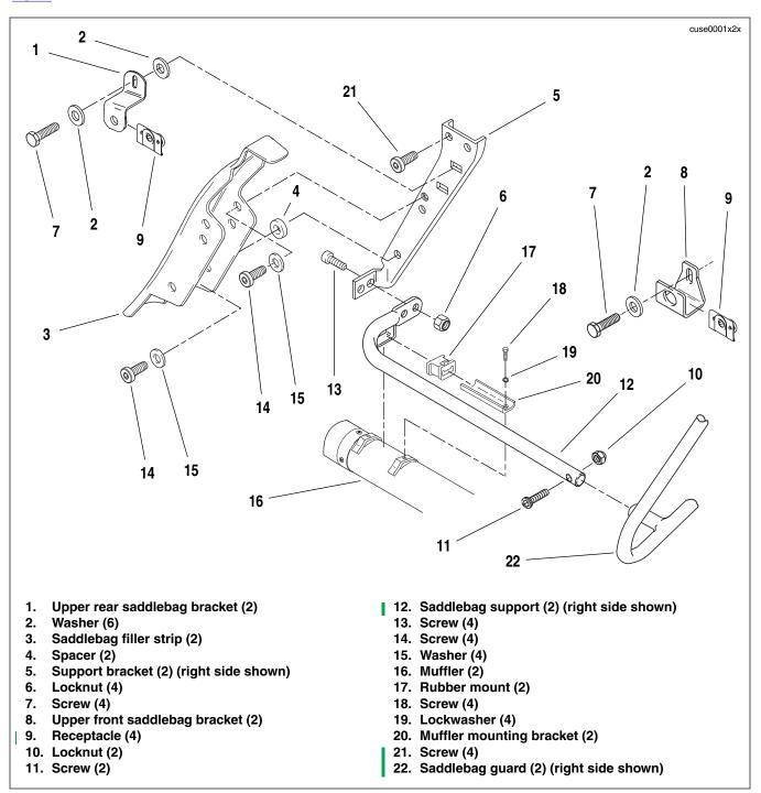
Figure 2-55. Saddlebag Support Components
