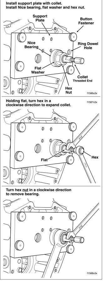
Figure 3-117. Remove Cam Needle Bearing
