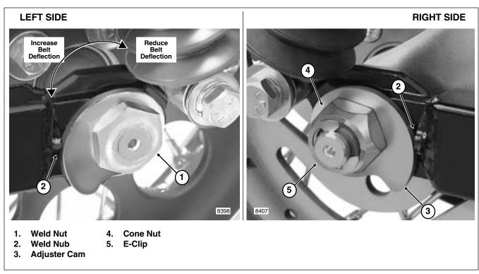
Figure 2-15. Move Rear Wheel Forward Until Adjuster Cams Just Contact Weld Nubs
