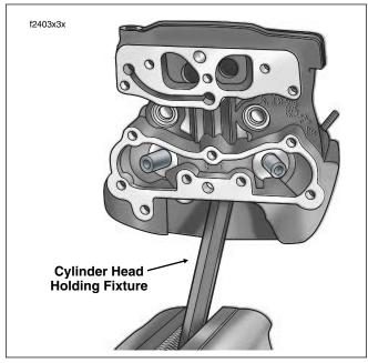
Figure 3-64. Install Cylinder Head Holding Fixture in Vise
