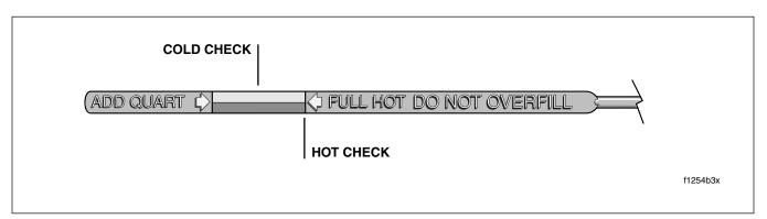
Figure 3-1. Engine Oil Dipstick
