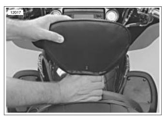
Figure 2-46. Removing Backrest
