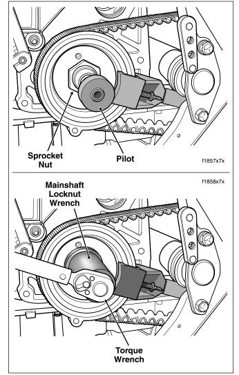
Figure 7-45. Install Mainshaft Locknut Pilot/Wrench and Torque Sprocket Nut
