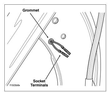
Figure 8-49. Pull Fender Tip Lamp Wires and Terminals
