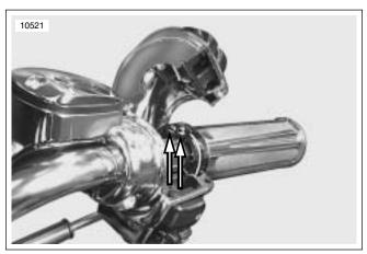
Figure 2-12. Throttle and Idle Cable Ferrules
