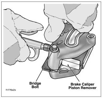
Figure 2-61. Direct Compressed Air Into Banjo Bolt Hole
