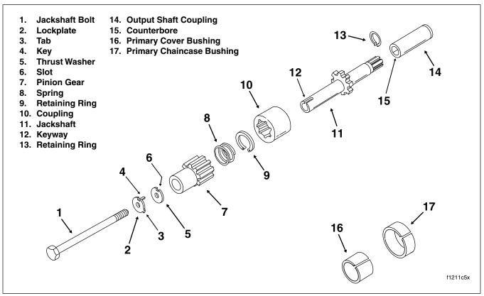
Figure 5-22. Starter Jackshaft Assembly
