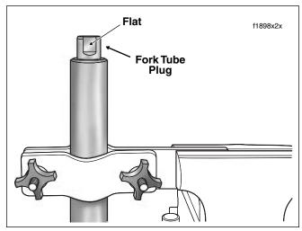
Figure 2-75. Install Fork Tube Into Fork Holder
