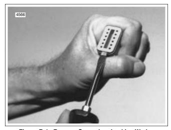
Figure B-1. Remove Secondary Locking Wedge
