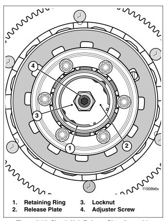
Figure 6-16. Clutch Hub Release Plate Assembly
