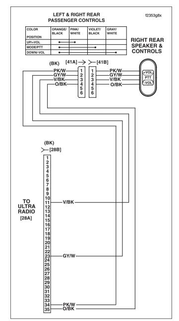
Figure 6-14. Passenger Audio/PTT Switch Circuit
