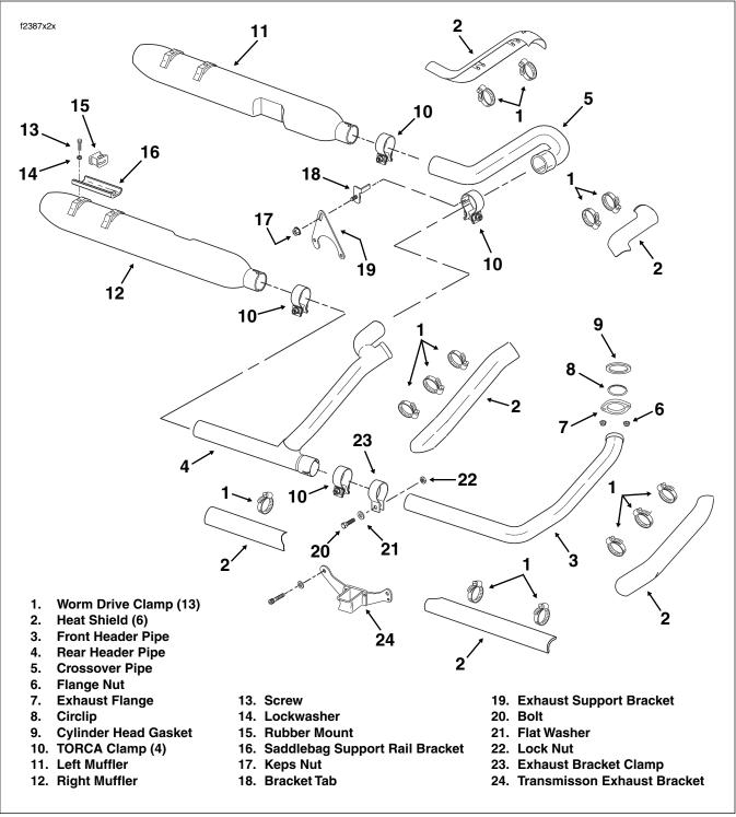
Figure 2-207. Disassemble/Assemble Exhaust System
