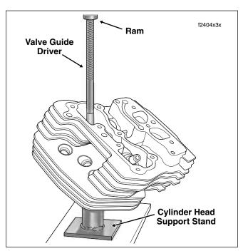
Figure 3-69. Remove Valve Guide
