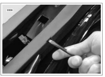
Figure 8-150. Release Catches From Cover
