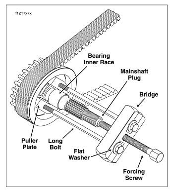
Figure 6-23. Pull Mainshaft Bearing Inner Race
