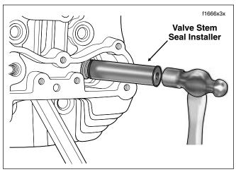
Figure 3-30. Tap Installer to Seat Valve Stem Seal
