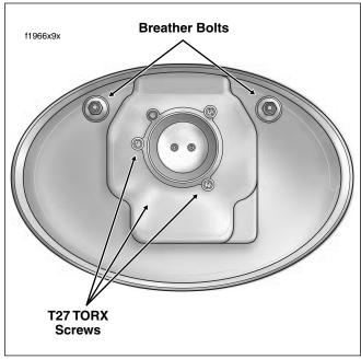
Figure 9-26. Install Backplate to Align Induction Module
