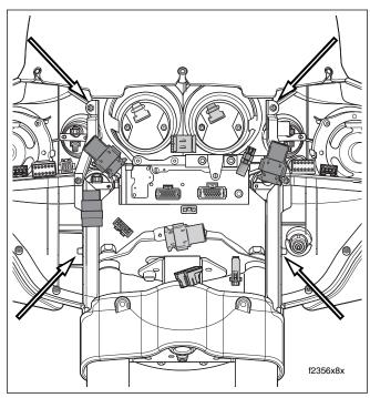
Figure 2-168. Remove Fairing Bracket Screws
