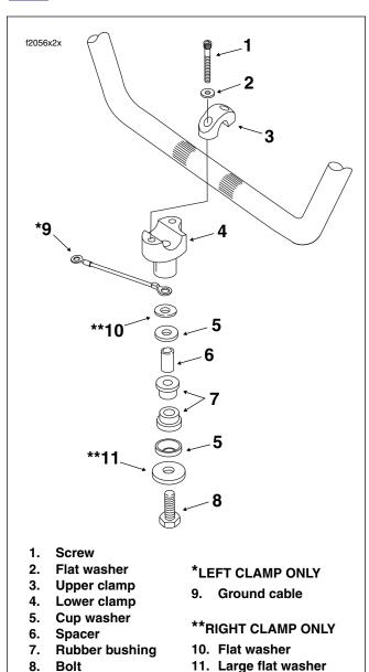
Figure 2-121. Handlebar Clamp Assemblies
