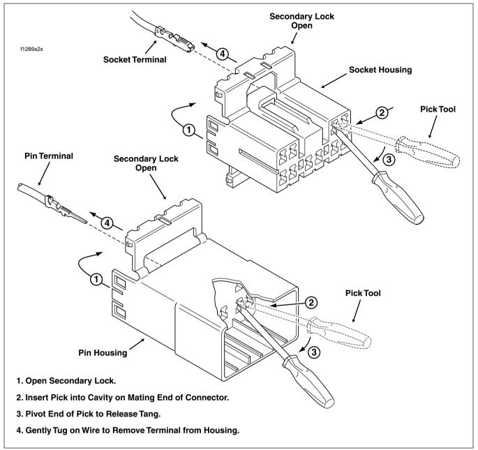
Figure 8-11. Release Tang and Back Out Terminals
