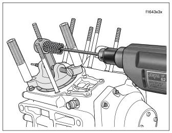
Figure 3-98. Hone Connecting Rod Bushing
