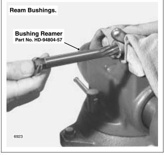
Figure 3-59. Replace Rocker Arm Bushings
