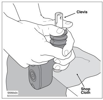
Figure 2-50. Compress Spring and Remove Retaining Ring
