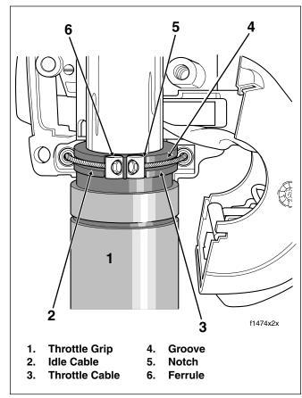
Figure 2-169. Install Throttle/Idle Cables
