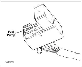
Figure 9-10. EFI Fuse Block
