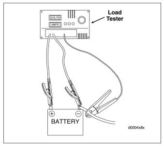
Figure 1-12. Check Current Draw (Ignition Switch On)
