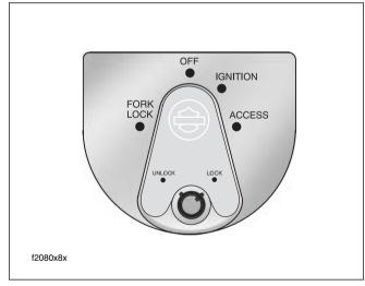
Figure 2-12. Ignition Switch (FLHX, FLHT/C/U, FLTR)
