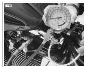
Figure 5-34. Fuel Pressure Gauge Installed (Typical)
