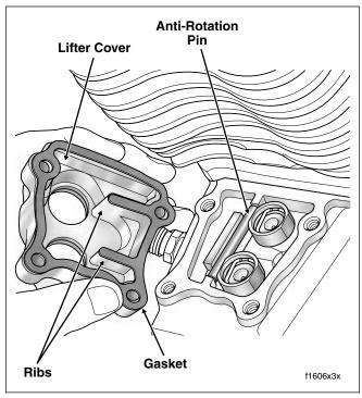
Figure 3-37. Install Lifters and Lock Position
