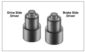
Figure 2-99. Rear Swingarm Bearing Installer (HD-45327)
