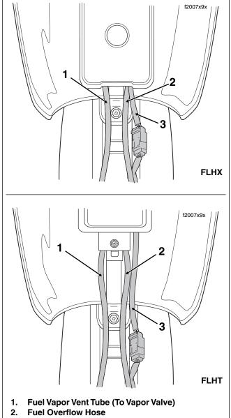
3. Fuel Tank Harness (To Fuel Level Sender)
