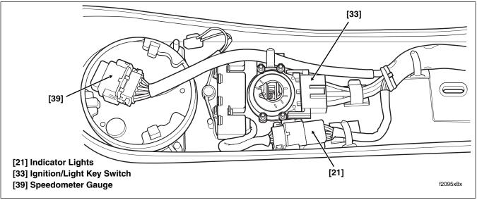
Figure B-56. Instrument Console Connectors (FLHR/C)
