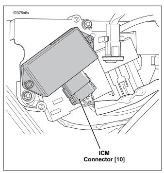
Figure 8-6. Electrical Bracket (Under Right Side Cover)
