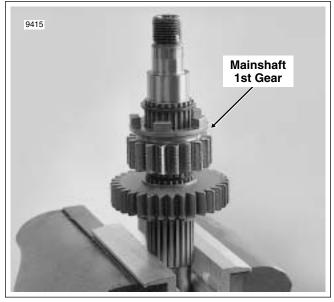
Figure D-5. Disassemble/Assemble Mainshaft
