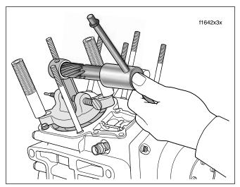
Figure 3-96. Ream Connecting Rod Bushing
