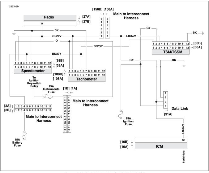
Figure 4-19. Serial Data Circuit (FLHX, FLHT/C)
