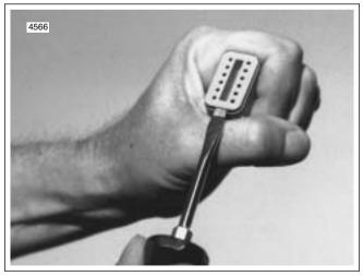
Figure 8-1. Remove Secondary Locking Wedge
