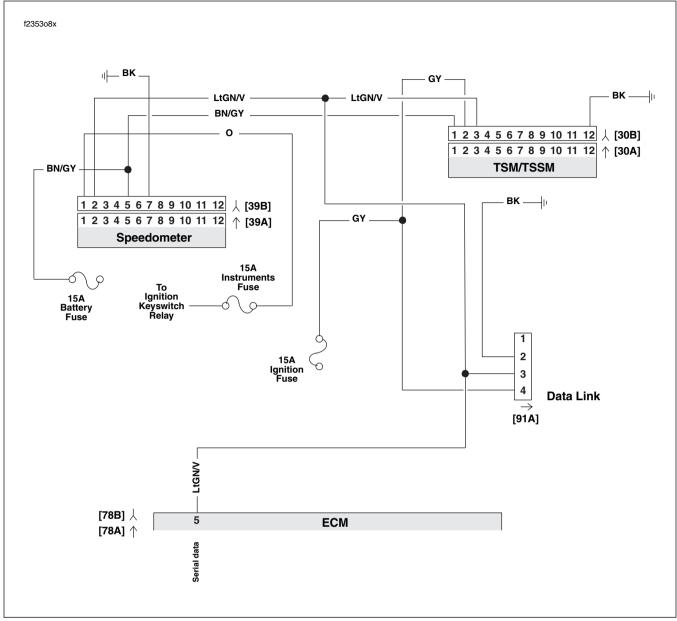
Figure 2-10. Diagnostic Check: FLHR/C/S (Fuel Injected)
