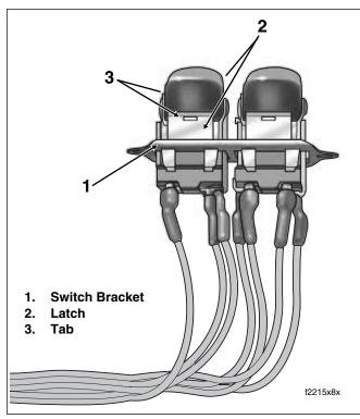
Figure 8-84. Bend Latches Outward to Release Tabs
