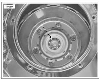
Figure 6-1. Clutch Release Bearing
