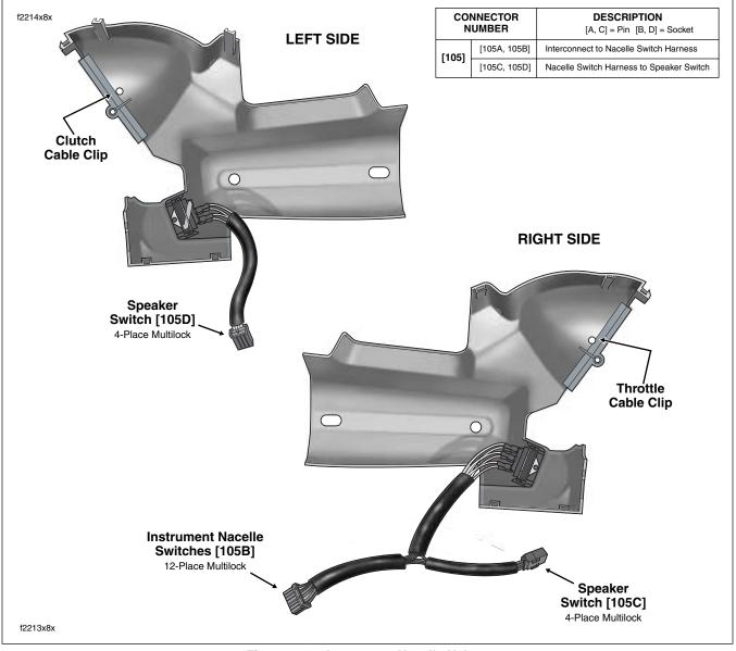
Figure 8-86. Instrument Nacelle Halves
