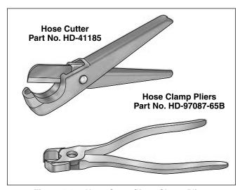
Figure 4-17. Hose Cutter/Hose Clamp Pliers
