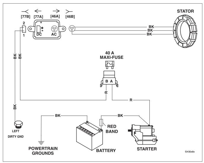
Figure 1-9. Charging System Circuit (Typical)
