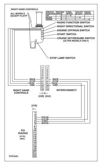
Figure 6-7. Handlebar Mode Switch Circuit
