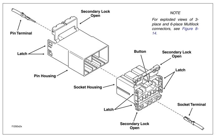
Figure 8-10. 10-Place Multilock Connector (Exploded View)
