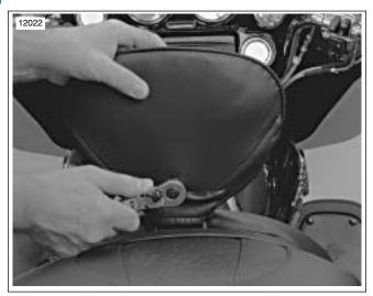
Figure 2-48. Adjusting Backrest Tilt Angle
