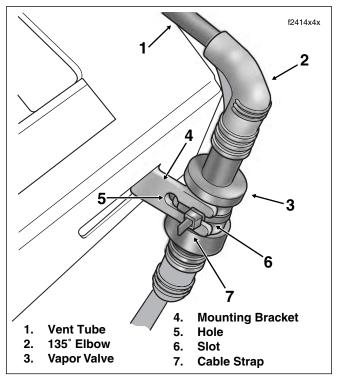
Figure 4-22. Vapor Valve Mounting Bracket (Left Side View)
