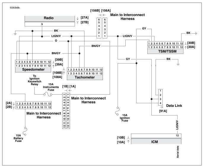
Figure 2-28. Serial Data Circuit: FLHX, FLHT/C (Carbureted)
