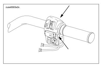
Figure 2-27. Right Handlebar Switch Housing Screws
