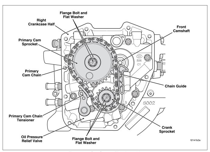
Figure 3-40. Cam Support Plate Assembly
