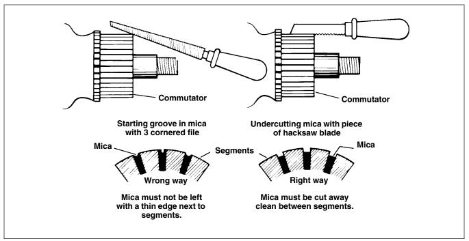
Figure 5-10. Undercutting the Mica Separators
