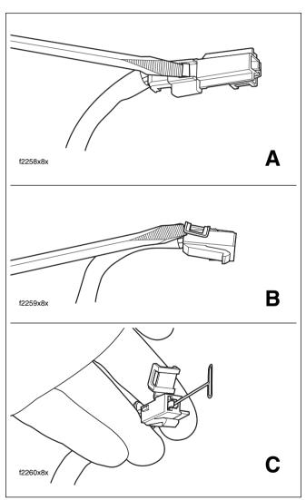
Figure 8-24. Remove Socket Terminal
