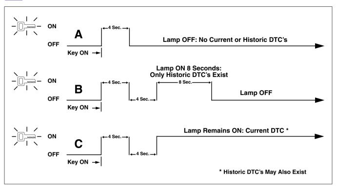
Figure 3-9. Security Lamp Operation
