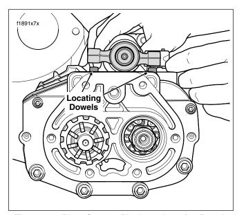
Figure 7-12. Place Support Blocks on Locating Dowels
