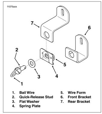
Figure 2-136. Saddlebag Quick-Release Fasteners
