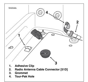
Figure 2-145. Feed Main Harness Thru Tour-Pak Hole
