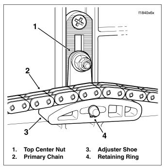
Figure 6-1. Primary Chain Tensioner Assembly
