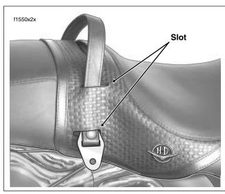
Figure 2-131. Route Passenger Seat Strap Through Slots in Seat - FLHRC
