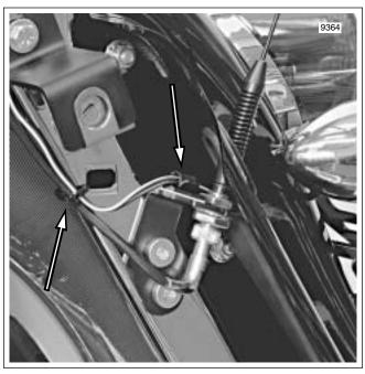
Figure 2-199. Capture Rear Facia Lamp Wires
