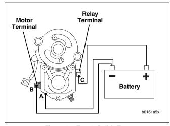
Figure 1-5. Test 1: Pull-In Test
