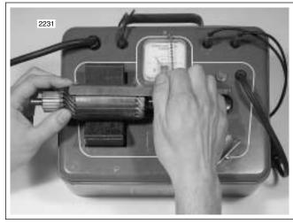
Figure 5-11. Shorted Armature Test Using Growler
