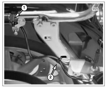
Figure 8-166. Capture Radio Antenna Cable (FLTR)
