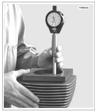
Figure 3-85. Measure for Out-of-Round and Taper
