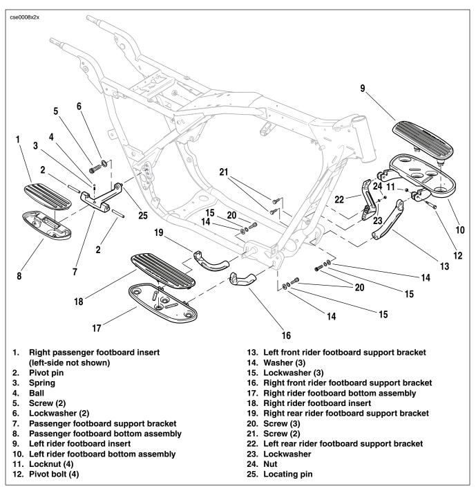
Figure 2-5. Rider and Passenger Footboard Components
