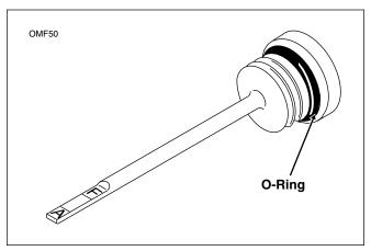
Figure 7-17. Transmission Lubricant Filler Plug/Dipstick
