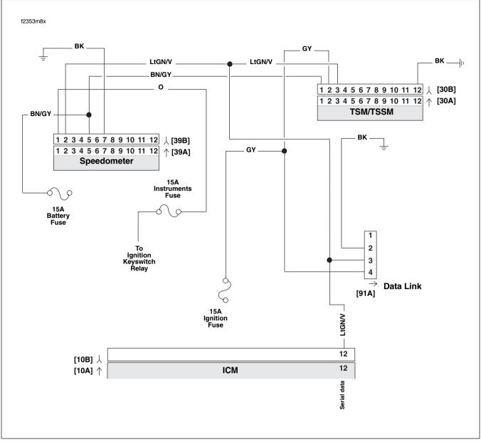
Figure 3-48. Serial Data Circuit: FLHR/S (Carbureted)
