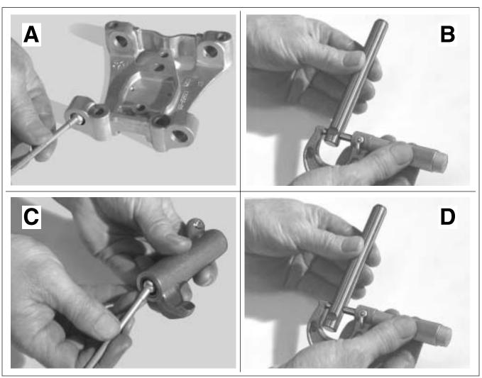
Figure 3-58. Measure Rocker Arm Assembly for Wear
