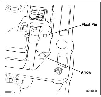
Figure 4-7. Remove Float Pin in Direction of Arrow
