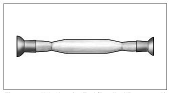
Figure 3-78. Valve Lapping Tool (Part No. HD-96550-36A)
