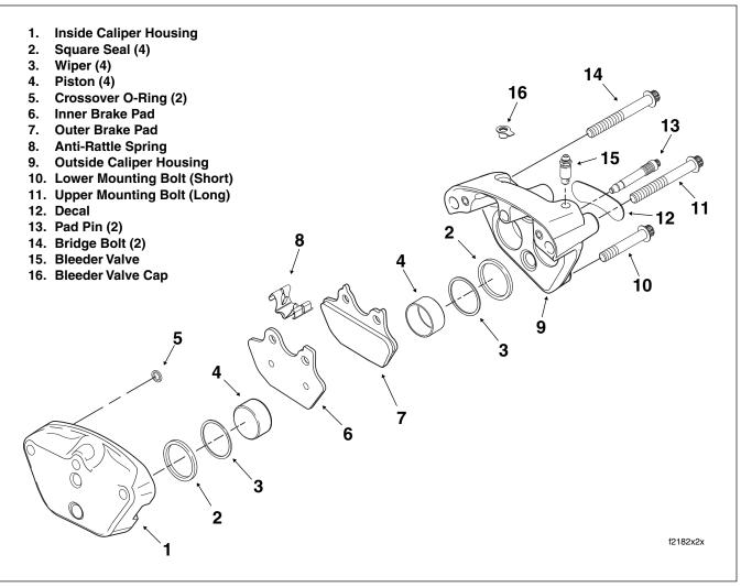
Figure 2-59. Front Brake Caliper Assembly (Left Side)
