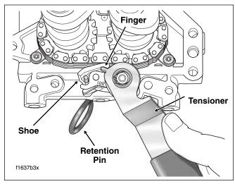
Figure 3-105. Retract Secondary Cam Chain Tensioner
