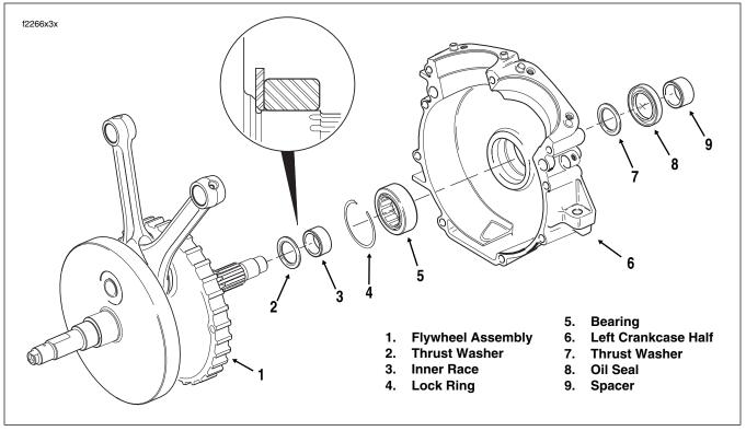
Figure 3-131. Sprocket Shaft Bearing Assembly
