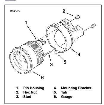
Figure 2-166. Voltmeter Gauge Assembly
