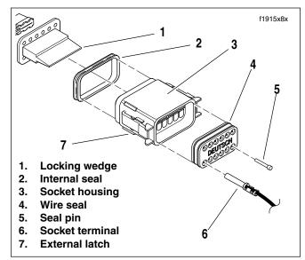
Figure 2-14. 12-place Deutsch Socket Side Connector
