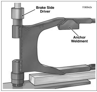
Figure 2-100. Press In Brake Side Bearing
