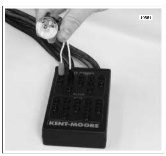
Figure 4-31. Ignition Coil Circuit Test
