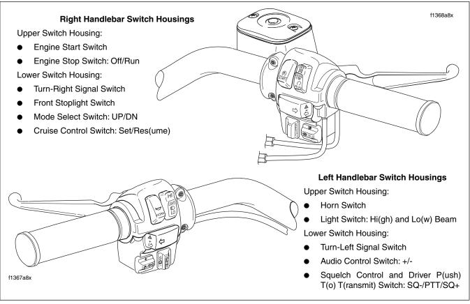
Figure 8-98. Ultra Handlebar Switch Assemblies
