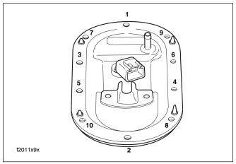
Figure 8-125. Canopy Torque Sequence (FLHR)
