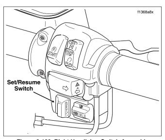
Figure 8-139. Right Handlebar Switch Assembly (FLTR, FLHTCU)
