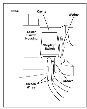
Figure 8-103. Install Stoplight Switch
