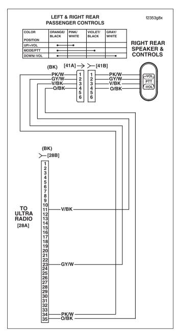
Figure 6-16. Passenger Audio/PTT Switch Circuit
