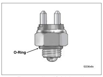
Figure 8-115. Neutral Switch Assembly
