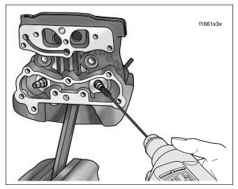
Figure 3-21. Hone Valve Guide Bore
