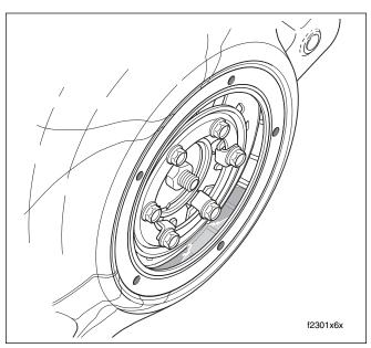
Figure 1-7. Add Primary Chaincase Lubricant
