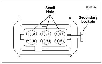
Figure 8-27. Mating End of Connector
