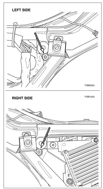
Figure 2-193. Fender Side Mounting Screws (T40 TORX)
