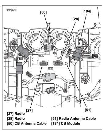
Figure 8-140. Radio Connections (FLHTC/U)
