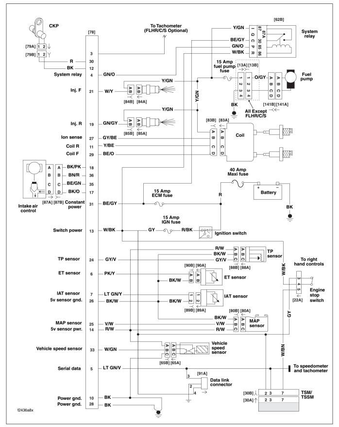
Figure 5-2. Simplified EFI System Circuit
