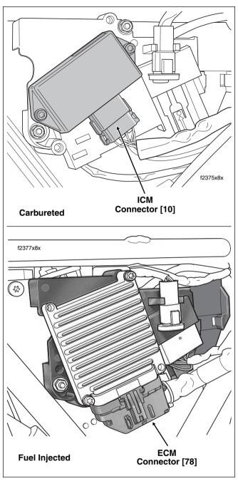
Figure 3-51. Electrical Bracket (Under Right Side Cover)
