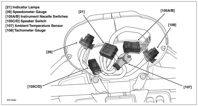
Figure 8-178. Instrument Nacelle (Bezel Removed)
