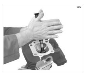
Figure 3-25. Oscillate Valve Lapping
