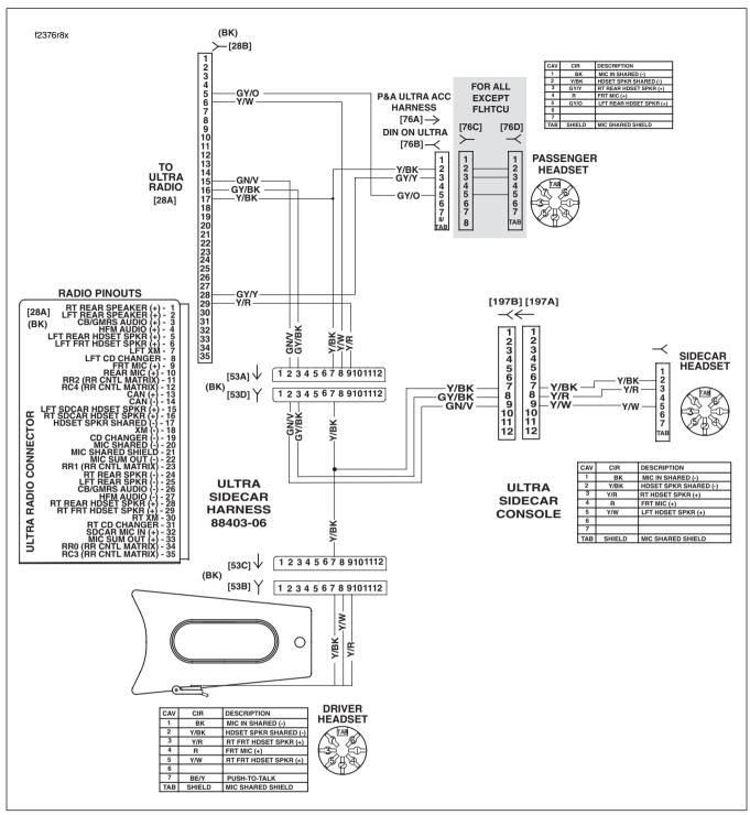
Figure 6-38. Headset Speaker Circuit
