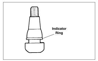
Figure 2-32. Snap-in Tubeless Tire Valves
