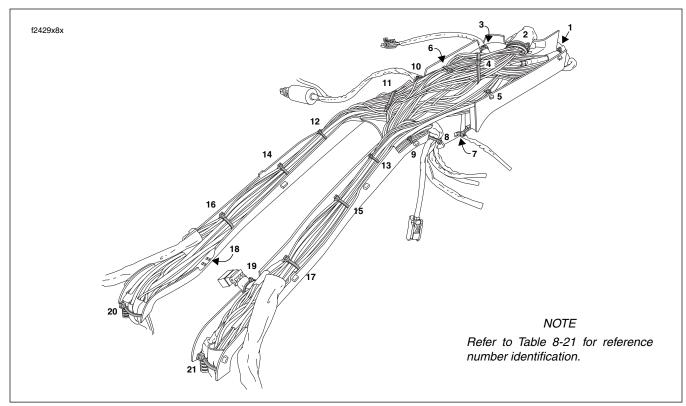
Figure 8-190. Wire Trough Cable Strap Locations (FLHTCU)
