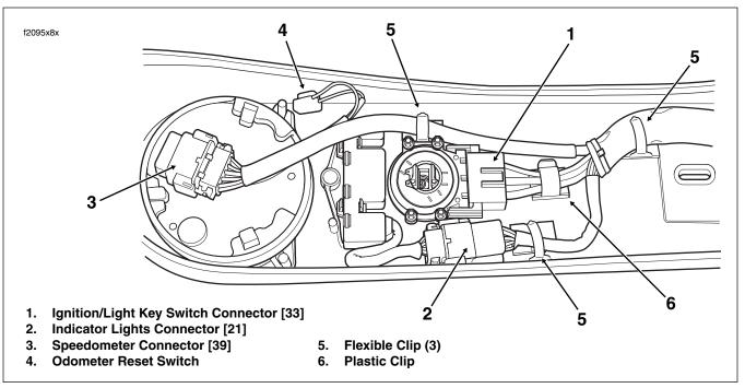
Figure 8-157. Instrument Console Assembly - Main Harness Connectors (FLHR/C)
