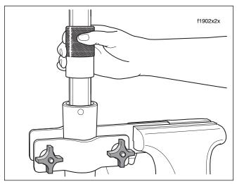
Figure 2-78. Install Fork Oil Seal
