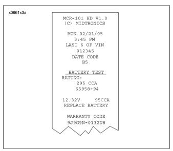
Figure 1-19. Battery Test Results-Printout
