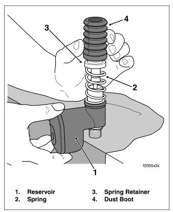
Figure 2-54. Install Spring, Spring Retainer and Dust Boot
