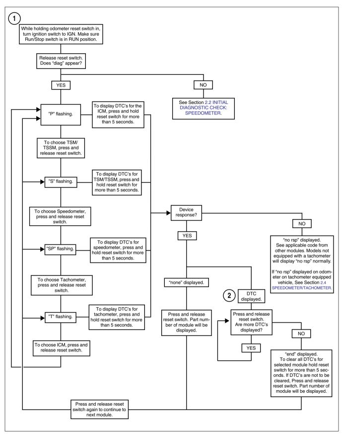
Figure 4-8. Speedometer Self Diagnostics
