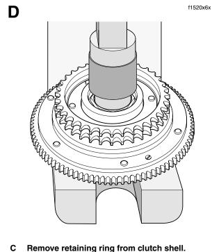
Figure 6-5. Remove Bearing from Clutch Shell
