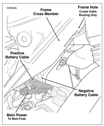
Figure 8-22. Battery Cable Routing (Right Side View)
