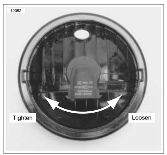
Figure 8-11. Replacing Bulb in Reflector
