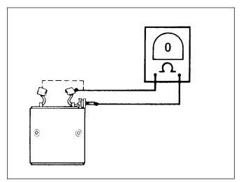
Figure 5-15. Open Field Test
