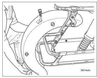
Figure 2-195. Carefully Roll Out Rear Fender
