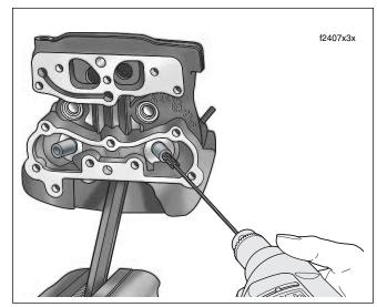
Figure 3-74. Hone Valve Guide Bore
