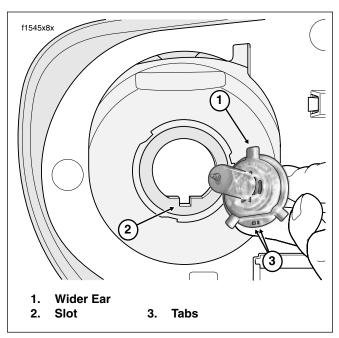
Figure 8-30. Install New Bulb in Bulb Housing
