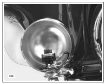
Figure 8-37. Auxiliary Lamp Housing
