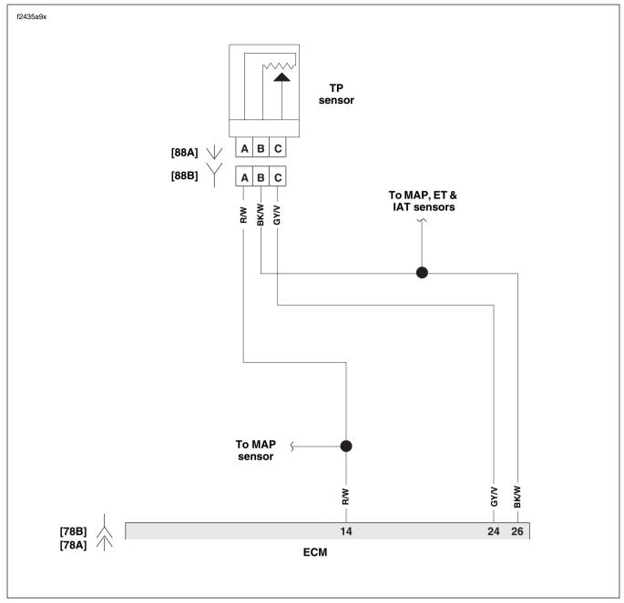
Figure 5-49. TP Sensor Circuit
