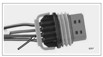
Figure B-16. Remove Wire Lock
