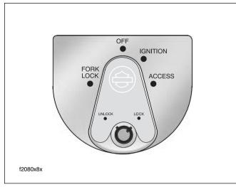
Figure 3-7. Ignition Switch (FLHX, FLHT/C/U, FLTR)
