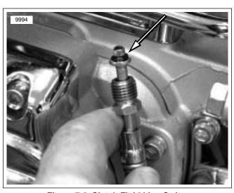
Figure 7-3. Clutch Fluid Line O-ring
