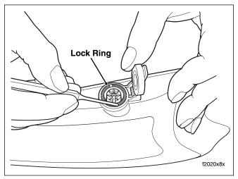
Figure 8-145. Remove Lock Ring from Receptacle
