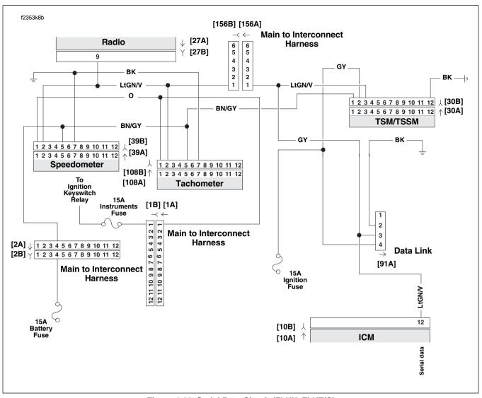
Figure 4-29. Serial Data Circuit (FLHX, FLHT/C)
