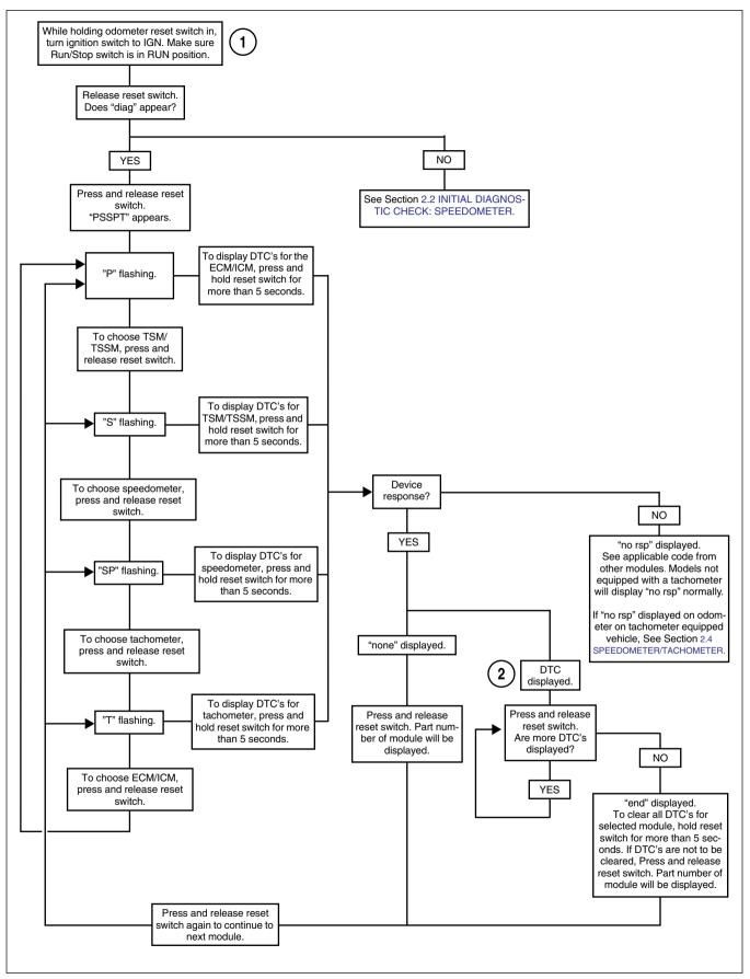
Figure 3-16. Initial Diagnostic Check
