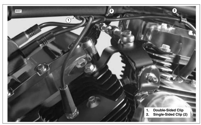
Figure 8-11. Spark Plug Cable Clips (Left Side View)
