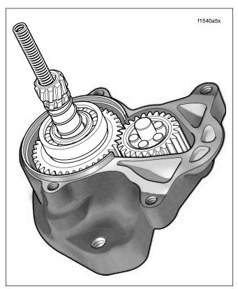
Figure 5-18. Drive Housing Assembly
