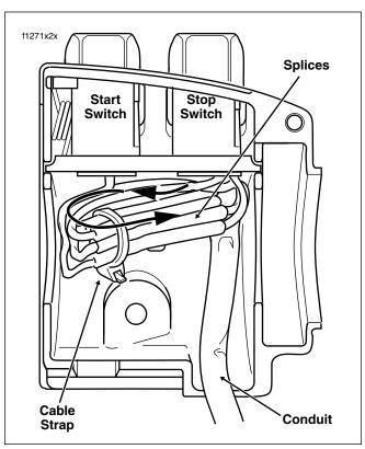
Figure 8-100. Upper Right Handlebar Switch Housing (With Splices)
