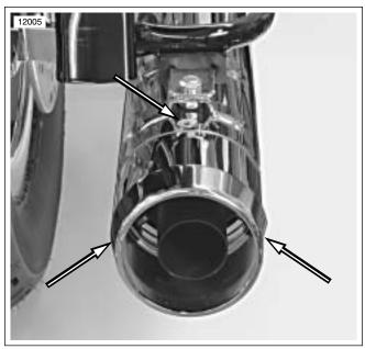
Figure 2-56. Muffler End Cap Fastener Locations
