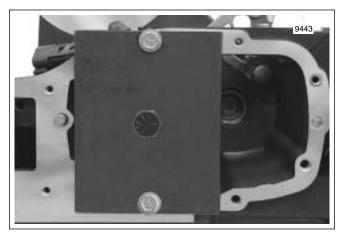
Figure 7-34. Main Drive Gear Bearing Installation (Right Side)
