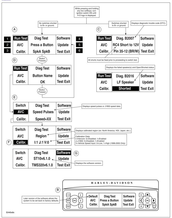
Figure 6-1. Radio Diagnostic Display
