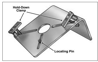
Figure 3-127. Flywheel Fixture (Part No. HD-44358)
