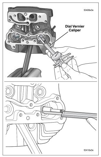
Figure 3-77. Measure Valve Stem Protrusion
