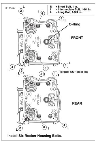
Figure 3-36. Rocker Housing Torque Sequence and Bolt Size
