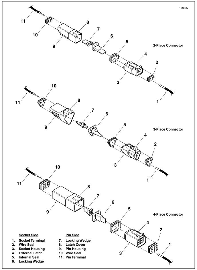
Figure 8-5. 2-Place, 3-Place and 4-Place Deutsch Connectors
