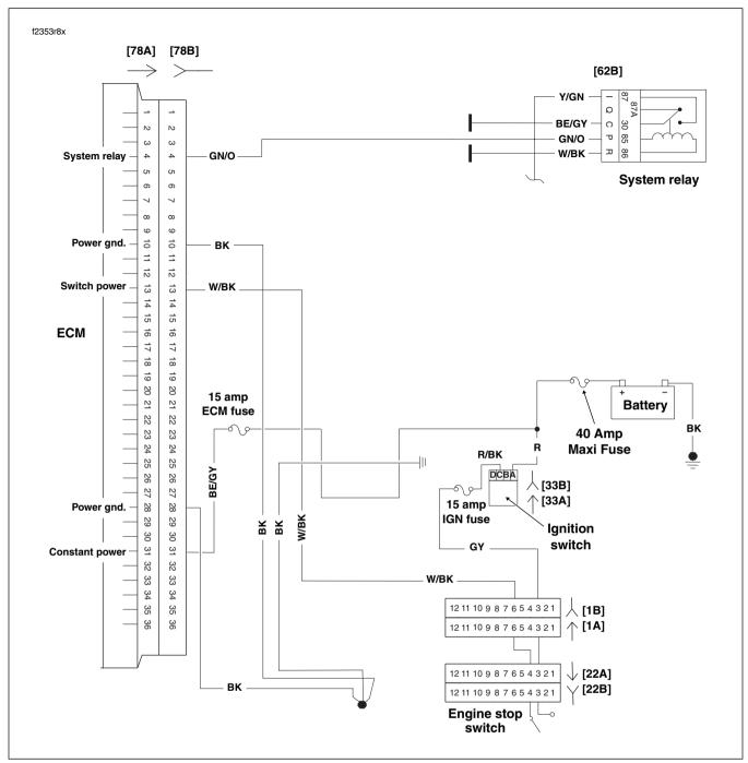
Figure 5-60. Battery Voltage Circuit (FLHX, FLHT/C/U, FLTR)
