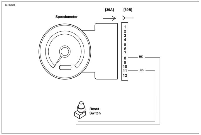
Figure 2-25. Reset Switch Circuit
