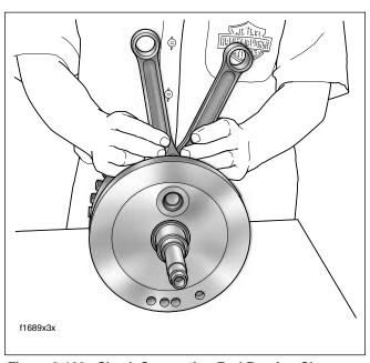
Figure 3-132. Check Connecting Rod Bearing Clearance
