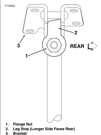
Figure 2-201. Leg Stop Orientation (Full Forward Position)
