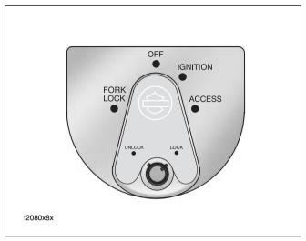
Figure 5-4. Ignition Switch (FLHX, FLHT/C/U, FLTR)
