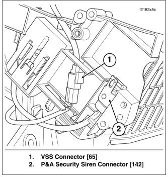
Figure 4-37. Electrical Bracket (Inboard Side)
