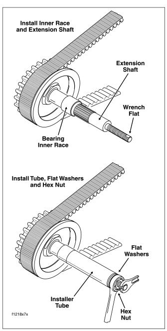
Figure 6-25. Press Bearing Inner Race onto Mainshaft
