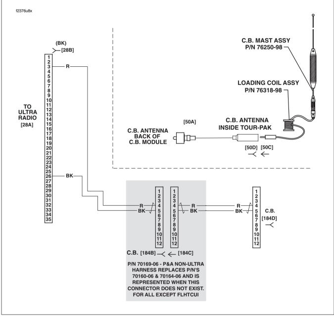
Figure 6-35. CB Receiver Audio Circuit
