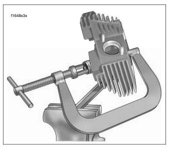
Figure 3-11. Compress Valve Springs
