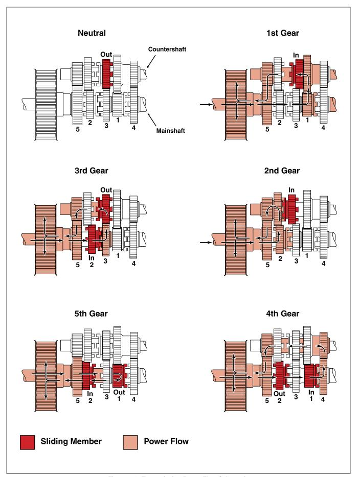
Figure 7-1. Transmission Power Flow Schematic
