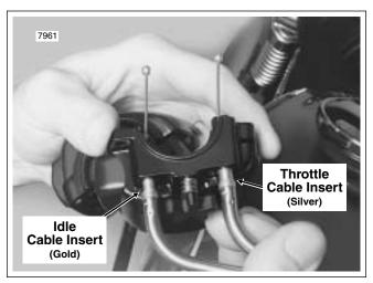
Figure 2-109. Install Throttle/Idle Cables in Lower Switch Housing
