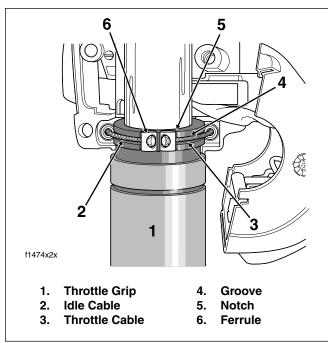
Figure 1-18. Remove Throttle/Idle Cables
