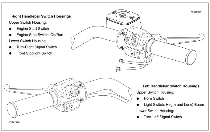
Figure 8-95. Road King Handlebar Switch Assemblies
