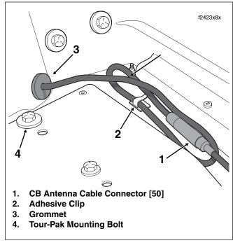
Figure 8-188. Disconnect CB Antenna Cable Connector
