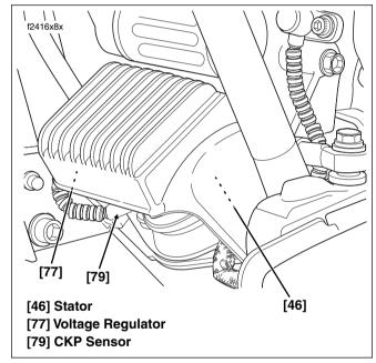
Figure 5-54. Voltage Regulator (Left Side View)
