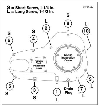
Figure 6-32. Primary Chaincase Cover Torque Sequence and Screw Size
