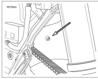
Figure 2-191. Rear Fender Front Screw (T40 TORX)
