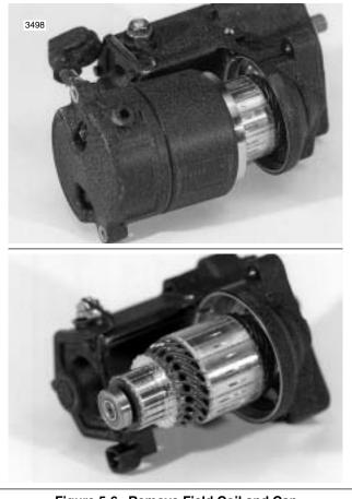
Figure 5-6. Remove Field Coil and Cap
