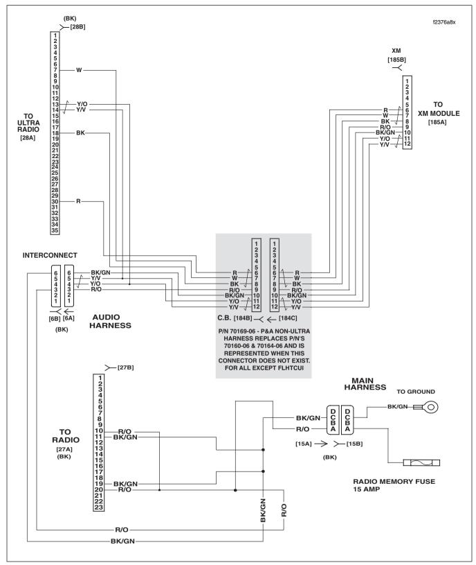
Figure 6-41. XM Circuit
