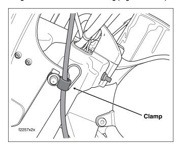
Figure 2-117. Clutch Cable Routing - FLHR/C (Left Side View)
