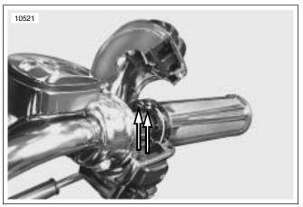
Figure 2-28. Throttle and Idle Cable Ferrules
