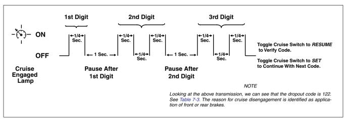
Figure 7-5. Cruise Engaged Lamp Dropout Code Timing Diagram
