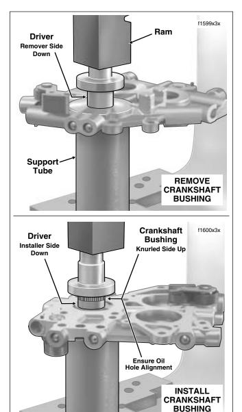
Figure 3-102. Remove/Install Crankshaft Bushing in Cam Support Plate
