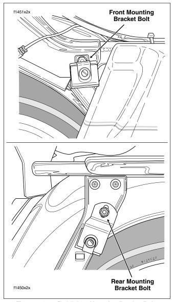
Figure 2-137. Saddlebag Mounting Bracket Bolts (Right Side View)
