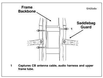
Figure 8-195. Capture CB Antenna Cable (FLHTCU)
