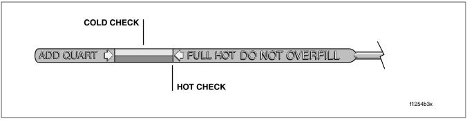
Figure 3-19. Engine Oil Dipstick
