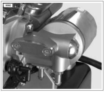
Figure 3-50. Oil Filter Mount (engine removed from frame)
