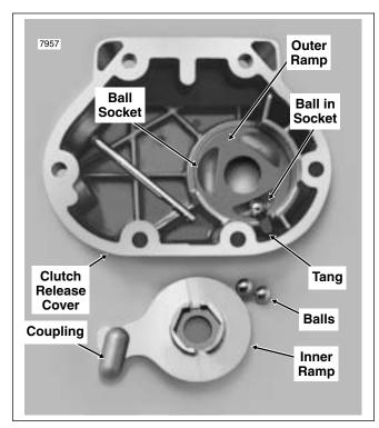
Figure 7-15. Install Outer Ramp and Balls
