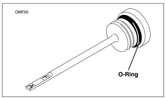
Figure 1-12. Transmission Lubricant Filler Plug/Dipstick
