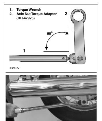
Figure 2-14. Install Tool Perpendicular to Torque Wrench
