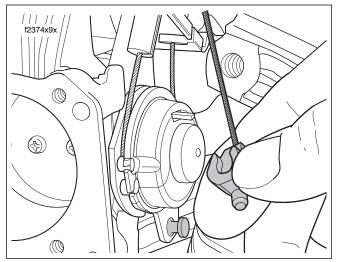
Figure 8-134. Remove End Fitting From Wheel Pin
