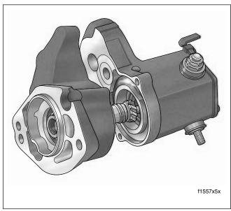
Figure 5-17. Remove Drive Housing
