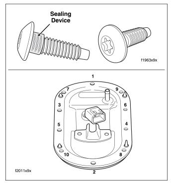
Figure 9-16. Canopy Sealing Screws and Torque Sequence
