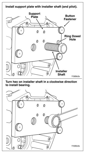
Figure 3-118. Install Cam Needle Bearing
