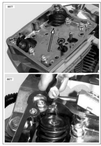
Figure 3-4. Valve Spring to Rocker Housing Clearance
