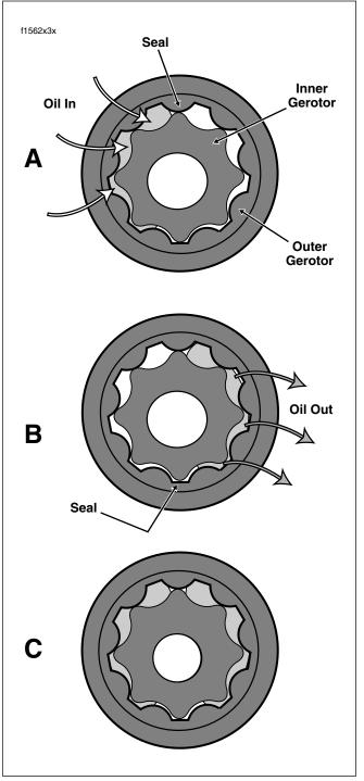
Figure 3-9. Gerotor Operation
