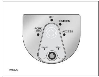
Figure 3-15. Ignition Switch (FLHX, FLHT/C/U, FLTR)
