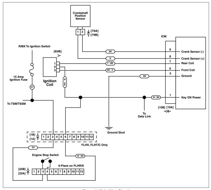
Figure 4-17. Ignition Circuit
