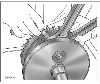
Figure 3-133. Check Connecting Rod Side Play
