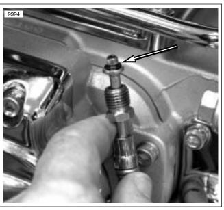
Figure 2-36. Clutch Fluid Line O-ring
