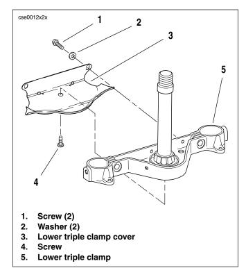
Figure 2-8. Lower Triple Clamp Cover
