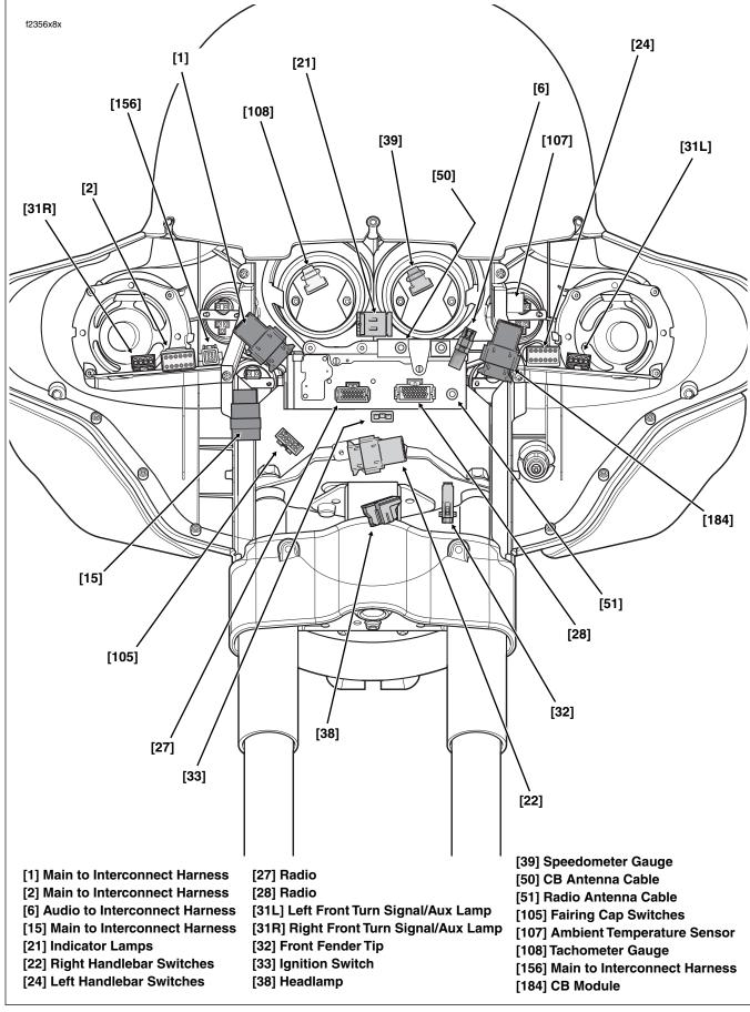
Figure B-41. Inner Fairing Connectors (FLHX, FLHT/C/U)
