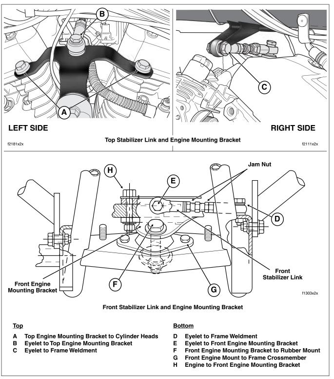
Figure 1-26. Engine Mounting Bracket Bolts
