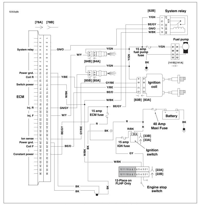
Figure 5-30. System Relay Circuit (FLHR/C/S)
