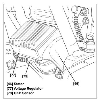
Figure B-51. Voltage Regulator (Left Side View)
