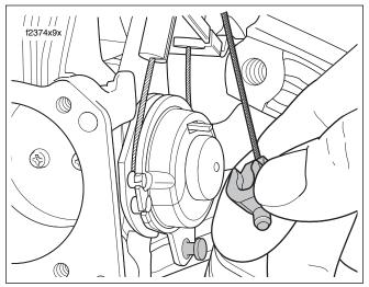
Figure 9-24. Remove End Fitting From Wheel Pin
