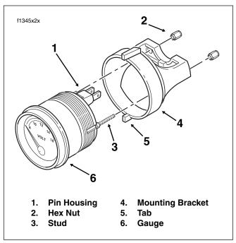
Figure 8-116. Voltmeter Gauge Assembly
