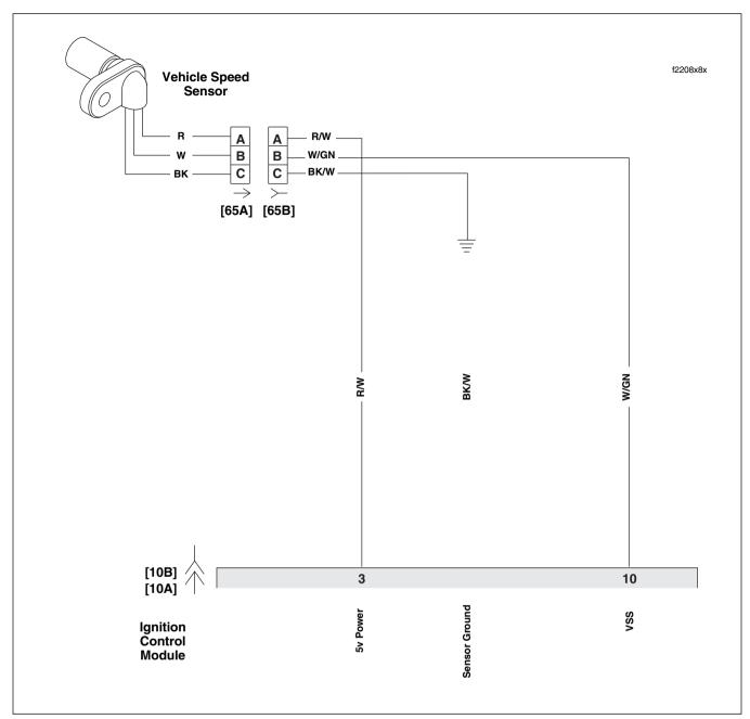
Figure 4-38. Vehicle Speed Sensor Circuit
