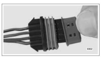
Figure 8-17. Remove Terminal Lock
