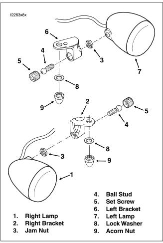
Figure 8-59. Front Turn Signal Lamp Brackets (FLHRS)
