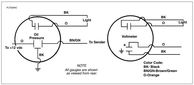
Figure 2-18. Connections for Gauges
