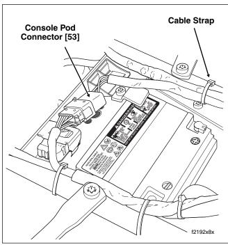
Figure 8-143. Disconnect Console Pod Connector
