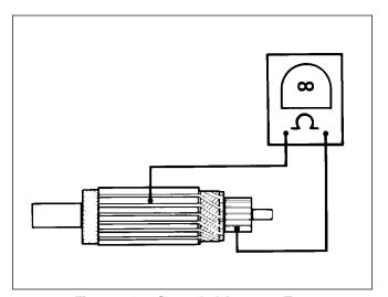
Figure 5-12. Grounded Armature Test
