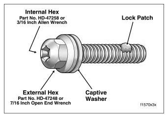
Figure 3-20. Rocker Cover Bolt (1-1/4 Inch)
