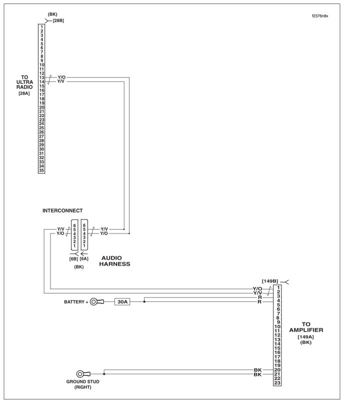
Figure 6-30. High Output Amplifier Circuit
