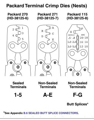
Figure B-36. Packard Terminal Crimp Tools
