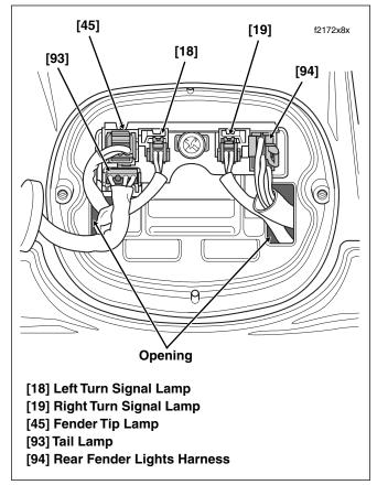
Figure 8-41. Rear Fender Lights Assembly
