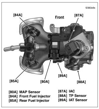
Figure 8-163. Induction Module Assembly (Top View)
