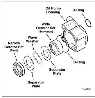
Figure 3-119. Oil Pump Assembly
