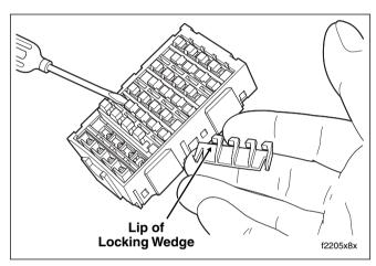
Figure 8-21. Remove Secondary Locks From Fuse Block
