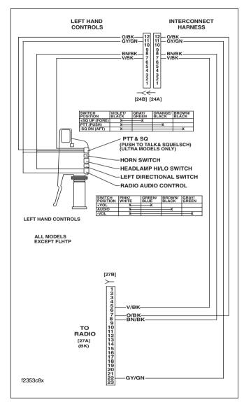
Figure 6-5. Handlebar PTT/Squelch Switch Circuit
