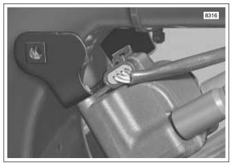
Figure 8-8. Remove Ignition Coil Bracket From Vehicle
