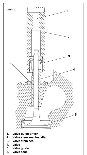
Figure 3-31. Using Arbor Press to Install Valve Stem Seal
