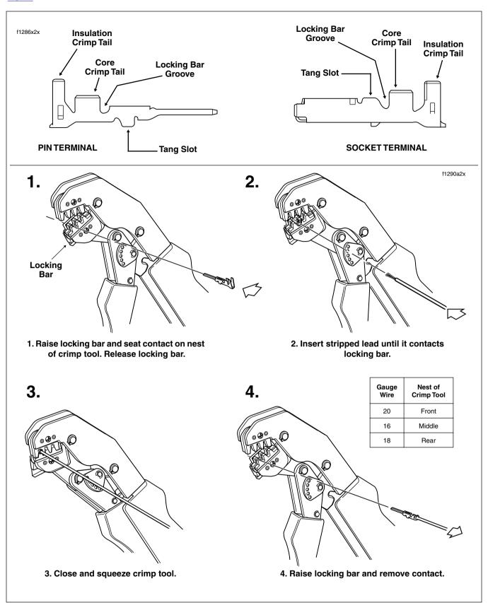
Figure 8-15. Multilock Crimping Procedure
