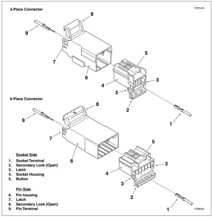
Figure B-14. 3-Place and 6-Place Multilock Connectors
