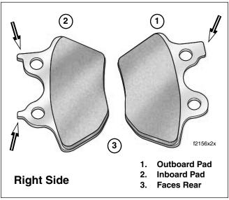
Figure 2-66. Rear Brake Pad Locations
