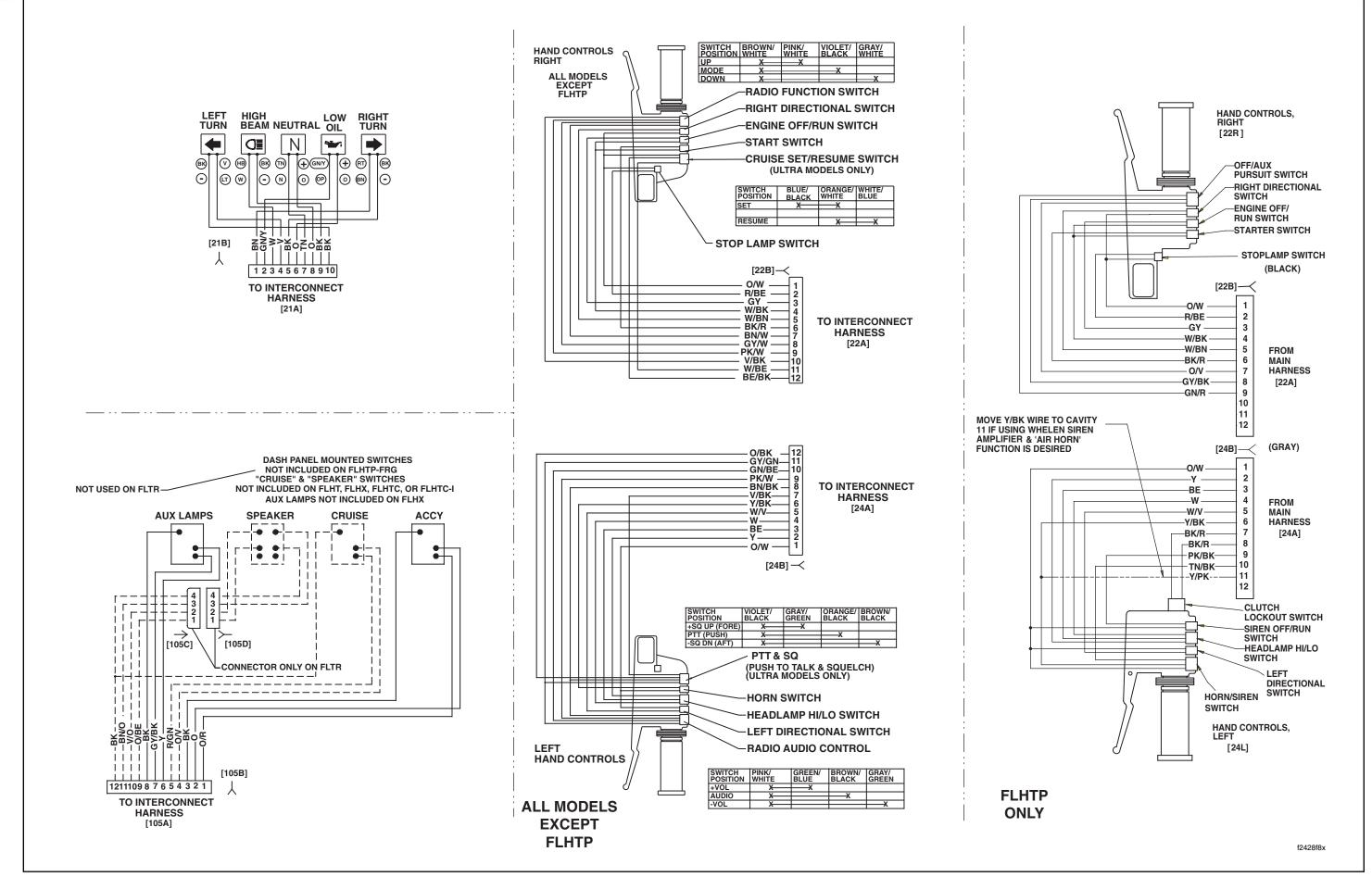
2006 FLHX, FLHT, FLHTC, FLHTCU and FLTR, DOMESTIC and INTERNATIONAL Models, Handlebar Switches, Indicator Lamps and Fairing Cap/Instrument Nacelle Switches
