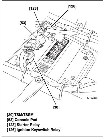
Figure B-52. Electrical Connectors/Relays (Under Seat)
