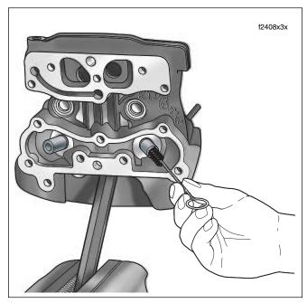
Figure 3-76. Scrub Valve Guide Bore
