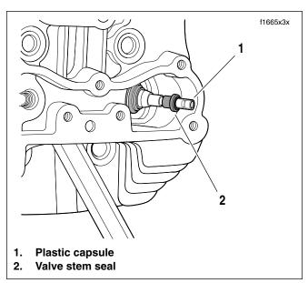
Figure 3-28. Install Valve Stem Seal
